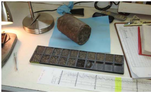
Drill core and drill chip logging from site characterization at the Mississippi Test Site. (Courtesy of Southern Company and Advanced Resources International)
