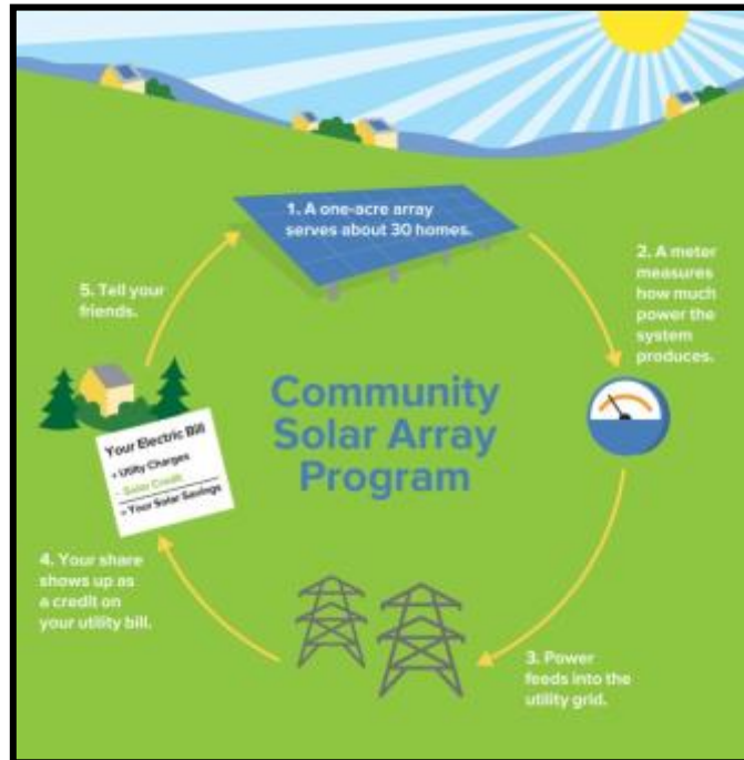
FIGURE 11. HOW COMMUNITY SOLAR ARRAYS (GARDENS) WORK
