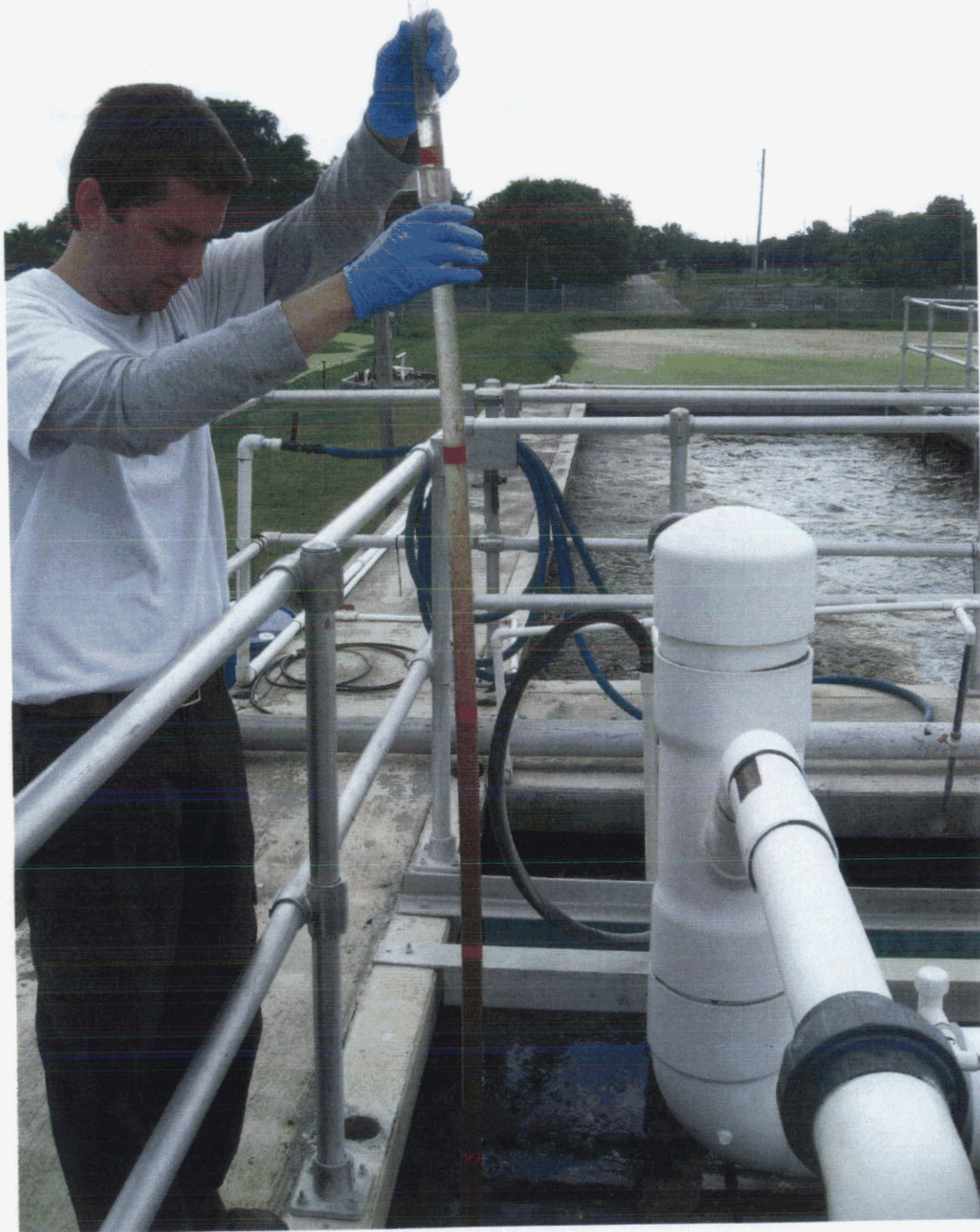
Photo above of the sludge blanket in the northern clarifier. Total height was 8'.
