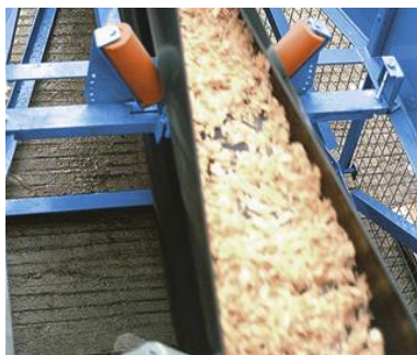
Material loading area: The conveyor belt is open and is loaded like a conventional belt conveyor.
