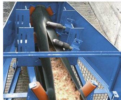
Belt closing section: Special devices close the conveyor carrying the conveyed material.
