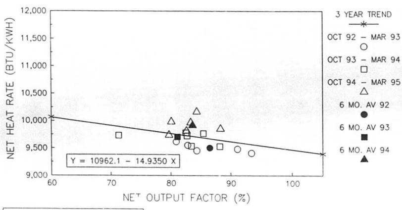
TARGET NET HEAT RATE: 9596 TARGET NET OUTPUT FACTOR: 91.5 ORIGIONAL SHEET NO. 7.401.95E PAGE 31 OF 35
