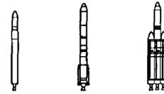
The Delta IV family of Medium, Medium-Plus and Heavy launch vehicles can lift payloads ranging from 9,285 pounds (4,210 kilograms) to 28,950 pounds (13,130 kilograms) to geosynchronous transfer orbit. The rockets are designed to meet the needs of the commercial and U.S. government launch markets for low-cost, assured access to space. On November 20, 2002, Boeing successfully launched its first Delta IV rocket, placing a Eutelsat commercial communications satellite into orbit.
