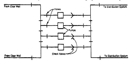
Figure 4.1 Simple Arrangement of Suction and Discharge Piping for Four Pumps
