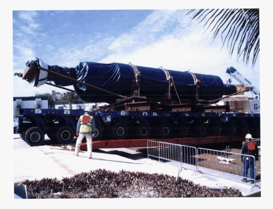
Docket No. 100009-EI Unloading the Main Generator Rotor at St. Lucie Exhibit TOJ-17, Page 1 of 1
