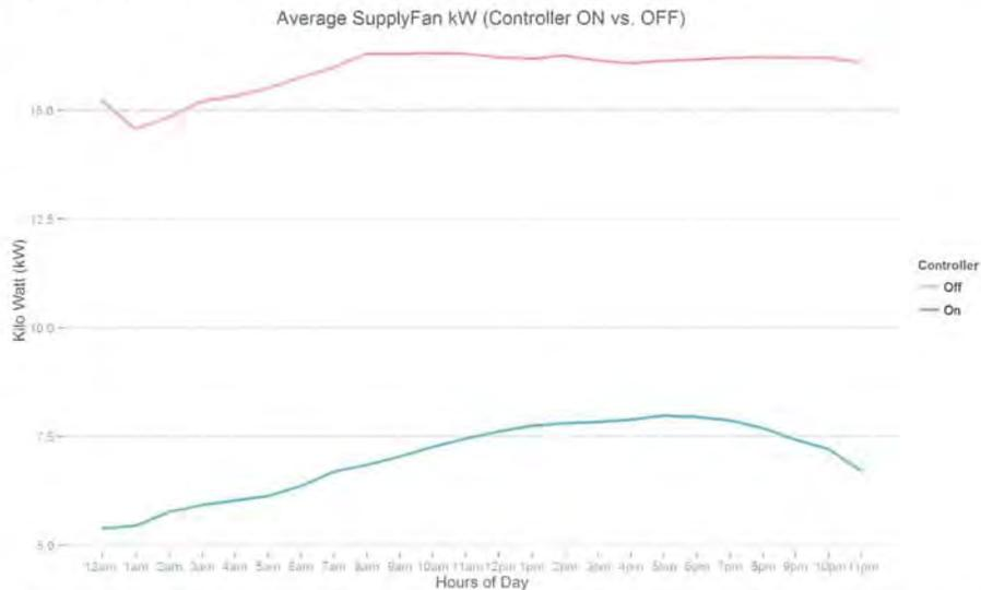
Figure 141: Figure above illustrates that there is a significant reduction in supply fan kWh draw when the controller is ON versus when it is OFF. The kWh draw follows a similar trend throughout the day. This indicates that both control strategies are reacting to the outside temperature and super market occupancy.
