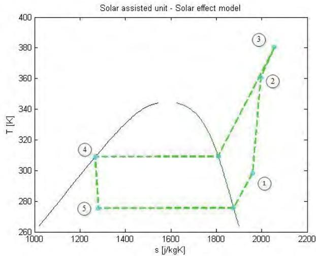
**Figure 23: VCC T-s diagram - (CASE II)**
