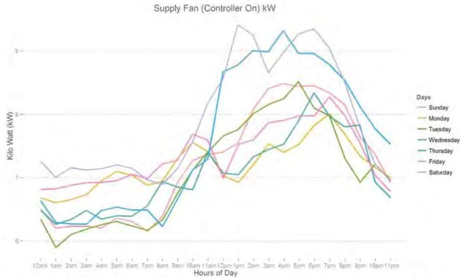
Figure 114: The figure above illustrates the average kWh draw of the supply fan when the controller is ON for each hour of the day and each day of the week. This is helpful in understanding the operation of the unit throughout the days of the week. It is clear that as the temperature increases throughout the day, so will the kWh draw.
