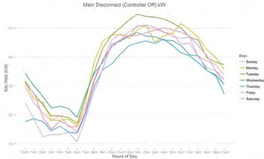
Figure 37: The figure above illustrates the average kWh draw of the main disconnect when the controller is OFF for each hour of the day and each day of the week. This is helpful in understanding the operation of the unit throughout the days of the week. It is clear that as the temperature increases throughout the day, so will the kWh draw.
