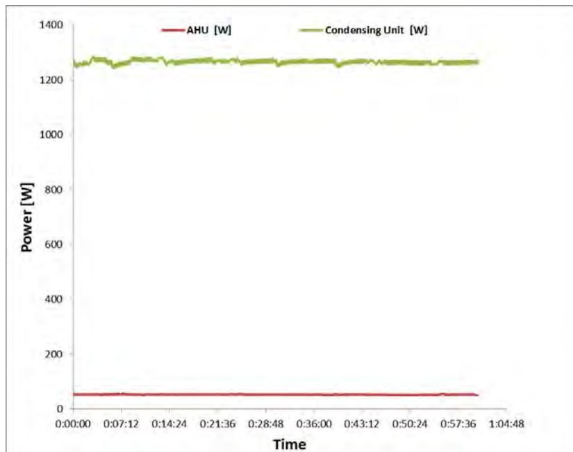
Figure 9: Bypass test AHU and condensing unit electric power consumption
