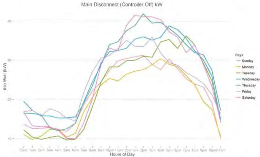
Figure 13: The figure above illustrates the average kWh draw of the main A/C unit when the controller is OFF for each hour of the day and each day of the week. This is helpful in understanding the operation of the unit throughout the days of the week. It is clear that as the temperature increases throughout the day, so will the kWh draw.
