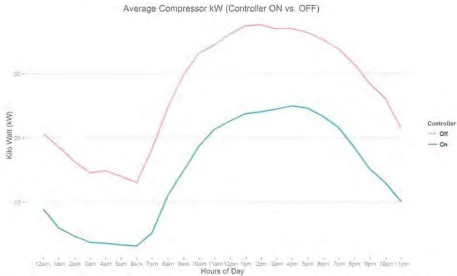
Figure 65: The figure above that there is a significant reduction in compressor kWh drawn when the controller is ON versus when it is OFF. The kWh draw follows a similar trend throughout the day. This indicates that both control strategies are reacting to the outside temperature and super market occupancy.
