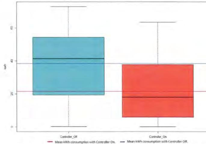
Figure 33: The Box Plot of the Compressor kWh and the Controller Status.
