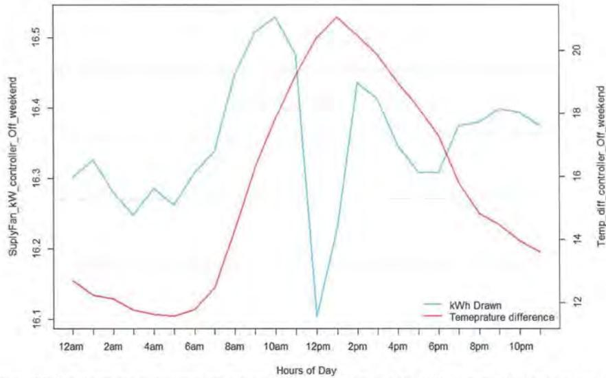
Figure 122: The figure above illustrates the relationship between the supply fan kWh draw and the indoor and outdoor temperature difference when the controller is OFF for the weekend hours (Saturday and Sunday). As it can be seen, as the temperature difference between indoor and outdoor temperature increased so does the kW consumption of the main disconnect panel. This indicates a high correlation between kW and temperature.
