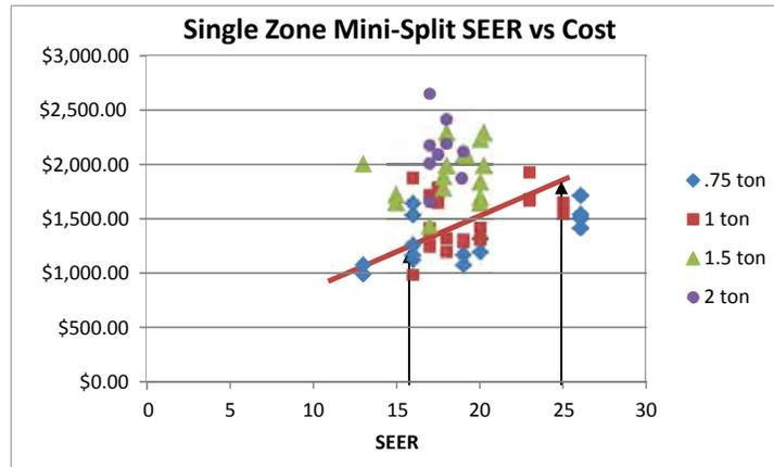
**Figure 28.** Equipment cost versus SEER rating for four sizes of mini-split heat pumps based on an on-line survey, including a best-fit line for the 1-ton units. (Source: survey performed by ██████████ in 2011.)
