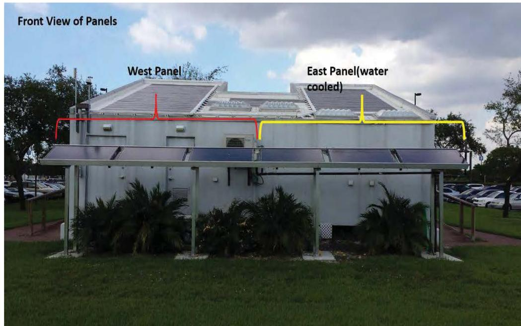
Figure 2-1: The PVT test bed installed at the south end of the FIU Solar House.
