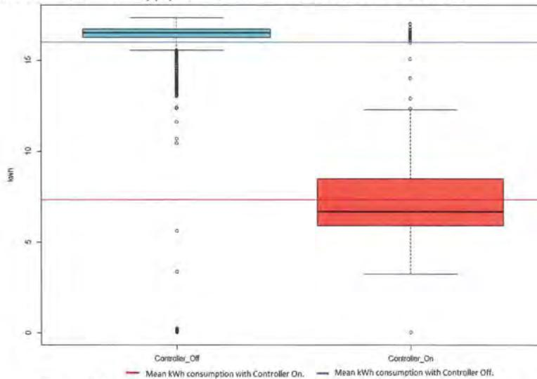
Figure 106: The Box Plot of the Supply Fan kWh and the Controller Status.
