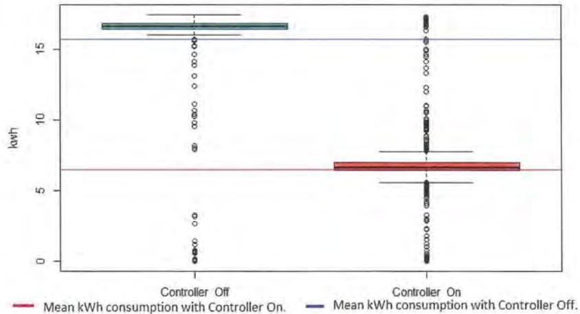
Figure 83: The Box Plot of the Supply Fan kWh and the Controller Status.
