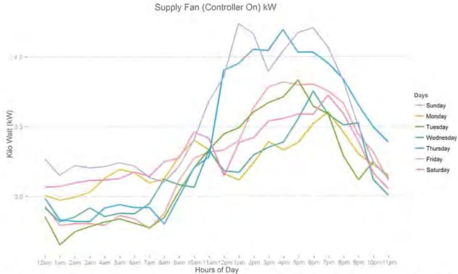
Figure 43: The figure above illustrates the average kWh draw of the supply fan when the controller is ON for each hour of the day and each day of the week. This is helpful in understanding the operation of the unit throughout the days of the week. It is clear that as the temperature increases throughout the day, so will the kWh draw.
