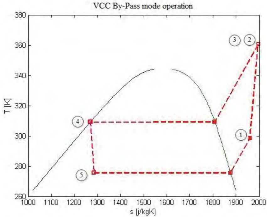
Figure 22: VCC by-pass T-s diagram
