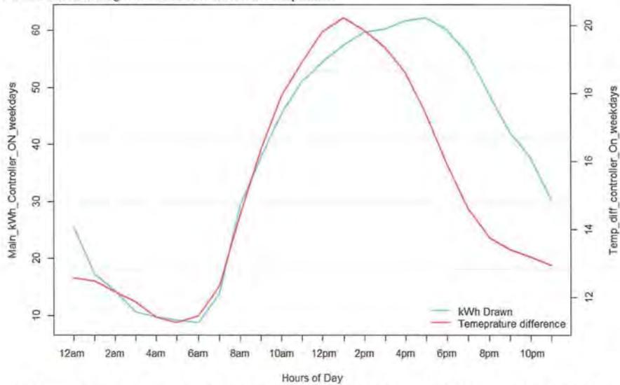
Figure 121: The figure above illustrates the relationship between the main disconnect kWh draw and the indoor and outdoor temperature difference when the controller is ON for the weekday hours (Monday to Friday). As it can be seen, as the temperature difference between indoor and outdoor temperature raises so does the kW consumption of the main disconnect panel. This indicates a high correlation between kW and temperature.
