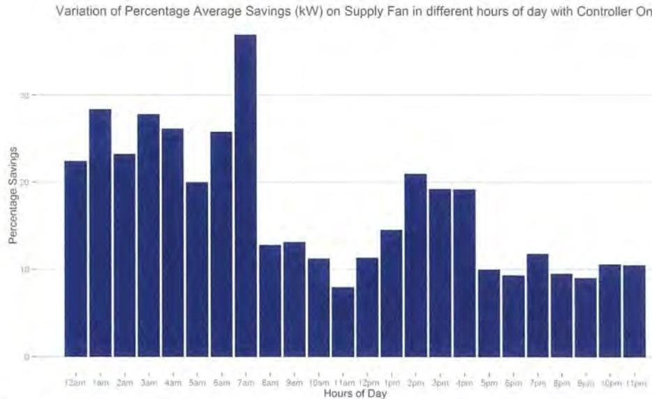
Figure 92: The figure above illustrates the average percent savings of the supply fan throughout the day. As it can be seen, savings are higher during the cooler parts of the day as the VFD is able to slow down the speed of the fan for longer periods of time.
