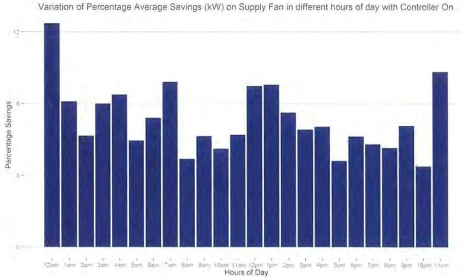
Figure 69: The figure above illustrates the average percent savings of the supply fan throughout the day. As it can be seen, savings are higher during the cooler parts of the day as the VFD is able to slow down the speed of the fan for longer periods of time.
