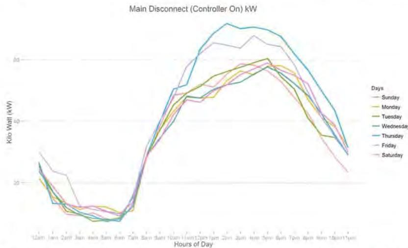
Figure 109: The figure above illustrates the average kWh draw of the main disconnect when the controller is ON for each hour of the day and each day of the week. This is helpful in understanding the operation of the unit throughout the days of the week. It is clear that as the temperature increases throughout the day, so will the kWh draw.
