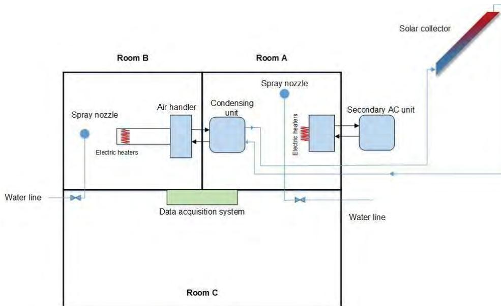
**Figure 2: Schematic diagram of the test facility and installed equipment**
