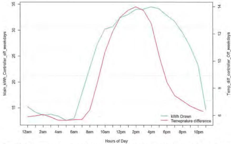
Figure 25: The figure above illustrates the relationship between the main disconnect kWh draw and the indoor and outdoor temperature difference when the controller is OFF for the weekday hours (Monday to Friday). As it can be seen, as the temperature difference between indoor and outdoor temperature increased so does the kW consumption of the main disconnect panel. This indicates a high correlation between kW and temperature.
