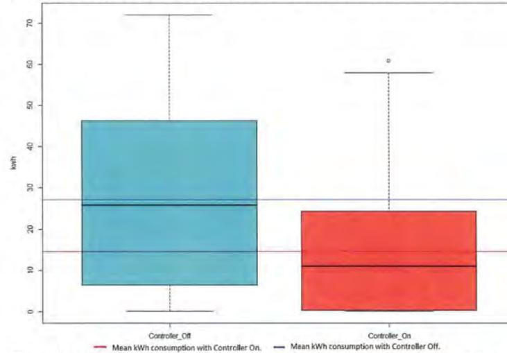
Figure 57: The Box Plot of the Compressor kWh and the Controller Status.
