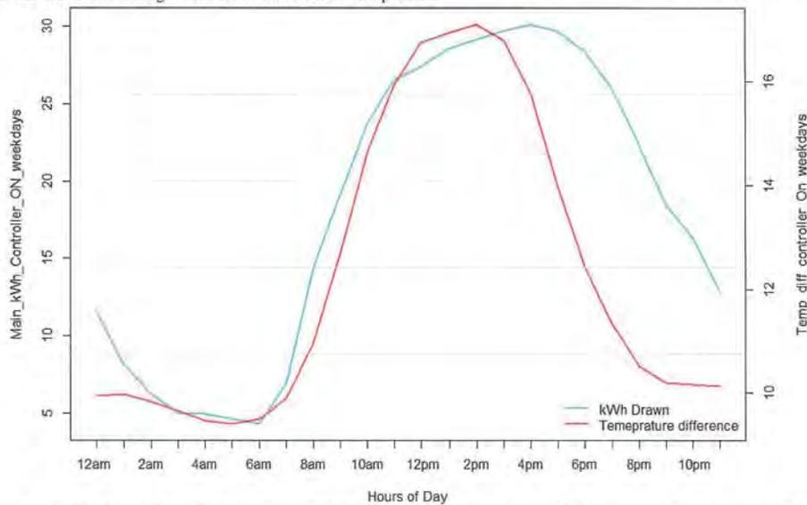
Figure 74: The figure above illustrates the relationship between the main disconnect kWh draw and the indoor and outdoor temperature difference when the controller is ON for the weekday hours (Monday to Friday). As it can be seen, as the temperature difference between indoor and outdoor temperature raises so does the kW consumption of the main disconnect panel. This indicates a high correlation between kW and temperature.
