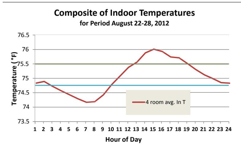
**Figure 17.** The red line is a measured 24-hour space temperature profile in the Building Science Lab for a 7-day period with only the mini-split conditioning the space, with space temperature setpoints used by the mini-split (blue line) and central system (orange line) illustrated.
