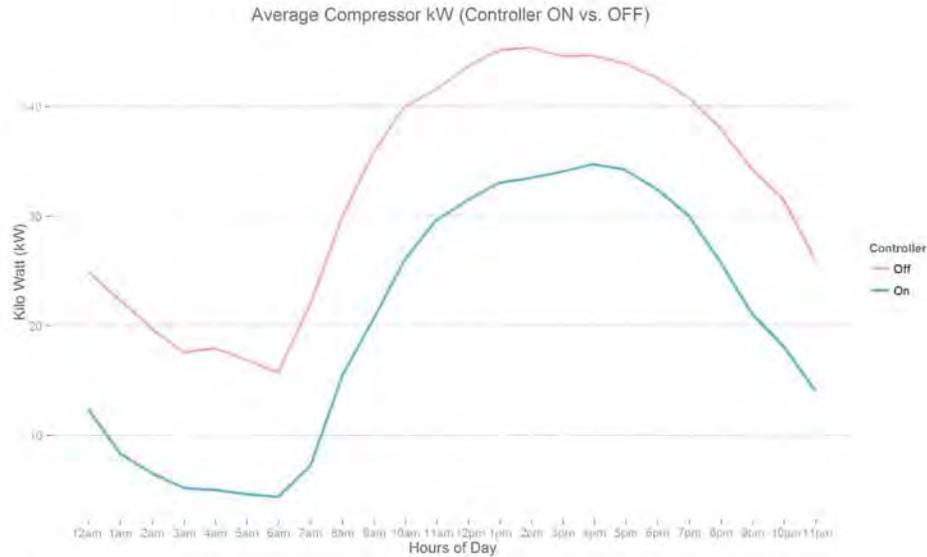
Figure 136: The figure above shows that there is a significant reduction in compressor kWh draw when the controller is ON versus when it is OFF. The kWh draw follows a similar trend throughout the day. This indicates that both control strategies are reacting to the outside temperature and super market occupancy.
