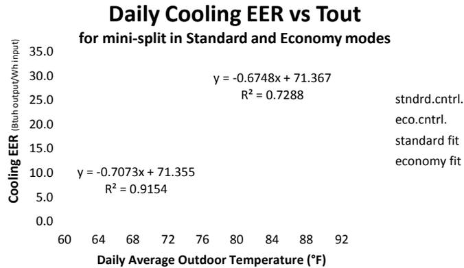
**Figure ES-1.** Monitored mini-split heat pump EER for Standard and Economy modes as a function of daily outdoor temperature with indoor temperature held constant at about 76°F.
