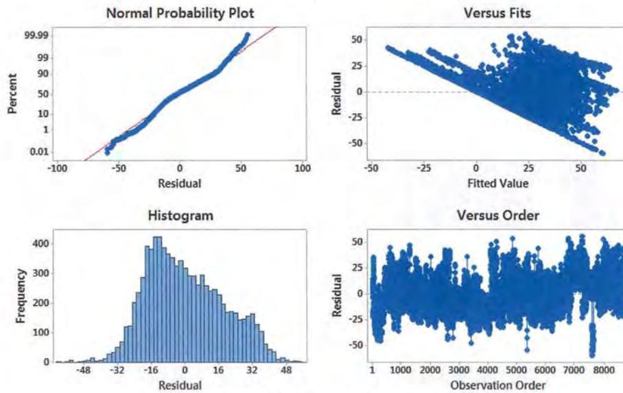
Figure 129: Residual Plots for Compressor kWh
