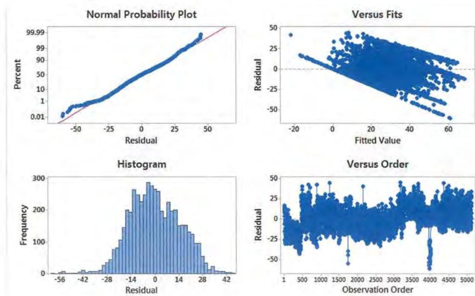
Figure 34: Residual Plots for Compressor kWh
