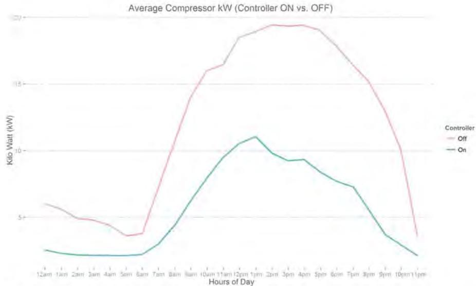
Figure 17: The figure above illustrates that there is a significant reduction in compressor kWh draw when the controller is ON versus when it is OFF. The kWh draw follows a similar trend throughout the day. This indicates that both control strategies are reacting to the outside temperature and super market occupancy.
