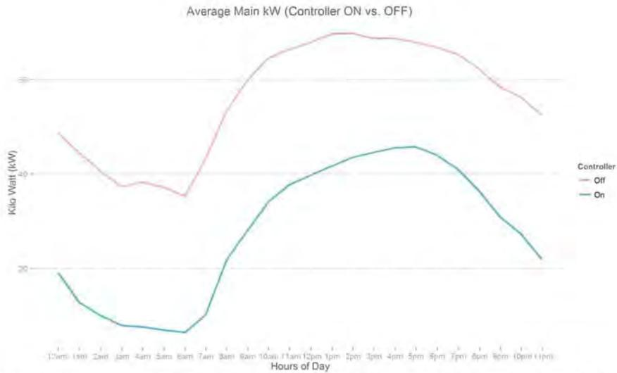
Figure 39: The plot above illustrates that there is a significant reduction in main kWh draw when the controller is ON versus when it is OFF. The kWh draw follows a similar trend throughout the day. This indicates that both control strategies are reacting to the outside temperature and super market occupancy.
