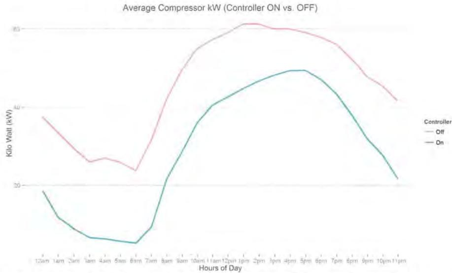
Figure 112: Fig above that there is a significant reduction in compressor kWh draw when the controller is ON versus when it is OFF. The kWh draw follows a similar trend throughout the day. This indicates that both control strategies are reacting to the outside temperature and super market occupancy.
