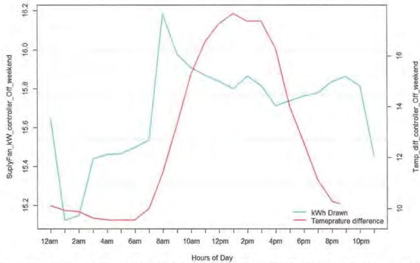
Figure 146: The figure above illustrates the relationship between the supply fan kWh draw and the indoor and outdoor temperature difference when the controller is OFF for the weekend hours (Saturday and Sunday). As it can be seen, as the temperature difference between indoor and outdoor temperature increased so does the kW consumption of the main disconnect panel. This indicates a high correlation between kW and temperature.
