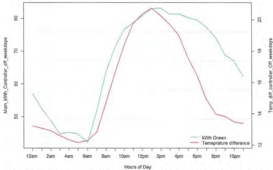
Figure 120: The figure above illustrates the relationship between the main disconnect kWh draw and the indoor and outdoor temperature difference when the controller is OFF for the weekday hours (Monday to Friday). As it can be seen, as the temperature difference between indoor and outdoor temperature increased so does the kW consumption of the main disconnect panel. This indicates a high correlation between kW and temperature.
