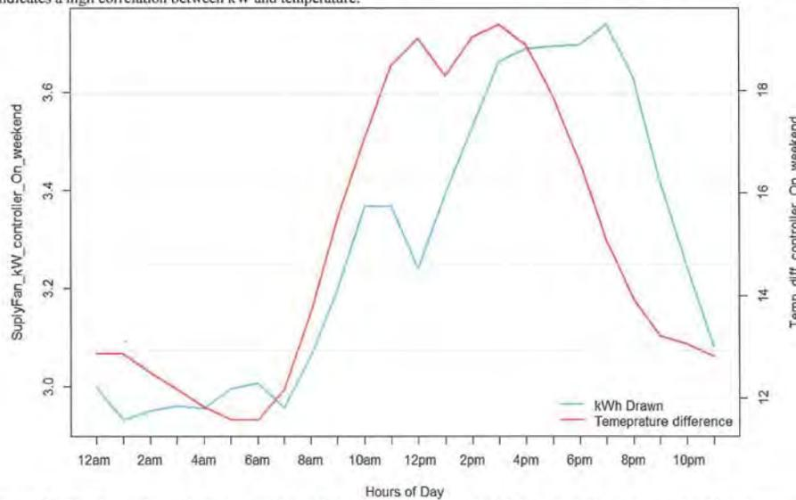
Figure 52: The figure above illustrates the relationship between the supply fan kWh draw and the indoor and outdoor temperature difference when the controller is ON for the weekend hours (Saturday and Sunday). As it can be seen, as the temperature difference between indoor and outdoor temperature raises so does the kW consumption of the main disconnect panel. This indicates a high correlation between kW and temperature.
