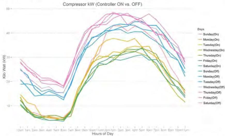
Figure 135: The figure above illustrates the average kWh draw of the compressors when the controller is ON and OFF for each hour of the day and each day of the week. This is helpful in understanding the operation of the unit throughout the days of the week. It is clear that as the temperature increases throughout the day, so will the kWh draw.
