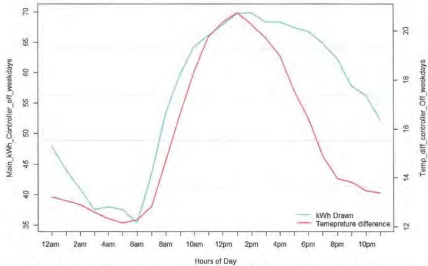
Figure 49: The figure above illustrates the relationship between the main disconnect kWh draw and the indoor and outdoor temperature difference when the controller is OFF for the weekday hours (Monday to Friday). As it can be seen, as the temperature difference between indoor and outdoor temperature increased so does the kW consumption of the main disconnect panel. This indicates a high correlation between kW and temperature.
