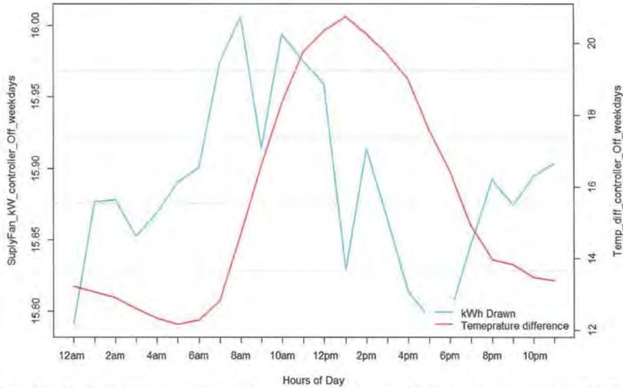
Figure 124: The figure above illustrates the relationship between the supply fan kWh draw and the indoor and outdoor temperature difference when the controller is OFF for the weekday hours (Monday to Friday). As it can be seen, as the temperature difference between indoor and outdoor temperature increased so does the kW consumption of the main disconnect panel. This indicates a high correlation between kW and temperature.
