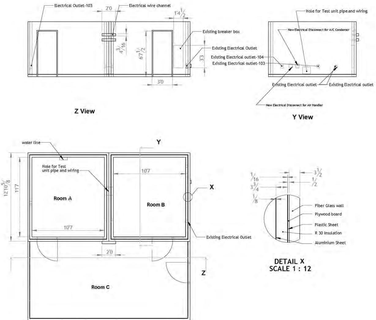
Figure 1: HVAC facility Layout
