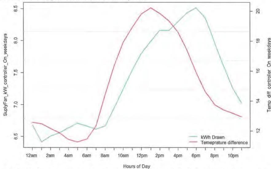
Figure 125: The figure above illustrates the relationship between the supply fan kWh draw and the indoor and outdoor temperature difference when the controller is ON for the weekday hours (Monday to Friday). As it can be seen, as the temperature difference between indoor and outdoor temperature raises so does the kW consumption of the main disconnect panel. This indicates a high correlation between kW and temperature.
