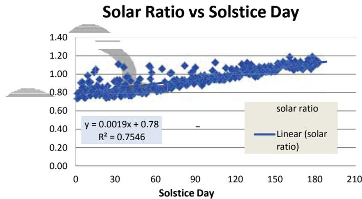
**Figure 13.** Solar ratio, which is used to convert solar radiation on the horizontal to solar radiation at PV array tilt, varies as a function of day of the year. Solstice day increases from 1 to 183 from December 21 to June 21, and then decreases from 183 to 1 from June 21 to December 21.
