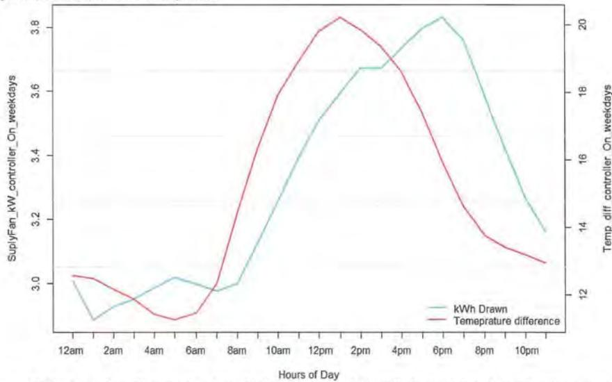
Figure 54: The figure above illustrates the relationship between the supply fan kWh draw and the indoor and outdoor temperature difference when the controller is ON for the weekday hours (Monday to Friday). As it can be seen, as the temperature difference between indoor and outdoor temperature raises so does the kW consumption of the main disconnect panel. This indicates a high correlation between kW and temperature.
