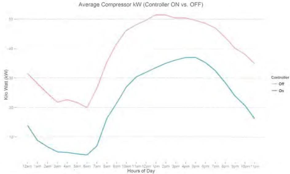
Figure 41: The plot above that there is a significant reduction in compressor kWh draw when the controller is ON versus when it is OFF. The kWh draw follows a similar trend throughout the day. This indicates that both control strategies are reacting to the outside temperature and super market occupancy.
