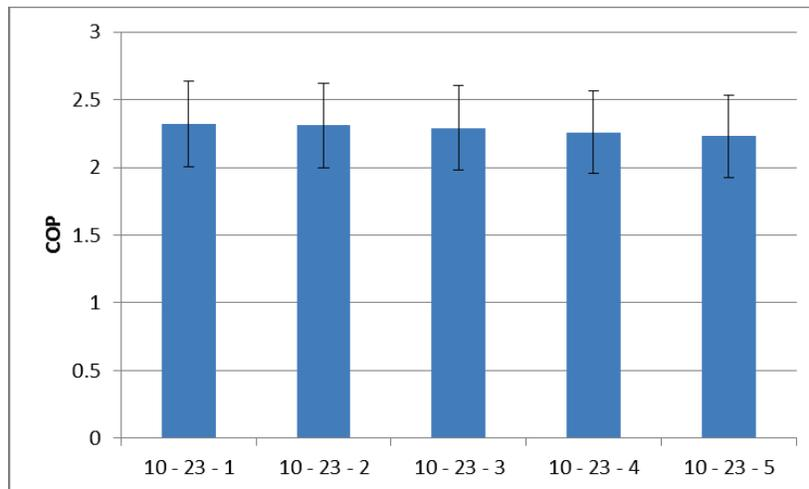
Figure 20: Solar test performance of the AC unit (CASE II)
