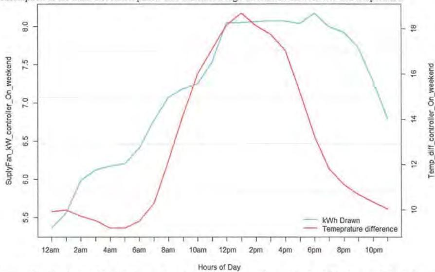
Figure 147: The figure above illustrates the relationship between the supply fan kWh draw and the indoor and outdoor temperature difference when the controller is ON for the weekend hours (Saturday and Sunday). As it can be seen, as the temperature difference between indoor and outdoor temperature raises so does the kW consumption of the main disconnect panel. This indicates a high correlation between kW and temperature.
