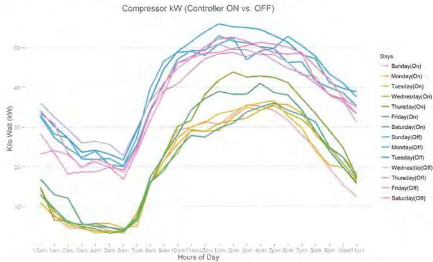
Figure 40: The figure above illustrates the average kWh draw of the compressors when the controller is ON and OFF for each hour of the day and each day of the week. This is helpful in understanding the operation of the unit throughout the days of the week. It is clear that as the temperature increases throughout the day, so will the kWh draw.
