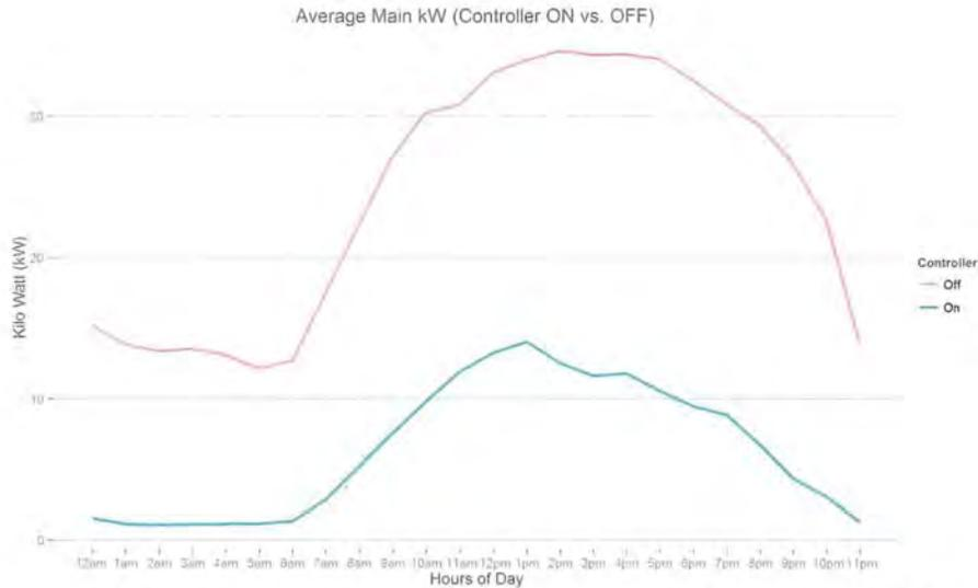
Figure 15: The figure above shows that there is a significant reduction in main kWh draw when the controller is ON versus when it is OFF. The kWh draw follows a similar trend throughout the day. This indicates that both control strategies are reacting to the outside temperature and super market occupancy.
