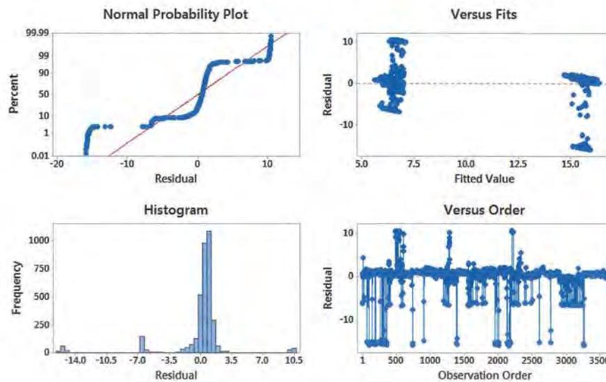
Figure 84: Residual Plots for Supply Fan kWh
