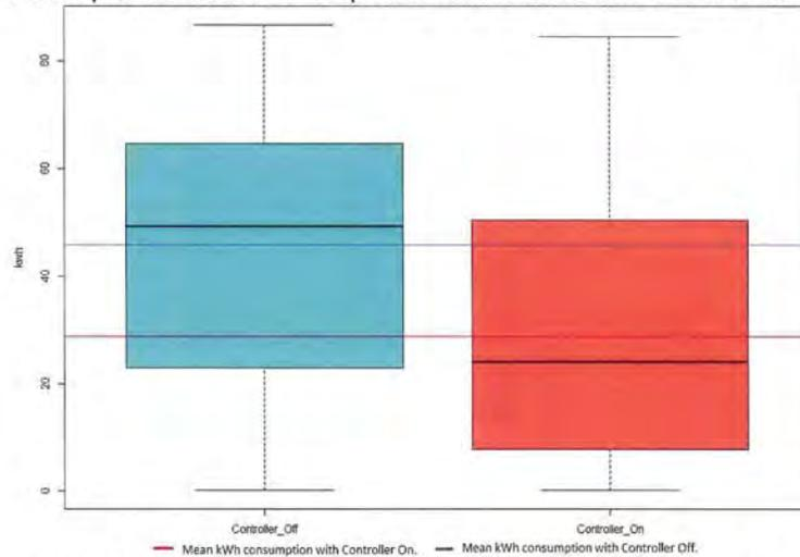
Figure 104: The Box Plot of the Compressor kWh and the Controller Status.
