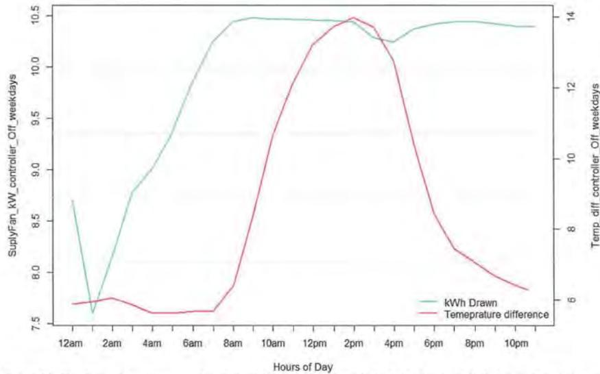
Figure 29: The figure above illustrates the relationship between the supply fan kWh draw and the indoor and outdoor temperature difference when the controller is OFF for the weekday hours (Monday to Friday). As it can be seen, as the temperature difference between indoor and outdoor temperature increased so does the kW consumption of the main disconnect panel. This indicates a high correlation between kW and temperature.
