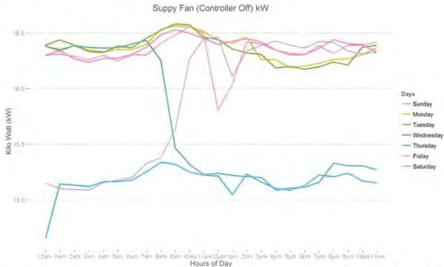
Figure 113: The figure above illustrates the average kWh draw of the supply fan when the controller is OFF for each hour of the day and each day of the week. This is helpful in understanding the operation of the unit throughout the days of the week. It is clear that as the temperature increases throughout the day, so will the kWh draw.
