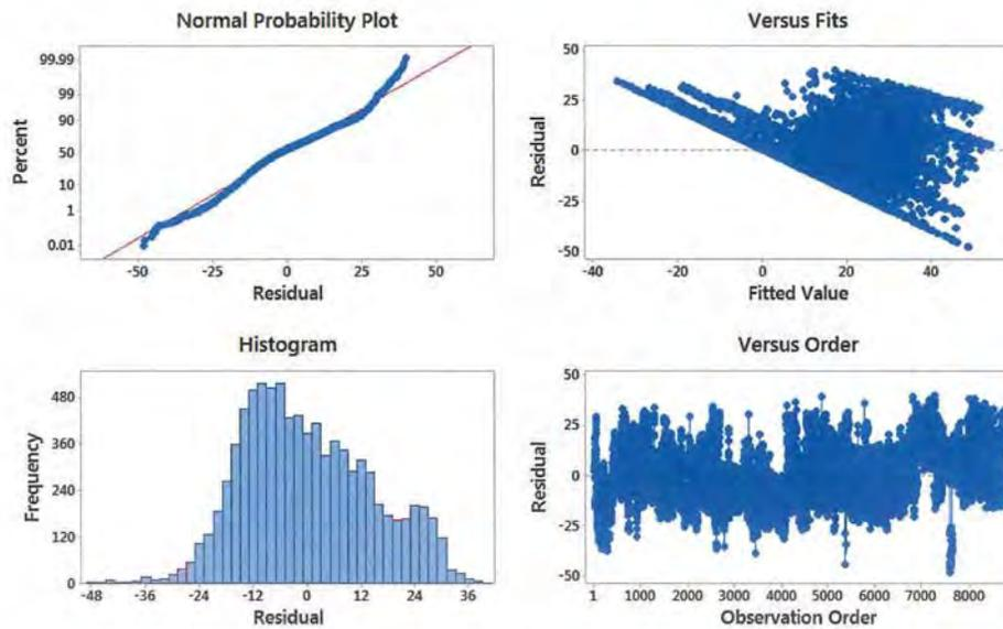
Figure 58: Residual Plots for Compressor kWh
