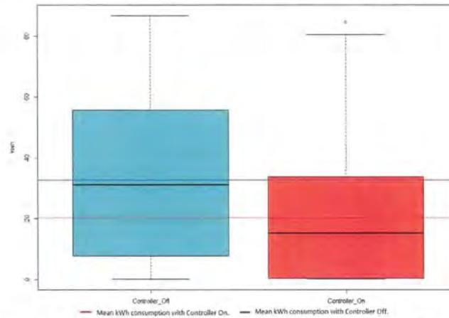
Figure 128: The Box Plot of the Compressor kWh and the Controller Status.
