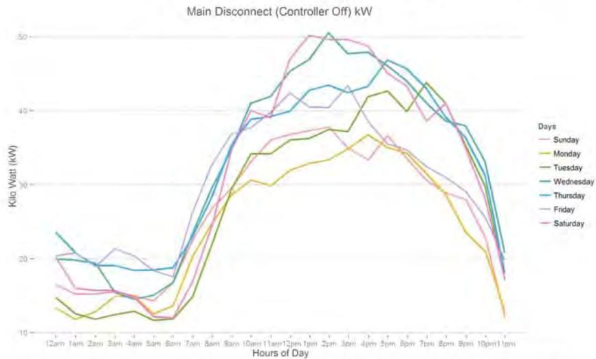
Figure 85: The figure above illustrates the average kWh draw of the main disconnect when the controller is OFF for each hour of the day and each day of the week. This is helpful in understanding the operation of the unit throughout the days of the week. It is clear that as the temperature increases throughout the day, so will the kWh draw.
