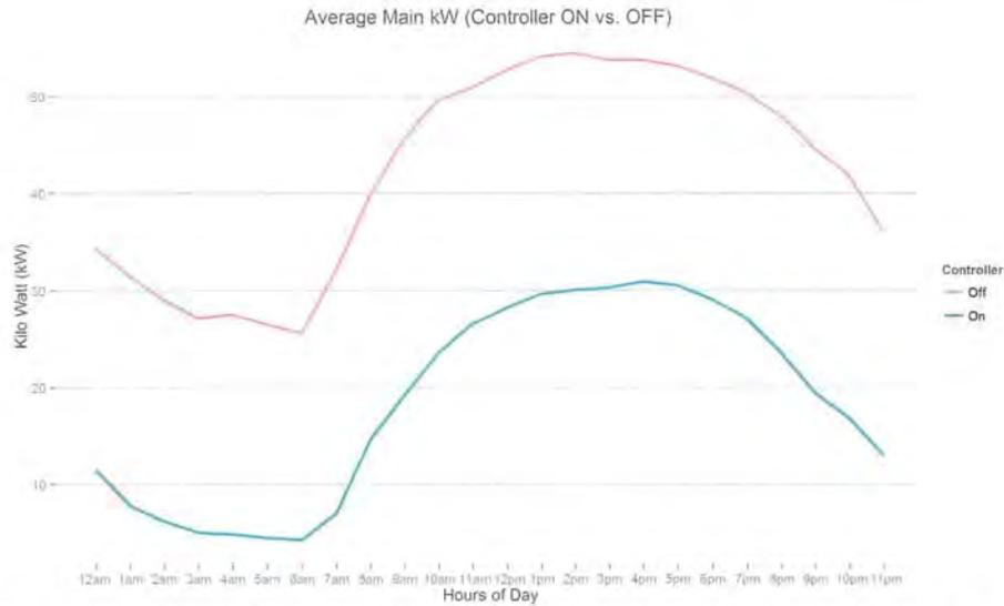
Figure 63: The plot above illustrates that there is a significant reduction in main kWh draw when the controller is ON versus when it is OFF. The kWh draw follows a similar trend throughout the day. This indicates that both control strategies are reacting to the outside temperature and super market occupancy.
