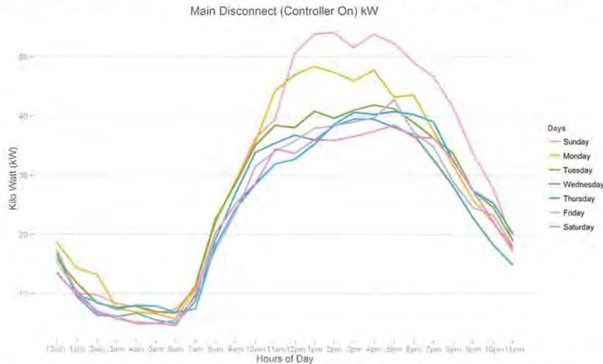
Figure 133: The figure above illustrates the average kWh draw of the main disconnect when the controller is ON for each hour of the day and each day of the week. This is helpful in understanding the operation of the unit throughout the days of the week. It is clear that as the temperature increases throughout the day, so will the kWh draw.
