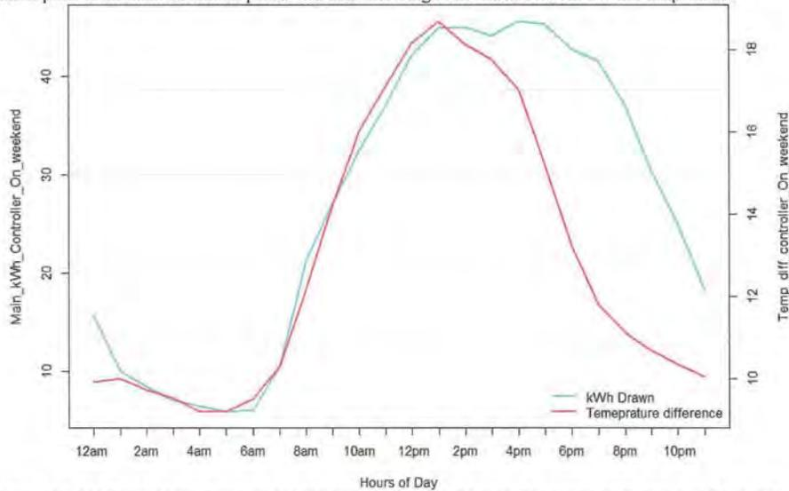
Figure 143: The figure above illustrates the relationship between the main disconnect kWh draw and the indoor and outdoor temperature difference when the controller is ON for the weekend hours (Saturday and Sunday). As it can be seen, as the temperature difference between indoor and outdoor temperature raises so does the kW consumption of the main disconnect panel. This indicates a high correlation between kW and temperature.
