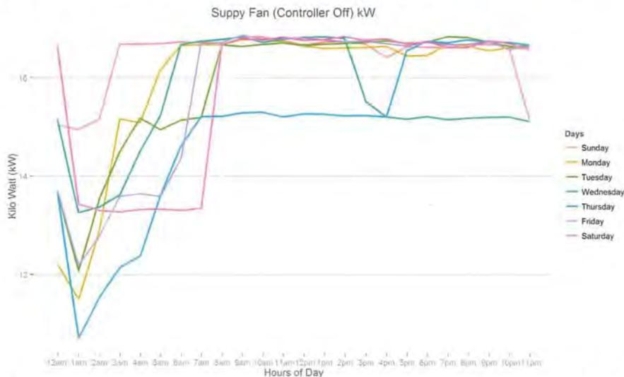
Figure 90: The figure above illustrates the average kWh draw of the supply fan when the controller is OFF for each hour of the day and each day of the week. This is helpful in understanding the operation of the unit throughout the days of the week. It is clear that as the temperature increases throughout the day, so will the kWh draw.
