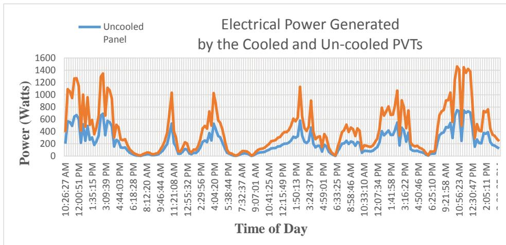
**Figure 3-1:** Electrical power generated by the cooled and un-cooled PVTs for a period of 5 days in 9/21/2014 – 9/26/2014.
