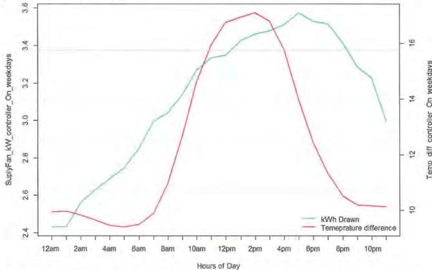
Figure 78: The figure above illustrates the relationship between the supply fan kWh draw and the indoor and outdoor temperature difference when the controller is ON for the weekday hours (Monday to Friday). As it can be seen, as the temperature difference between indoor and outdoor temperature raises so does the kW consumption of the main disconnect panel. This indicates a high correlation between kW and temperature.
