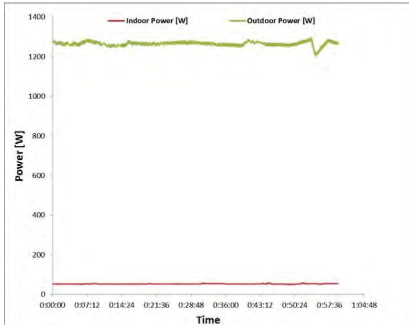
Figure 12: Solar test AHU and condensing unit electric power consumption (CASE I)
