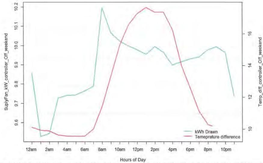
Figure 75: The figure above illustrates the relationship between the supply fan kWh draw and the indoor and outdoor temperature difference when the controller is OFF for the weekend hours (Saturday and Sunday). As it can be seen, as the temperature difference between indoor and outdoor temperature increased so does the kW consumption of the main disconnect panel. This indicates a high correlation between kW and temperature.
