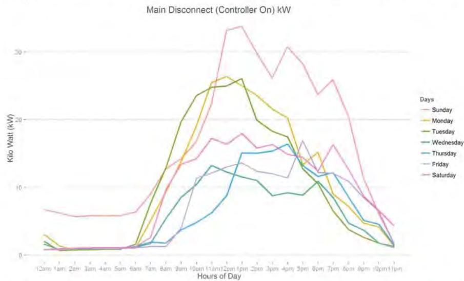
Figure 86: The figure above illustrates the average kWh draw of the main disconnect when the controller is ON for each hour of the day and each day of the week. This is helpful in understanding the operation of the unit throughout the days of the week. It is clear that as the temperature increases throughout the day, so will the kWh draw.
