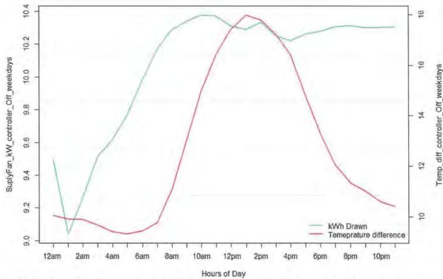
Figure 77: The figure above illustrates the relationship between the supply fan kWh draw and the indoor and outdoor temperature difference when the controller is OFF for the weekday hours (Monday to Friday). As it can be seen, as the temperature difference between indoor and outdoor temperature increased so does the kW consumption of the main disconnect panel. This indicates a high correlation between kW and temperature.
