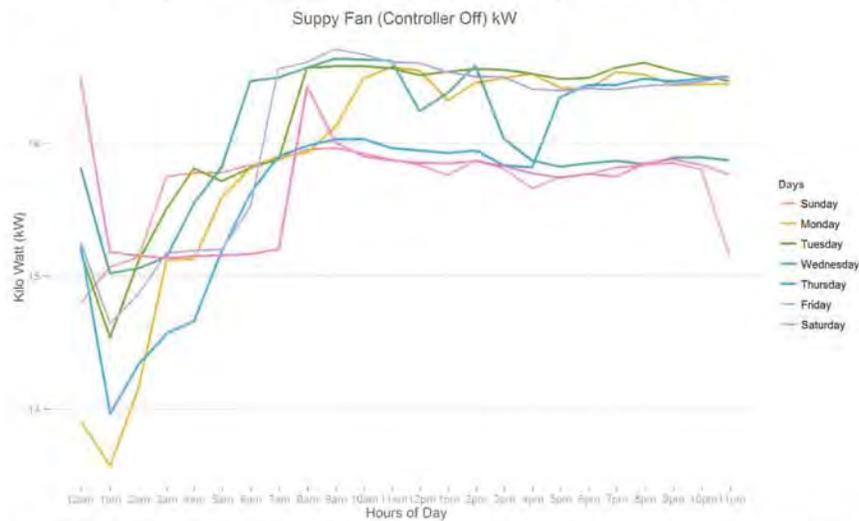
Figure 137: The figure above illustrates the average kWh draw of the supply fan when the controller is OFF for each hour of the day and each day of the week. This is helpful in understanding the operation of the unit throughout the days of the week. It is clear that as the temperature increases throughout the day, so will the kWh draw.
