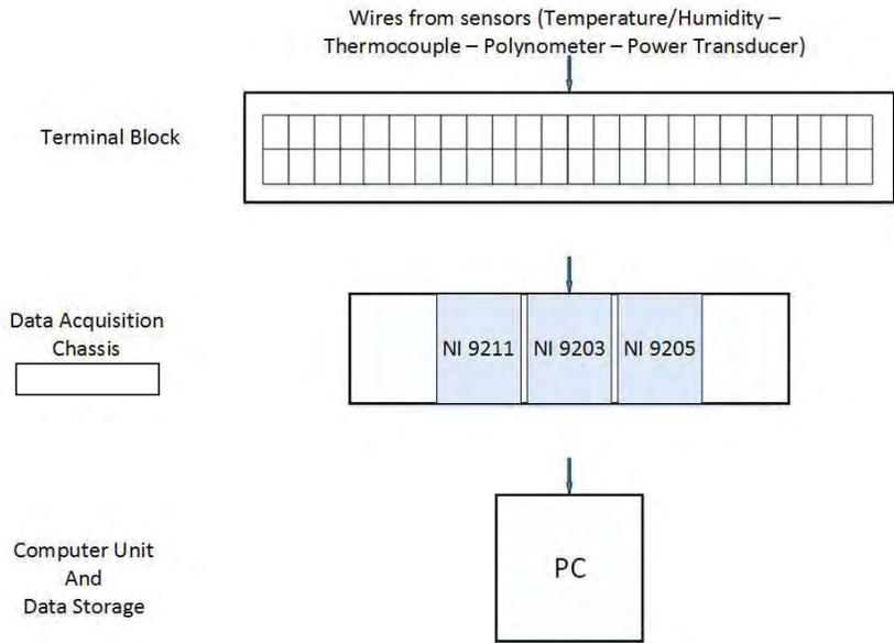
**Figure 4: Data Acquisition System**
