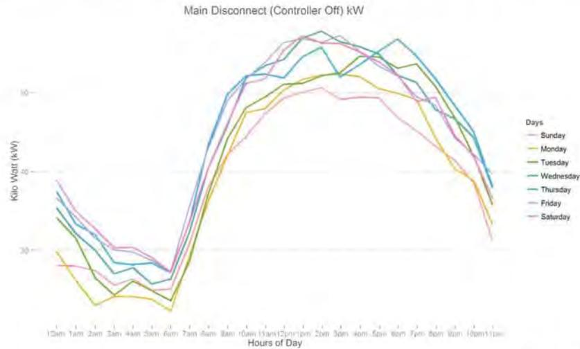
Figure 61: The figure above illustrates the average kWh draw of the main disconnect when the controller is OFF for each hour of the day and each day of the week. This is helpful in understanding the operation of the unit throughout the days of the week. It is clear that as the temperature increases throughout the day, so will the kWh draw.
