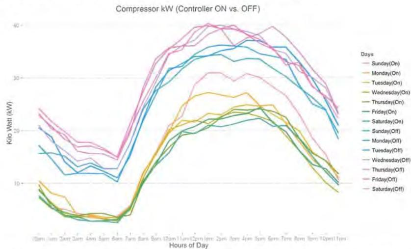
Figure 64: The figure above illustrates the average kWh draw of the compressors when the controller is ON and OFF for each hour of the day and each day of the week. This is helpful in understanding the operation of the unit throughout the days of the week. It is clear that as the temperature increases throughout the day, so will the kWh draw.
