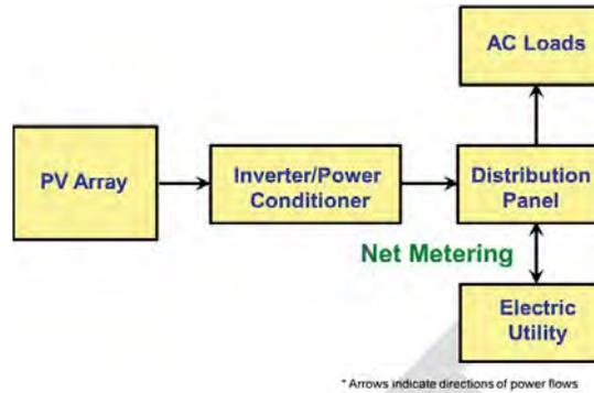
Figure 23. Utility Grid-Interactive PV System
