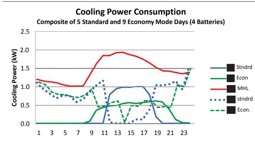
Figure 16. Twenty-four hour cooling power consumption profile for Standard and Economy mini-split operation when using 4 batteries, plus cooling power consumption for the Lab SEER 13 central system.
