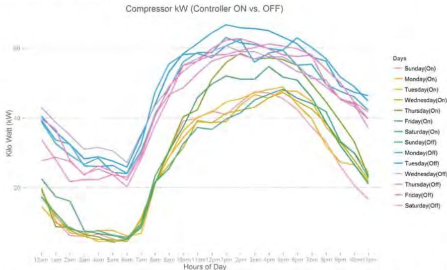
Figure 111: The figure above illustrates the average kWh draw of the compressors when the controller is ON and OFF for each hour of the day and each day of the week. This is helpful in understanding the operation of the unit throughout the days of the week. It is clear that as the temperature increases throughout the day, so will the kWh draw.
