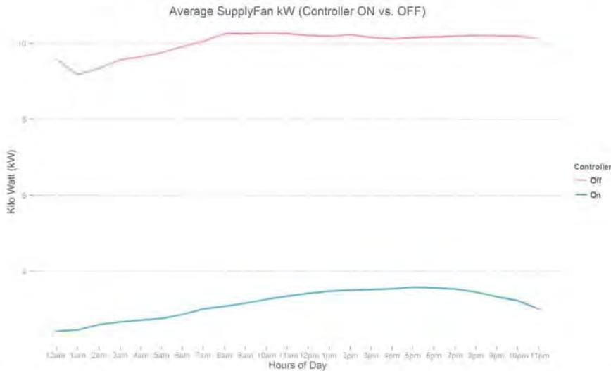
Figure 70: Figure above illustrates that there is a significant reduction in supply fan kWh draw when the controller is ON versus when it is OFF. The kWh draw follows a similar trend throughout the day. This indicates that both control strategies are reacting to the outside temperature and super market occupancy.
