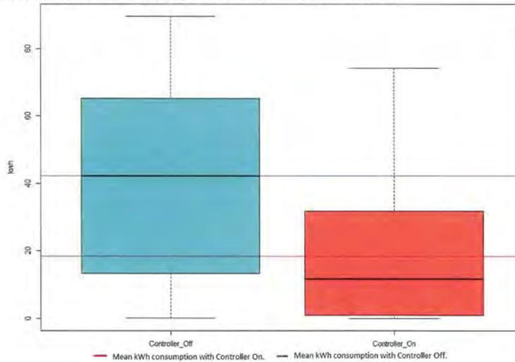
Figure 55: The Box Plot of the Main kWh and the Controller Status.
