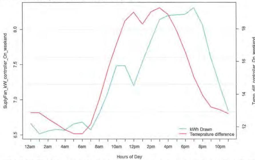
Figure 123: The figure above illustrates the relationship between the supply fan kWh draw and the indoor and outdoor temperature difference when the controller is ON for the weekend hours (Saturday and Sunday). As it can be seen, as the temperature difference between indoor and outdoor temperature raises so does the kW consumption of the main disconnect panel. This indicates a high correlation between kW and temperature.
