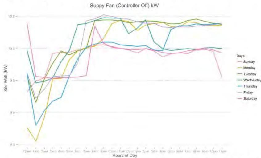
Figure 66: The figure above illustrates the average kWh draw of the supply fan when the controller is OFF for each hour of the day and each day of the week. This is helpful in understanding the operation of the unit throughout the days of the week. It is clear that as the temperature increases throughout the day, so will the kWh draw.
