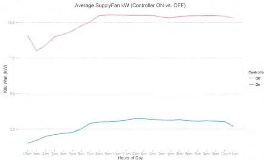
Figure 22: This plot illustrates that there is a significant reduction in supply fan kWh draw when the controller is ON versus when it is OFF. The kWh draw follows a similar trend throughout the day. This indicates that both control strategies are reacting to the outside temperature and super market occupancy.
