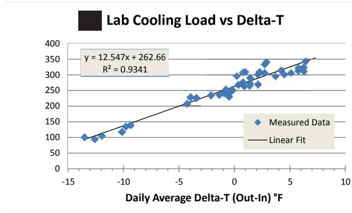
Figure 11. Daily Lab cooling load versus delta-T (out – in) when using attic ducts.
