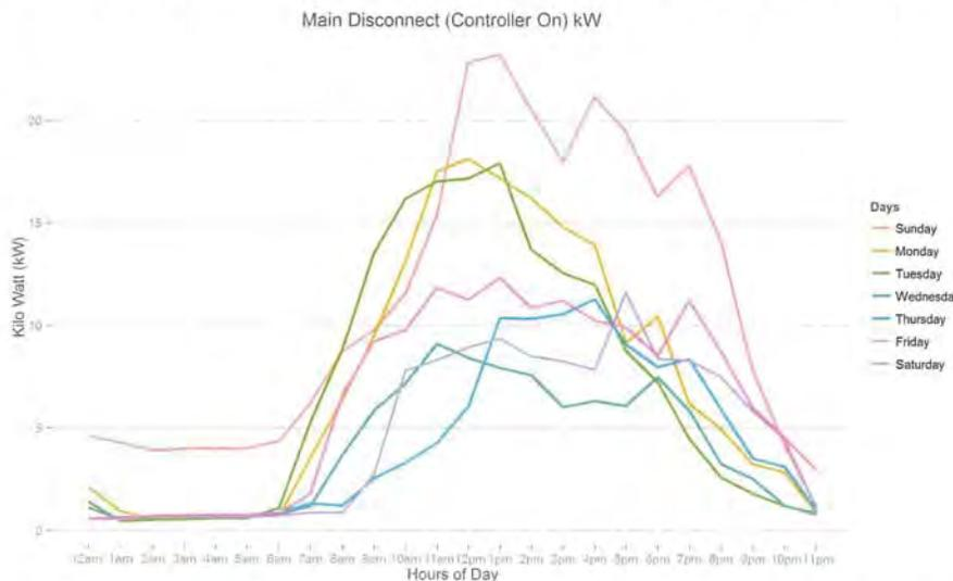
Figure 14: The figure above illustrates the average kWh draw of the main A/C unit when the controller is ON for each hour of the day and each day of the week. This is helpful in understanding the operation of the unit throughout the days of the week. It is clear that as the temperature increases throughout the day, so will the kWh draw.
