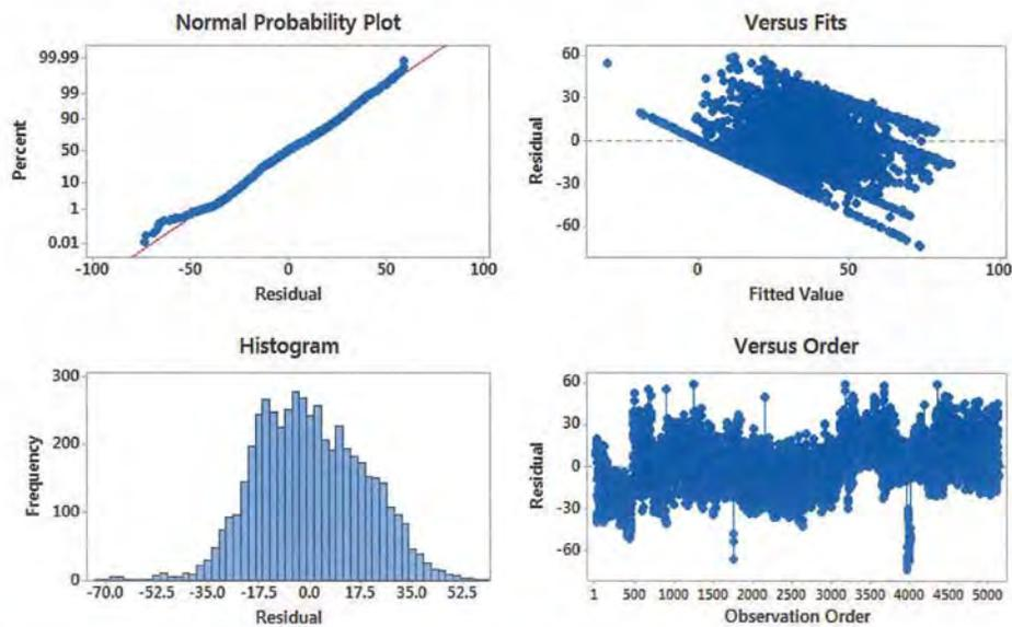
Figure 105: Residual Plots for Compressor kWh
