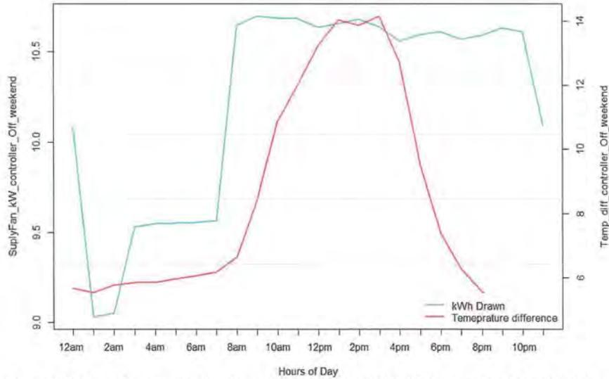
Figure 27: The figure above illustrates the relationship between the supply fan kWh draw and the indoor and outdoor temperature difference when the controller is OFF for the weekend hours (Saturday and Sunday). As it can be seen, as the temperature difference between indoor and outdoor temperature increased so does the kW consumption of the main disconnect panel. This indicates a high correlation between kW and temperature.
