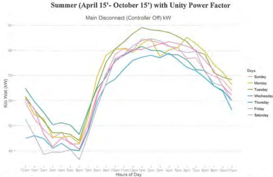
Figure 108: The figure above illustrates the average kWh draw of the main disconnect when the controller is OFF for each hour of the day and each day of the week. This is helpful in understanding the operation of the unit throughout the days of the week. It is clear that as the temperature increases throughout the day, so will the kWh draw.
