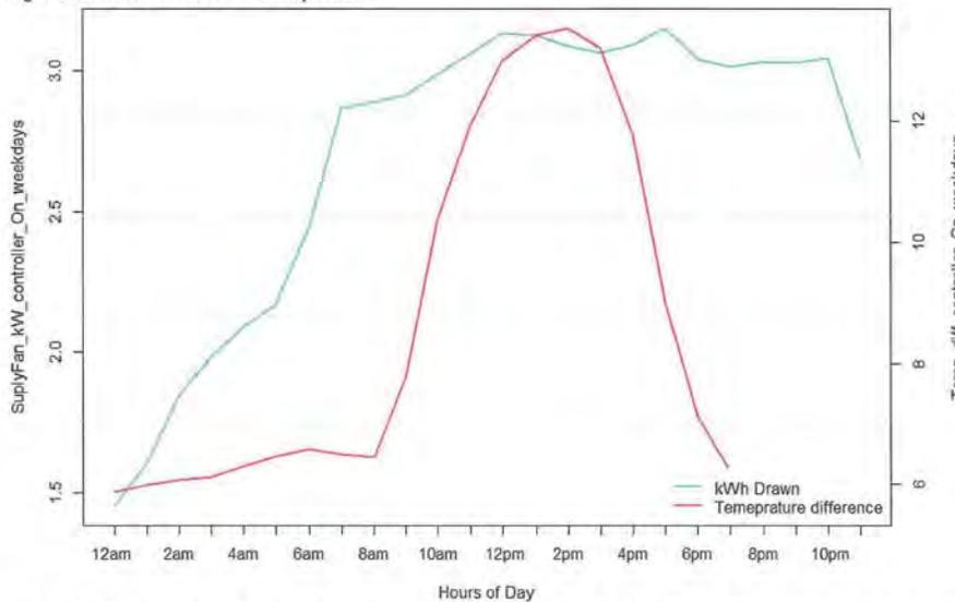
Figure 30: The figure above illustrates the relationship between the supply fan kWh draw and the indoor and outdoor temperature difference when the controller is ON for the weekday hours (Monday to Friday). As it can be seen, as the temperature difference between indoor and outdoor temperature raises so does the kW consumption of the main disconnect panel. This indicates a high correlation between kW and temperature.
