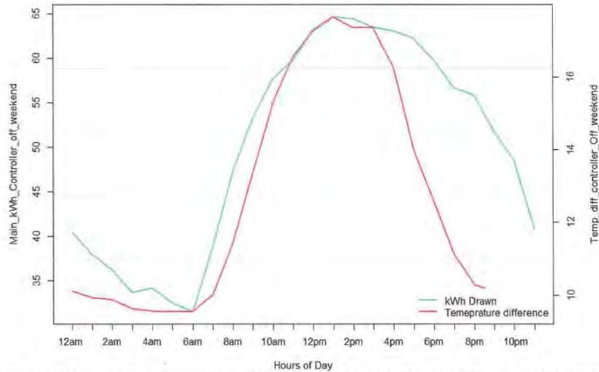
Figure 142: The figure above illustrates the relationship between the main disconnect kWh draw and the indoor and outdoor temperature difference when the controller is OFF for the weekend hours (Saturday and Sunday). As it can be seen, as the temperature difference between indoor and outdoor temperature increased so does the kW consumption of the main disconnect panel. This indicates a high correlation between kW and temperature.
