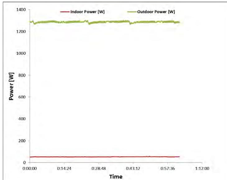
Figure 17: Solar test AHU and Condensing Unit electric power consumption (CASE II)
