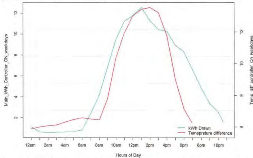
Figure 26: The figure above illustrates the relationship between the main disconnect kWh draw and the indoor and outdoor temperature difference when the controller is ON for the weekday hours (Monday to Friday). As it can be seen, as the temperature difference between indoor and outdoor temperature raises so does the kW consumption of the main disconnect panel. This indicates a high correlation between kW and temperature.
