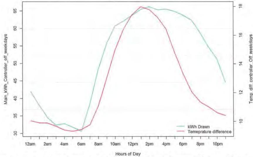
Figure 144: The figure above illustrates the relationship between the main disconnect kWh draw and the indoor and outdoor temperature difference when the controller is OFF for the weekday hours (Monday to Friday). As it can be seen, as the temperature difference between indoor and outdoor temperature increased so does the kW consumption of the main disconnect panel. This indicates a high correlation between kW and temperature.
