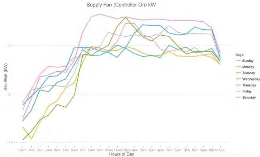
Figure 19: The figure above illustrates the average kWh draw of the supply fan when the controller is ON for each hour of the day and each day of the week. This is helpful in understanding the operation of the unit throughout the days of the week. It is clear that as the temperature increases throughout the day, so will the kWh draw.
