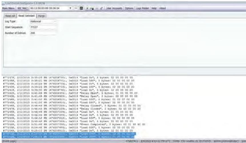
Inactive Appliance test for the switch controlling water heater and AC.
