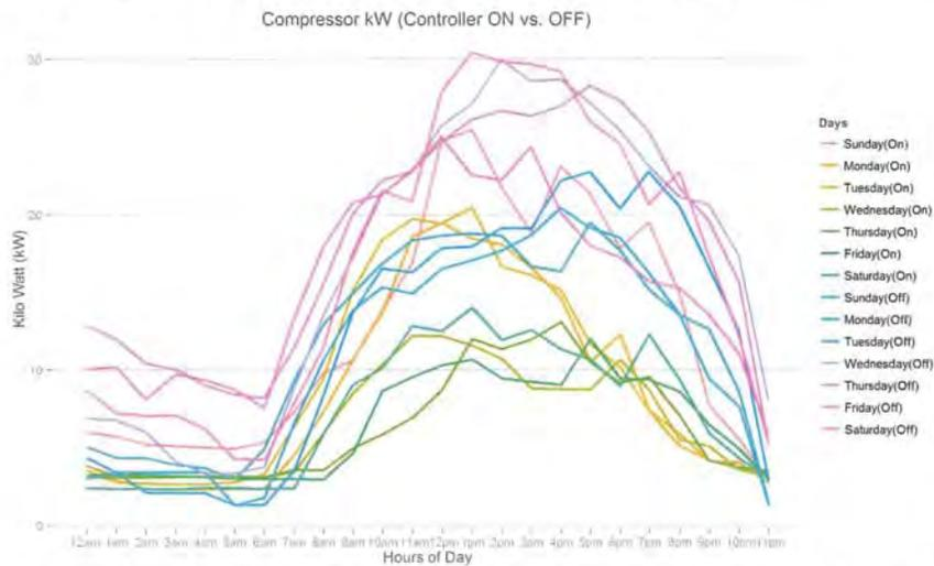
Figure 88: The figure above illustrates the average kWh draw of the compressors when the controller is ON and OFF for each hour of the day and each day of the week. This is helpful in understanding the operation of the unit throughout the days of the week. It is clear that as the temperature increases throughout the day, so will the kWh draw.
