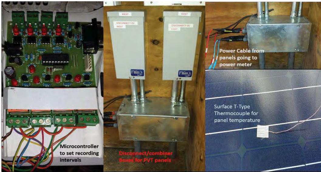
Figure 2-7 Microcontroller, DC-disconnect/Combiner, Surface thermocouple.
