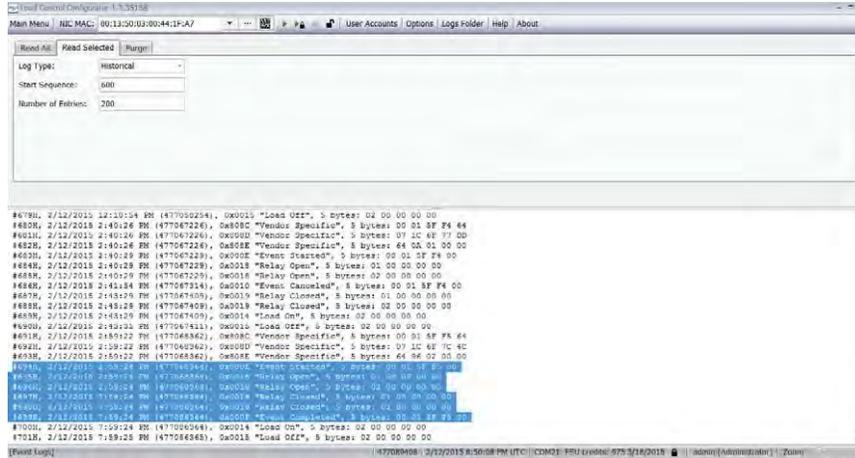
team checked the configuration file and apparently there was mistake creating the file. Loaded configuration file had maximum control duration parameter set to zero which means no limited control duration period.
