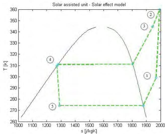
**Figure 24: VCC T-s diagram - (CASE I)**
