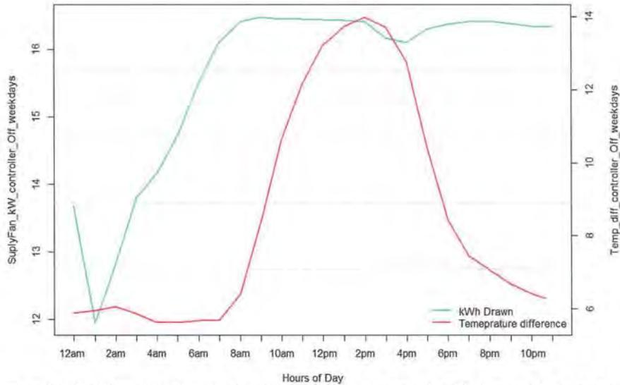
Figure 100: The figure above illustrates the relationship between the supply fan kWh draw and the indoor and outdoor temperature difference when the controller is OFF for the weekday hours (Monday to Friday). As it can be seen, as the temperature difference between indoor and outdoor temperature increased so does the kW consumption of the main disconnect panel. This indicates a high correlation between kW and temperature.
