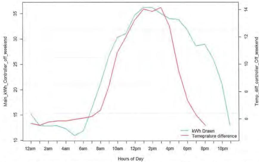
Figure 23: The figure above illustrates the relationship between the main disconnect kWh draw and the indoor and outdoor temperature difference when the controller is OFF for the weekend hours (Saturday and Sunday). As it can be seen, as the temperature difference between indoor and outdoor temperature increased so does the kW consumption of the main disconnect panel. This indicates a high correlation between kW and temperature.
