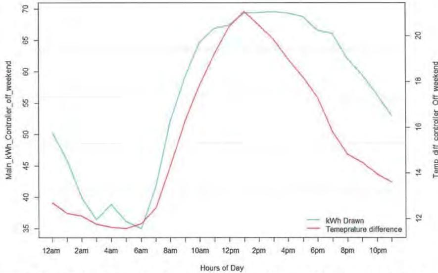
Figure 47: The figure above illustrates the relationship between the main disconnect kWh draw and the indoor and outdoor temperature difference when the controller is OFF for the weekend hours (Saturday and Sunday). As it can be seen, as the temperature difference between indoor and outdoor temperature increased so does the kW consumption of the main disconnect panel. This indicates a high correlation between kW and temperature.
