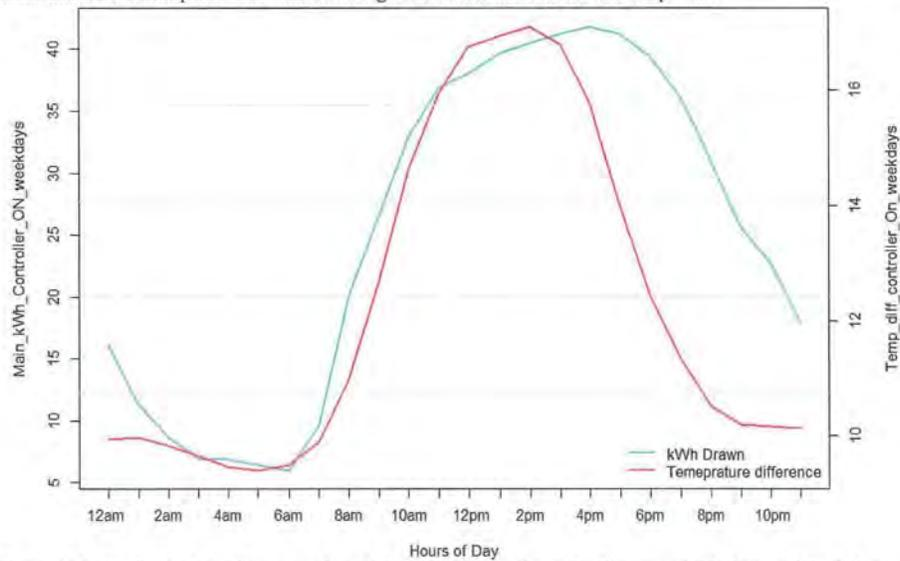
Figure 145: The figure above illustrates the relationship between the main disconnect kWh draw and the indoor and outdoor temperature difference when the controller is ON for the weekday hours (Monday to Friday). As it can be seen, as the temperature difference between indoor and outdoor temperature raises so does the kW consumption of the main disconnect panel. This indicates a high correlation between kW and temperature.
