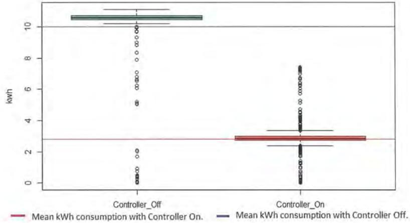
Figure 11: The Box Plot of the Supply Fan kWh and the Controller Status.
