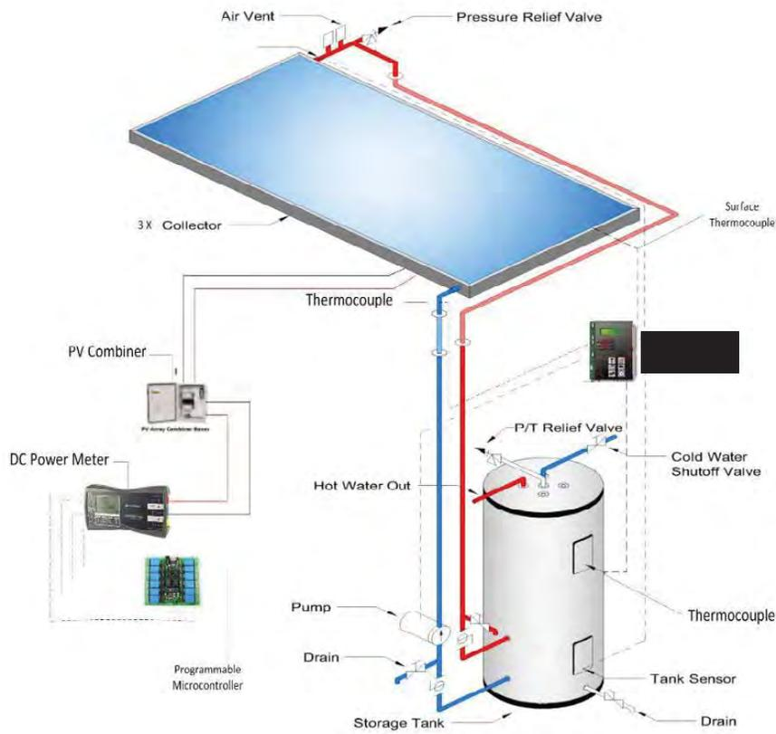
Figure 2-2: Schematic description of the PVT test bed.
