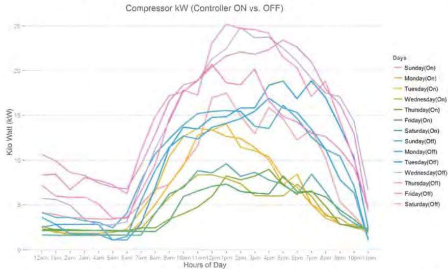
Figure 16: The figure above illustrates the average kWh draw of the compressors when the controller is ON and OFF for each hour of the day and each day of the week. This is helpful in understanding the operation of the unit throughout the days of the week. It is clear that as the temperature increases throughout the day, so will the kWh draw.
