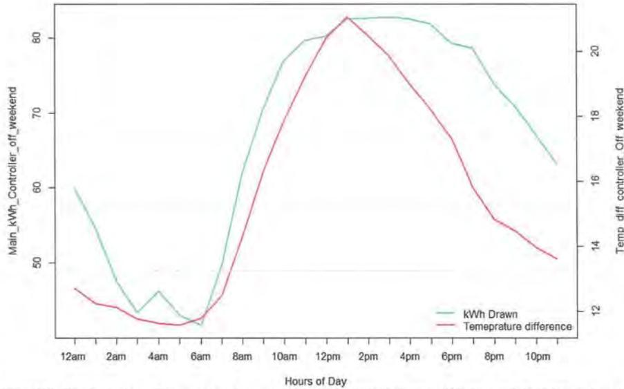
Figure 118: The figure above illustrates the relationship between the main disconnect kWh draw and the indoor and outdoor temperature difference when the controller is OFF for the weekend hours (Saturday and Sunday). As it can be seen, as the temperature difference between indoor and outdoor temperature increased so does the kW consumption of the main disconnect panel. This indicates a high correlation between kW and temperature.
