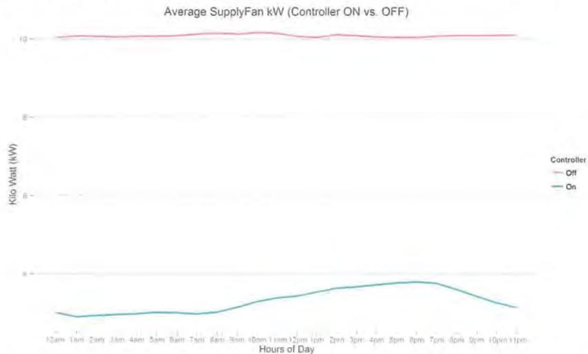
Figure 46: Figure above illustrates that there is a significant reduction in supply fan kWh draw when the controller is ON versus when it is OFF. The kWh draw follows a similar trend throughout the day. This indicates that both control strategies are reacting to the outside temperature and super market occupancy.
