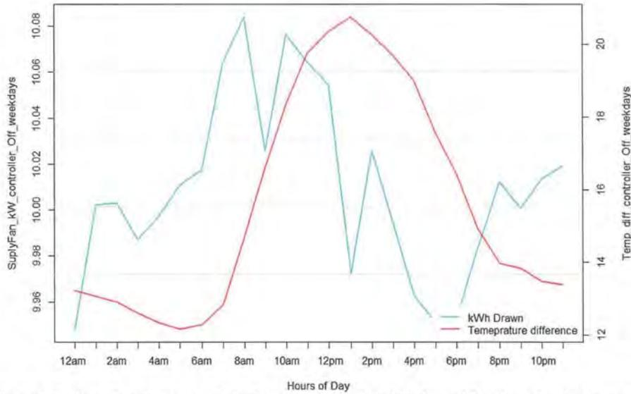
Figure 53: The figure above illustrates the relationship between the supply fan kWh draw and the indoor and outdoor temperature difference when the controller is OFF for the weekday hours (Monday to Friday). As it can be seen, as the temperature difference between indoor and outdoor temperature increased so does the kW consumption of the main disconnect panel. This indicates a high correlation between kW and temperature.
