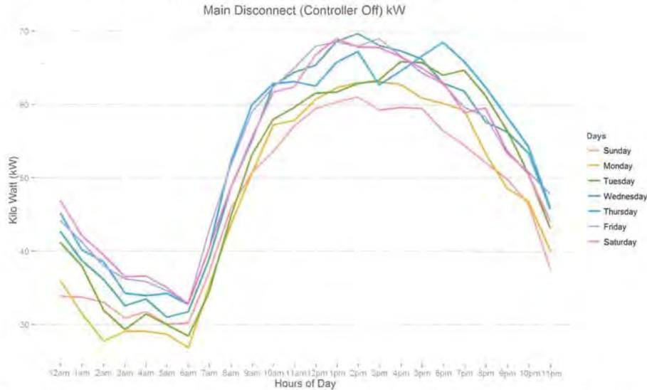
Figure 132: The figure above illustrates the average kWh draw of the main disconnect when the controller is OFF for each hour of the day and each day of the week. This is helpful in understanding the operation of the unit throughout the days of the week. It is clear that as the temperature increases throughout the day, so will the kWh draw.
