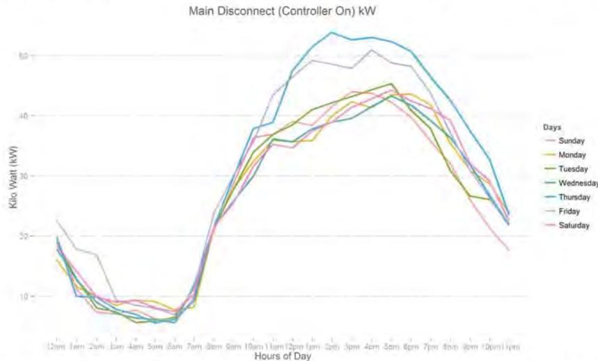
Figure 38: The figure above illustrates the average kWh draw of the main disconnect when the controller is ON for each hour of the day and each day of the week. This is helpful in understanding the operation of the unit throughout the days of the week. It is clear that as the temperature increases throughout the day, so will the kWh draw.
