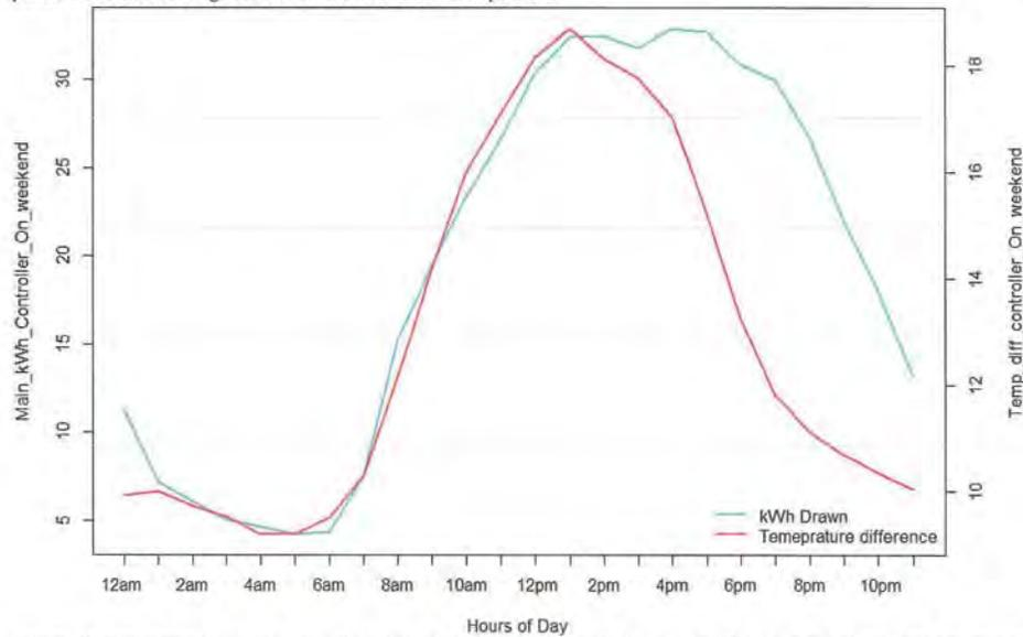
Figure 72: The figure above illustrates the relationship between the main disconnect kWh draw and the indoor and outdoor temperature difference when the controller is ON for the weekend hours (Saturday and Sunday). As it can be seen, as the temperature difference between indoor and outdoor temperature raises so does the kW consumption of the main disconnect panel. This indicates a high correlation between kW and temperature.
