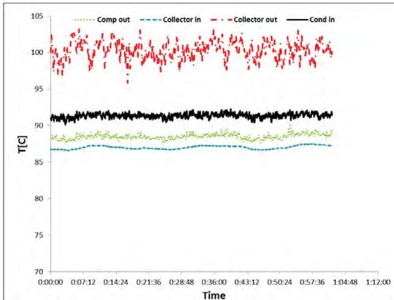
Figure 18: Solar test, refrigerant temperature profile between compressor outlet, solar collector inlet, solar collector outlet, and condenser inlet (CASE II)
