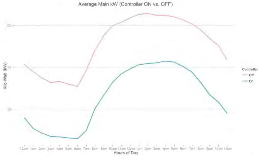
Figure 134: The plot above illustrates that there is a significant reduction in main kWh draw when the controller is ON versus when it is OFF. The kWh draw follows a similar trend throughout the day. This indicates that both control strategies are reacting to the outside temperature and super market occupancy.
