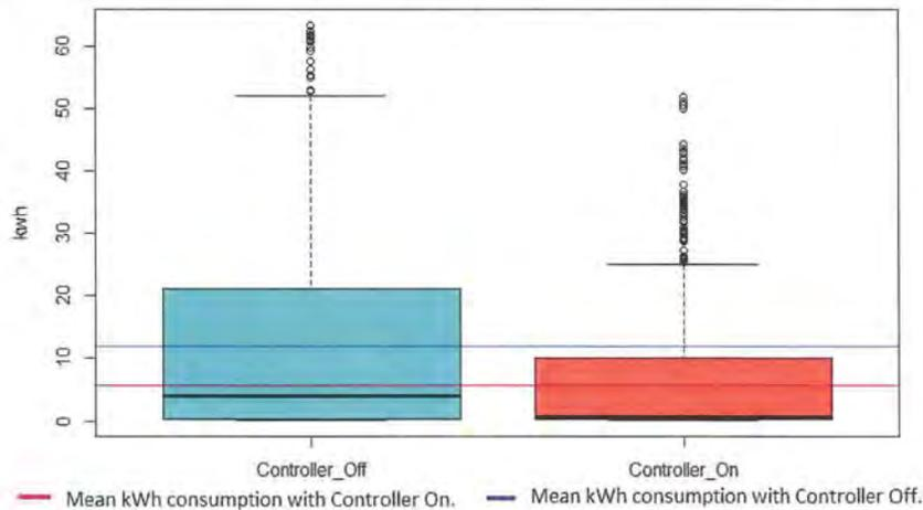
Figure 9: The Box Plot of the Compressor kWh and the Controller Status.
