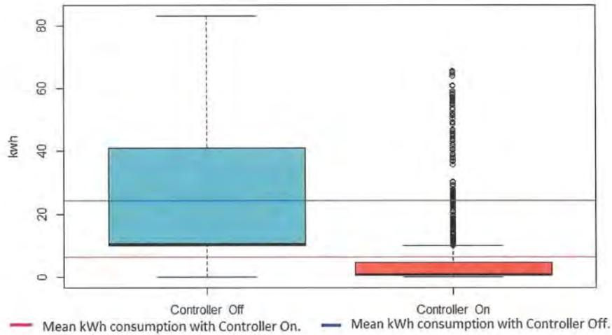
Figure 7: The Box Plot of the Main kWh and the Controller Status.
