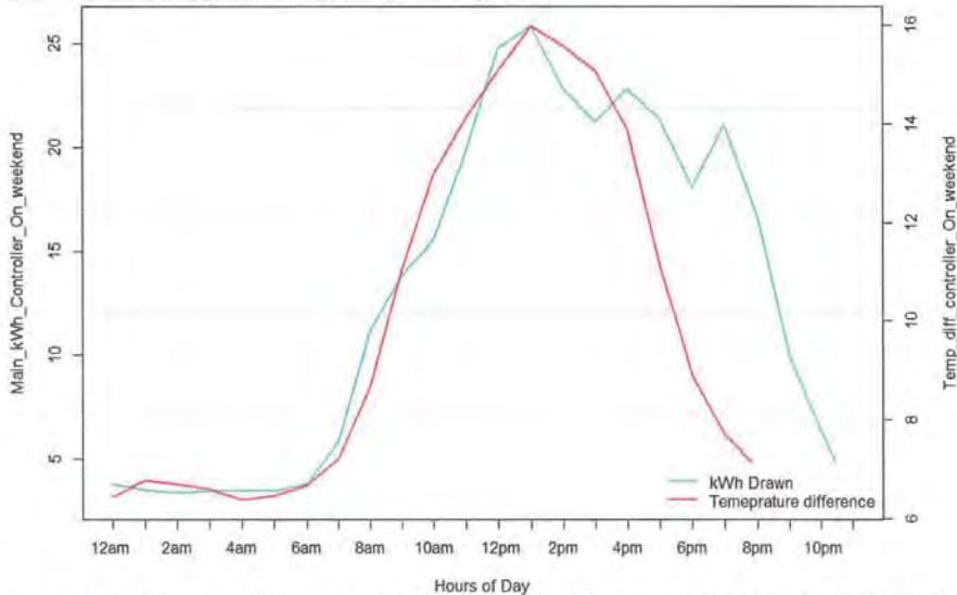
Figure 95: The figure above illustrates the relationship between the main disconnect kWh draw and the indoor and outdoor temperature difference when the controller is ON for the weekend hours (Saturday and Sunday). As it can be seen, as the temperature difference between indoor and outdoor temperature raises so does the kW consumption of the main disconnect panel. This indicates a high correlation between kW and temperature.
