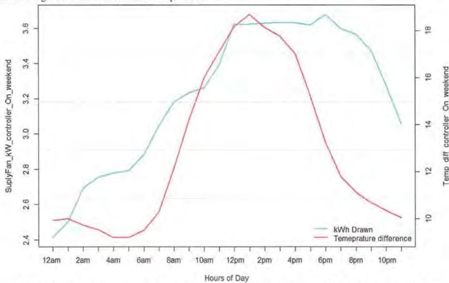
Figure 76: The figure above illustrates the relationship between the supply fan kWh draw and the indoor and outdoor temperature difference when the controller is ON for the weekend hours (Saturday and Sunday). As it can be seen, as the temperature difference between indoor and outdoor temperature raises so does the kW consumption of the main disconnect panel. This indicates a high correlation between kW and temperature.
