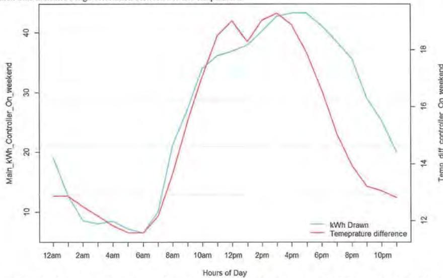
Figure 48: The figure above illustrates the relationship between the main disconnect kWh draw and the indoor and outdoor temperature difference when the controller is ON for the weekend hours (Saturday and Sunday). As it can be seen, as the temperature difference between indoor and outdoor temperature raises so does the kW consumption of the main disconnect panel. This indicates a high correlation between kW and temperature.
