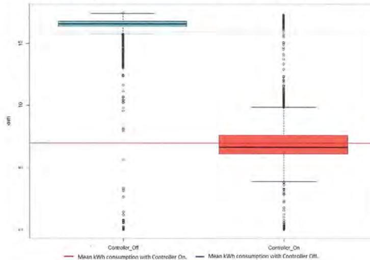
Figure 130: The Box Plot of the Supply Fan kWh and the Controller Status.
