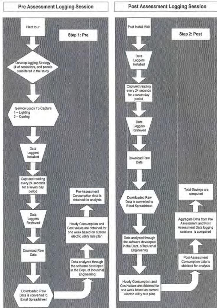
Figure 6. The Measuring & Verification Methodology
