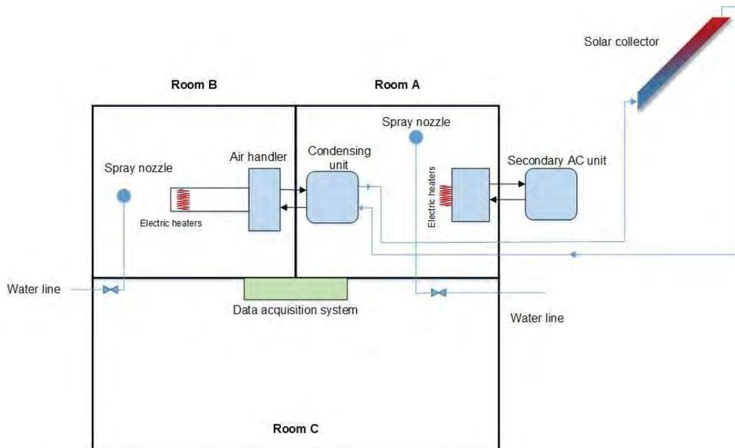
Schematic diagram of the test facility and the installed equipment
