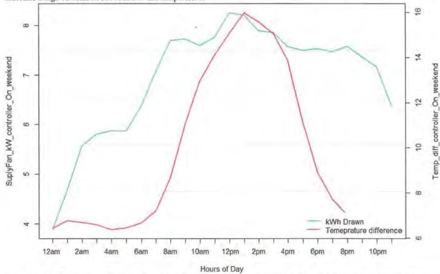
Figure 99: The figure above illustrates the relationship between the supply fan kWh draw and the indoor and outdoor temperature difference when the controller is ON for the weekend hours (Saturday and Sunday). As it can be seen, as the temperature difference between indoor and outdoor temperature raises so does the kW consumption of the main disconnect panel. This indicates a high correlation between kW and temperature.
