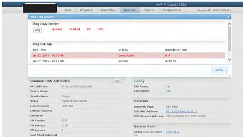
Ping [REDACTED] Switch S/N 1800163 MAC ID 00135003003D3611 after restoring power connection.
