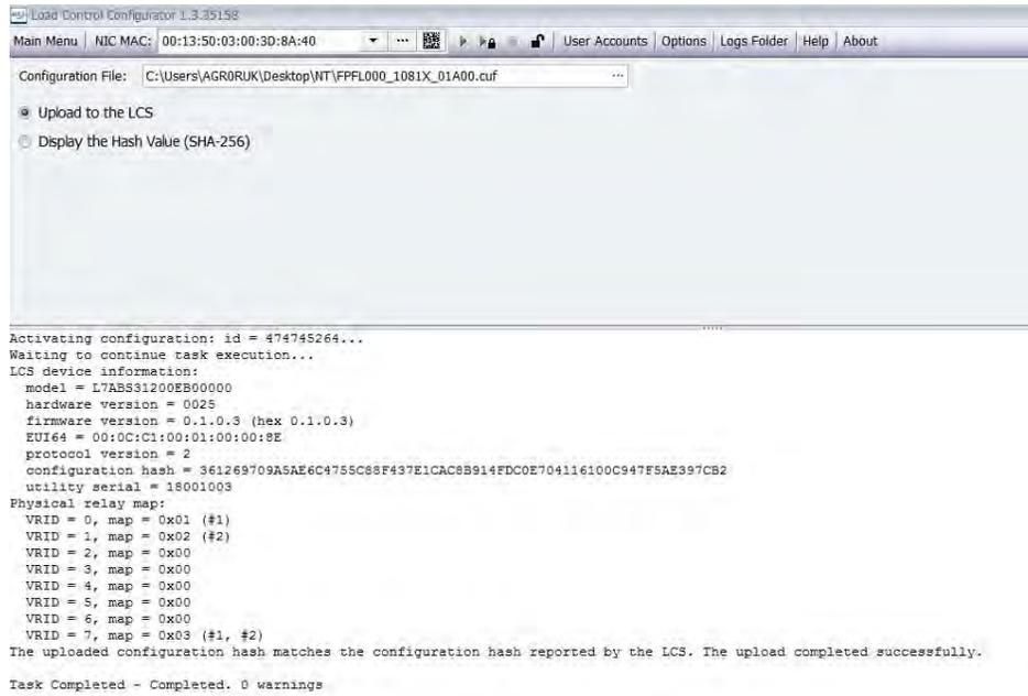
The screenshot shows the 'Load Control Configurator 1.3.25158' application window. The title bar includes 'Main Menu', 'NIC MAC: 00:13:50:03:00:30:8A:40', and standard window controls. The configuration file path is 'C:\Users\AGRORUK\Desktop\NT\FPFL000\_1081X\_01A00.cuf'. Two radio buttons are visible: 'Upload to the LCS' (selected) and 'Display the Hash Value (SHA-256)'. The main area displays the following text:
