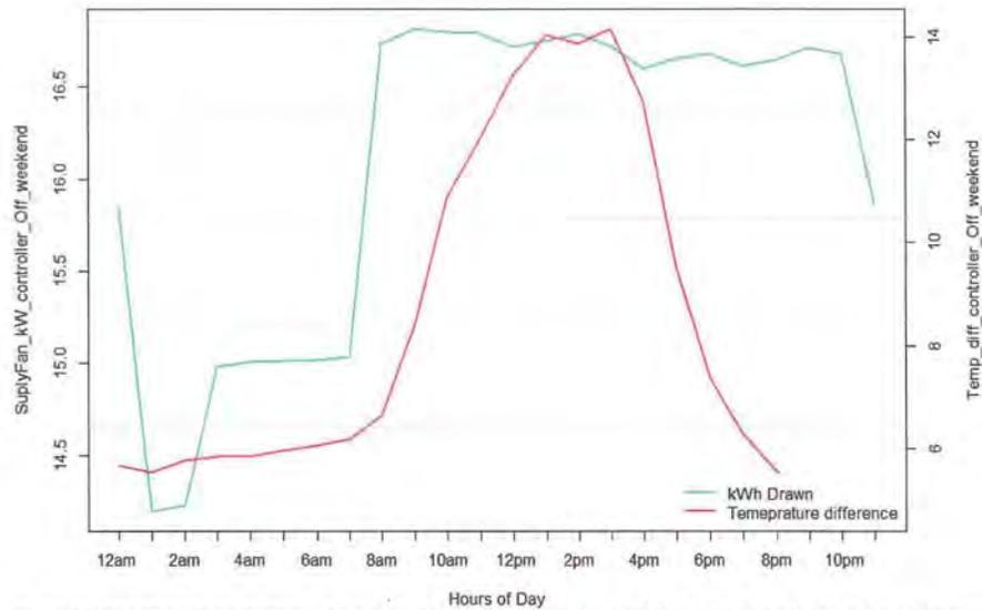
Figure 98: The figure above illustrates the relationship between the supply fan kWh draw and the indoor and outdoor temperature difference when the controller is OFF for the weekend hours (Saturday and Sunday). As it can be seen, as the temperature difference between indoor and outdoor temperature increased so does the kW consumption of the main disconnect panel. This indicates a high correlation between kW and temperature.
