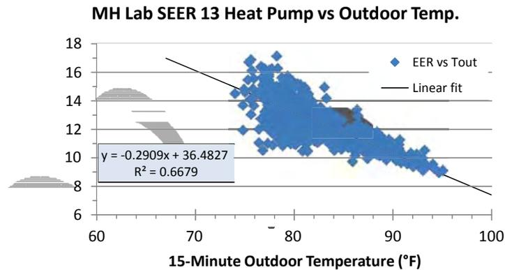
Figure 12. Measured cooling EER for the central ducted 3-ton SEER 13 Lab heat pump as a function outdoor temperature. Duct losses are not considered when calculating EER.
