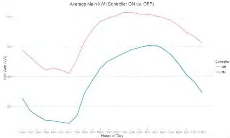
Figure 110: Illustrates that there is a significant reduction in main kWh draw when the controller is ON versus when it is OFF. The kWh draw follows a similar trend throughout the day. This indicates that both control strategies are reacting to the outside temperature and super market occupancy.
