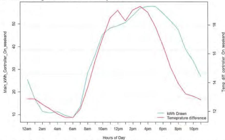
Figure 119: The figure above illustrates the relationship between the main disconnect kWh draw and the indoor and outdoor temperature difference when the controller is ON for the weekend hours (Saturday and Sunday). As it can be seen, as the temperature difference between indoor and outdoor temperature raises so does the kW consumption of the main disconnect panel. This indicates a high correlation between kW and temperature.
