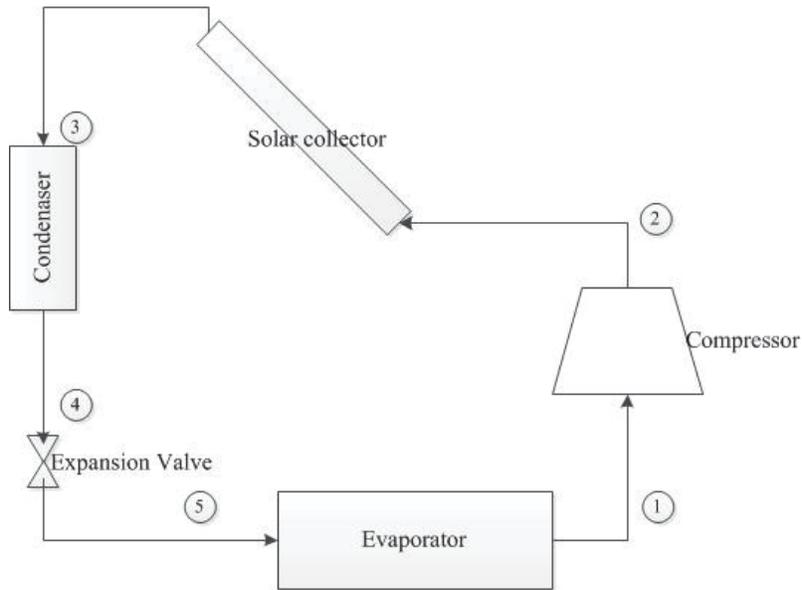
Figure 21: Schematic of the [redacted] solar assisted AC unit
