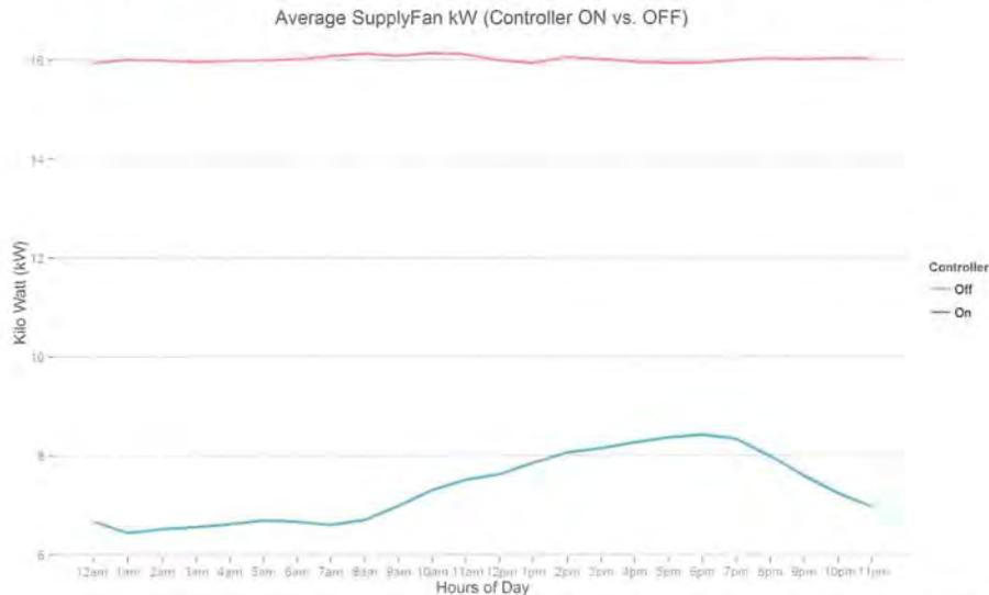
Figure 117: Figure above illustrates that there is a significant reduction in supply fan kWh draw when the controller is ON versus when it is OFF. The kWh draw follows a similar trend throughout the day. This indicates that both control strategies are reacting to the outside temperature and super market occupancy.
