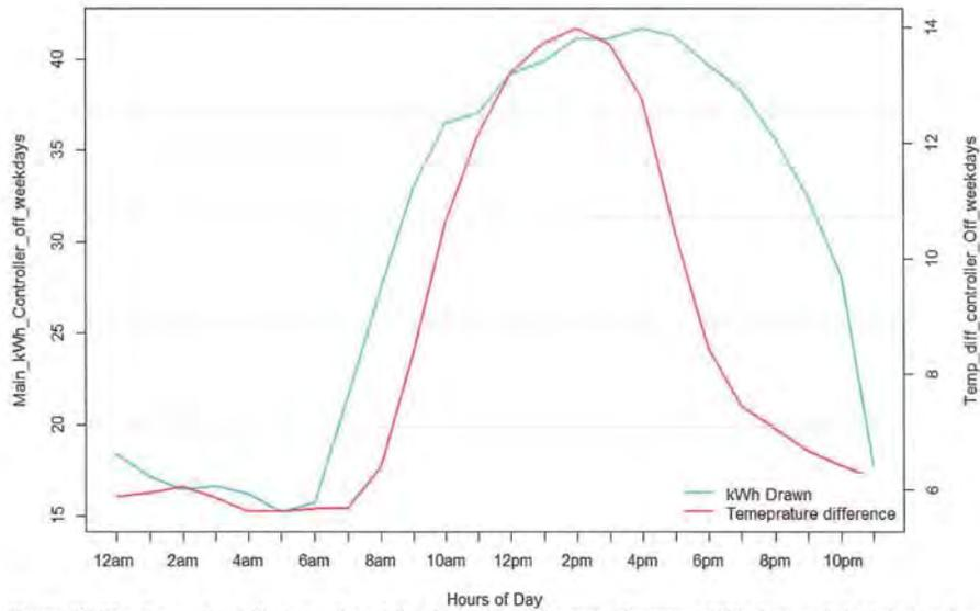
Figure 96: The figure above illustrates the relationship between the main disconnect kWh draw and the indoor and outdoor temperature difference when the controller is OFF for the weekday hours (Monday to Friday). As it can be seen, as the temperature difference between indoor and outdoor temperature increased so does the kW consumption of the main disconnect panel. This indicates a high correlation between kW and temperature.
