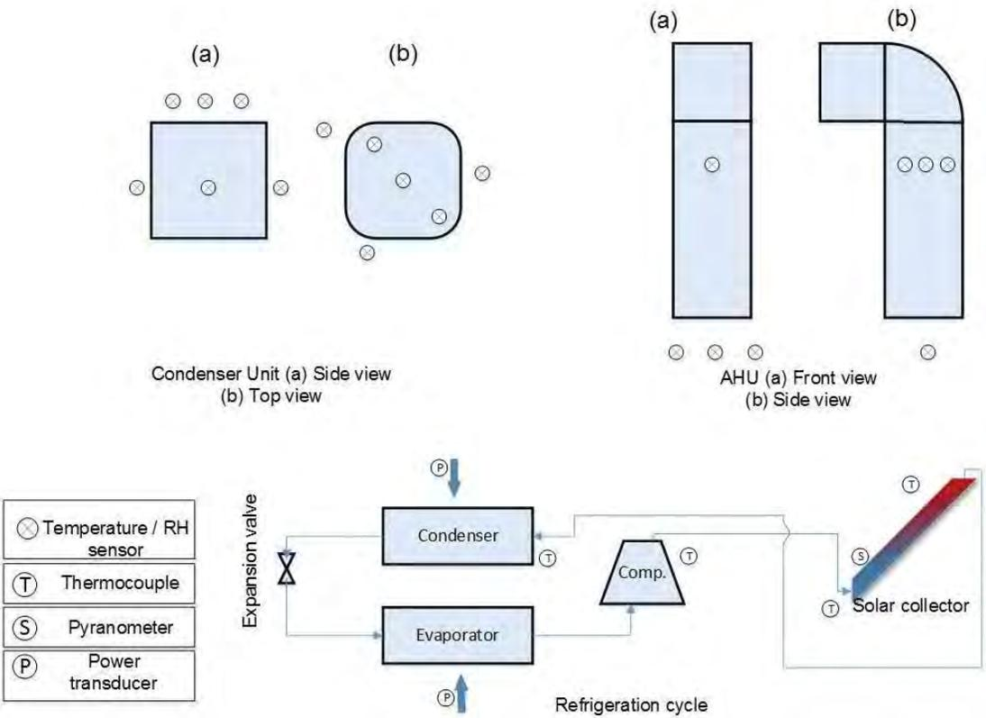
Figure 3: Locations of the sensors for monitoring the unit under test
