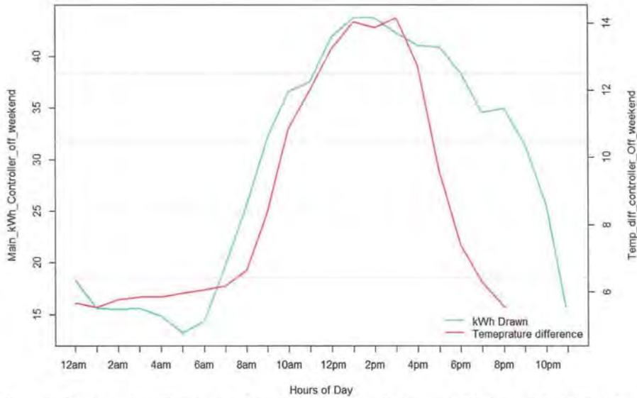
Figure 94: The figure above illustrates the relationship between the main disconnect kWh draw and the indoor and outdoor temperature difference when the controller is OFF for the weekend hours (Saturday and Sunday). As it can be seen, as the temperature difference between indoor and outdoor temperature increased so does the kW consumption of the main disconnect panel. This indicates a high correlation between kW and temperature.
