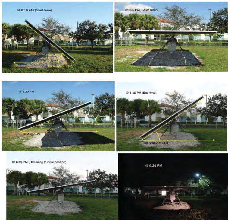
The single-axis tracker starts in the morning with a tilt angle of about 45° facing 15 degrees South of East and completes its daily path with a tilt angle of about 45° facing 15 degrees North of West. It has a broad turn range (0 to 90°) and remains flat with tilt angle of zero degree during night.
