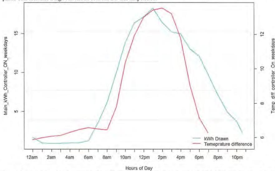
Figure 97: The figure above illustrates the relationship between the main disconnect kWh draw and the indoor and outdoor temperature difference when the controller is ON for the weekday hours (Monday to Friday). As it can be seen, as the temperature difference between indoor and outdoor temperature raises so does the kW consumption of the main disconnect panel. This indicates a high correlation between kW and temperature.
