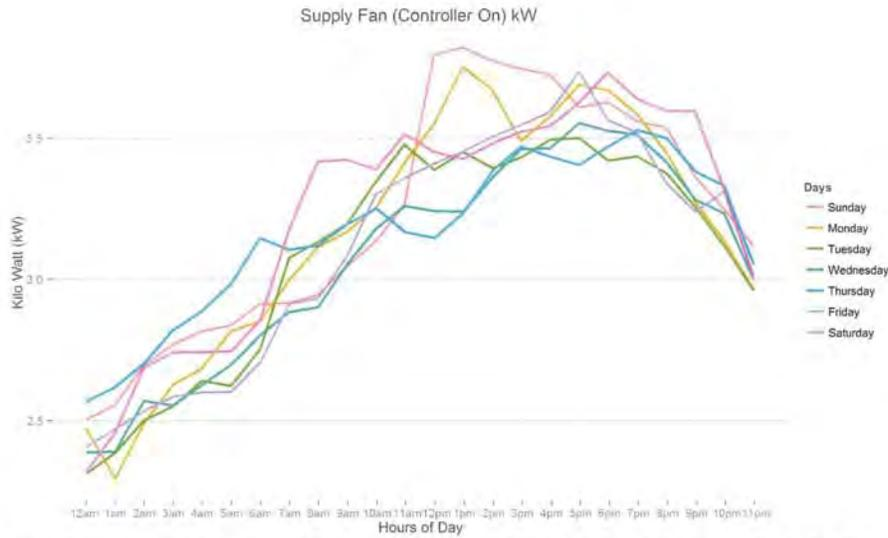
Figure 67: The figure above illustrates the average kWh draw of the supply fan when the controller is ON for each hour of the day and each day of the week. This is helpful in understanding the operation of the unit throughout the days of the week. It is clear that as the temperature increases throughout the day, so will the kWh draw.
