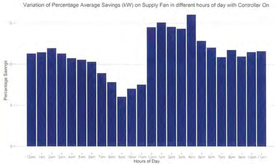
Figure 45: The figure above illustrates the average percent savings of the supply fan throughout the day. As it can be seen, savings are higher during the cooler parts of the day as the VFD is able to slow down the speed of the fan for longer periods of time.
