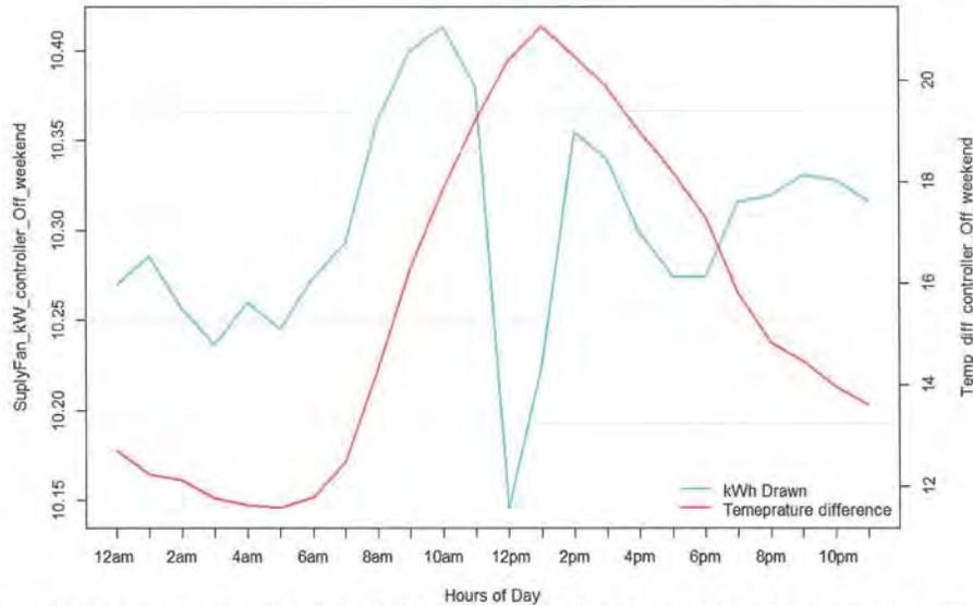
Figure 51: The figure above illustrates the relationship between the supply fan kWh draw and the indoor and outdoor temperature difference when the controller is OFF for the weekend hours (Saturday and Sunday). As it can be seen, as the temperature difference between indoor and outdoor temperature increased so does the kW consumption of the main disconnect panel. This indicates a high correlation between kW and temperature.
