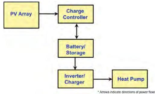
Figure 25. "As-tested" Stand-Alone Solar Heat Pump System
