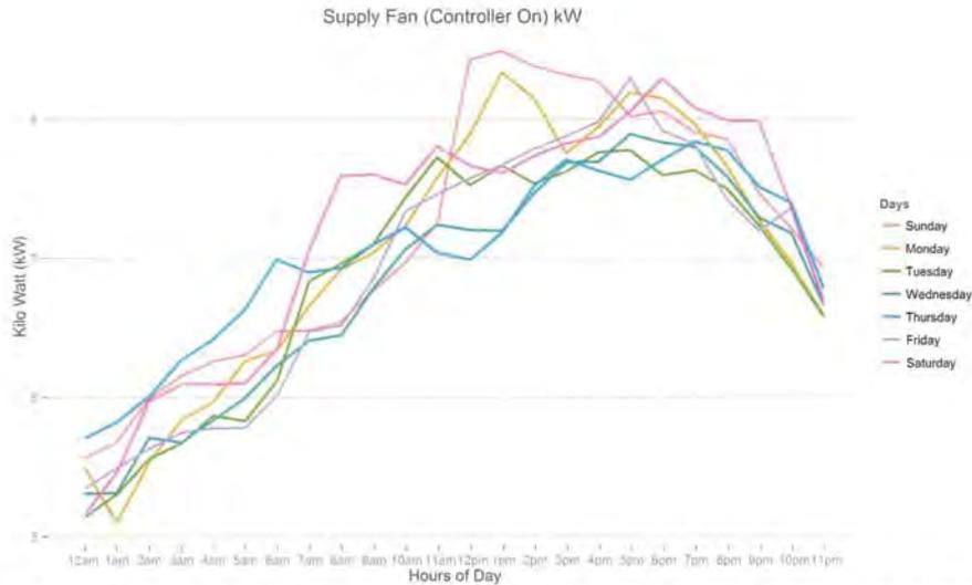
Figure 138: The figure above illustrates the average kWh draw of the supply fan when the controller is ON for each hour of the day and each day of the week. This is helpful in understanding the operation of the unit throughout the days of the week. It is clear that as the temperature increases throughout the day, so will the kWh draw.
