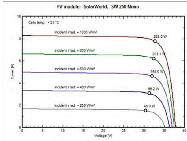
Figure 2. [REDACTED] I\_V Curves at 25°C cell temperature.
