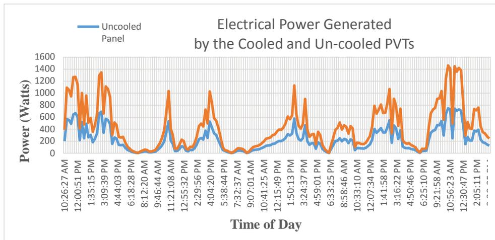
**Figure 1.1:** Electrical power generated by the cooled and un-cooled PVTs for a period of 5 days in 9/21/2014 – 9/26/2014.
