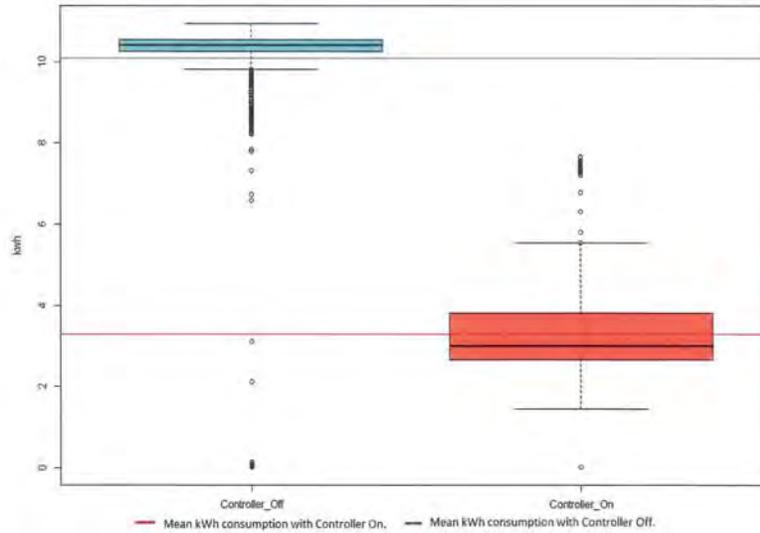
Figure 59: The Box Plot of the Supply Fan kWh and the Controller Status.
