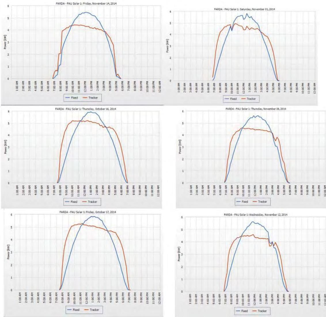
The diagrams show the non-symmetric nature of the tracker output as caused by the 15 degree deviation from the North-South axis. The following graphs show the total daily generation shown as the blue colored area in the first graph, versus the individual outputs for tracker versus non-tracker outputs shown in the second graph.
