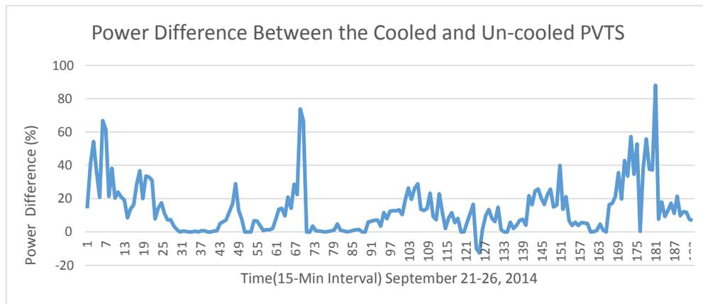
**Figure 3-2:** The difference between the power generated by the cooled and uncooled PVTs in the same time period for Figure 3-1.
