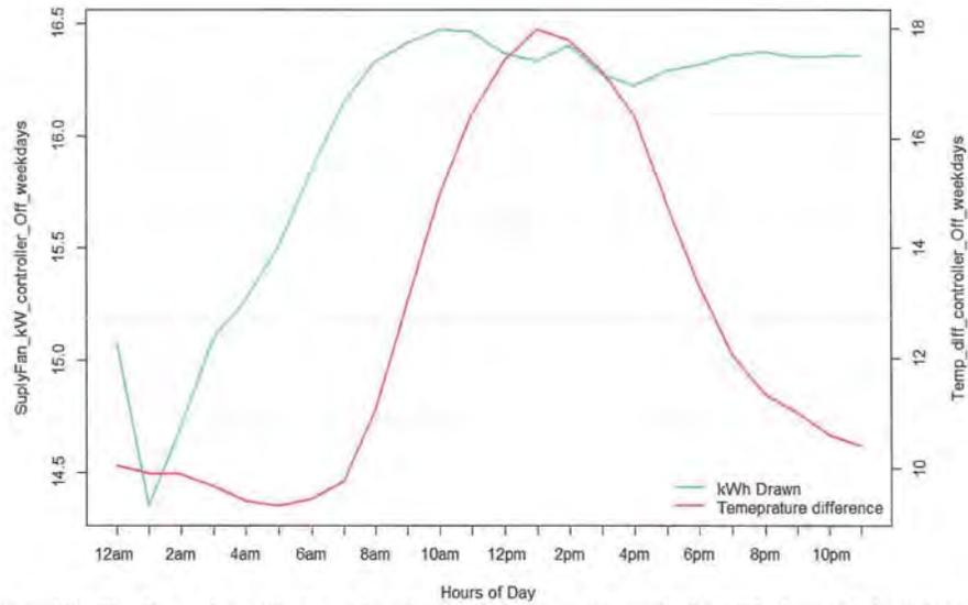
Figure 148: The figure above illustrates the relationship between the supply fan kWh draw and the indoor and outdoor temperature difference when the controller is OFF for the weekday hours (Monday to Friday). As it can be seen, as the temperature difference between indoor and outdoor temperature increased so does the kW consumption of the main disconnect panel. This indicates a high correlation between kW and temperature.
