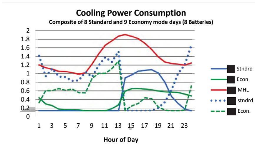
**Figure 15.** Twenty-four hour cooling power consumption profile for Standard and Economy mini-split operation when using 8 batteries, plus cooling power consumption for the Lab SEER 13 central system. Figure 15 has added economy profile to Figure 14.
