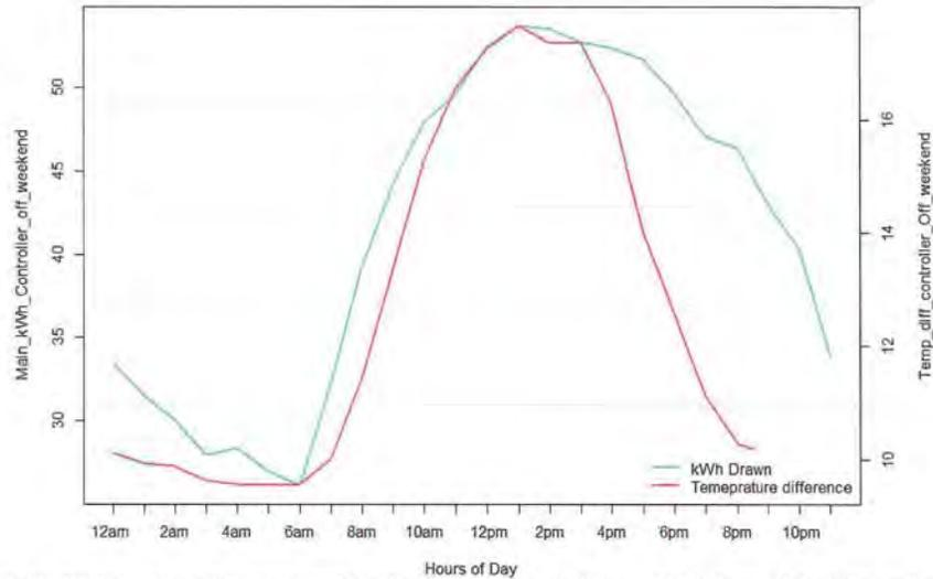
Figure 71: The figure above illustrates the relationship between the main disconnect kWh draw and the indoor and outdoor temperature difference when the controller is OFF for the weekend hours (Saturday and Sunday). As it can be seen, as the temperature difference between indoor and outdoor temperature increased so does the kW consumption of the main disconnect panel. This indicates a high correlation between kW and temperature.
