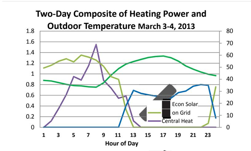
**Figure 21.** Twenty-four hour composite of solar heat pump operation on a cold two-day period, showing heating power for the mini-split operating on solar (blue line) and on the grid (olive green line), and heating power for the central 5-ton system (purple line).
