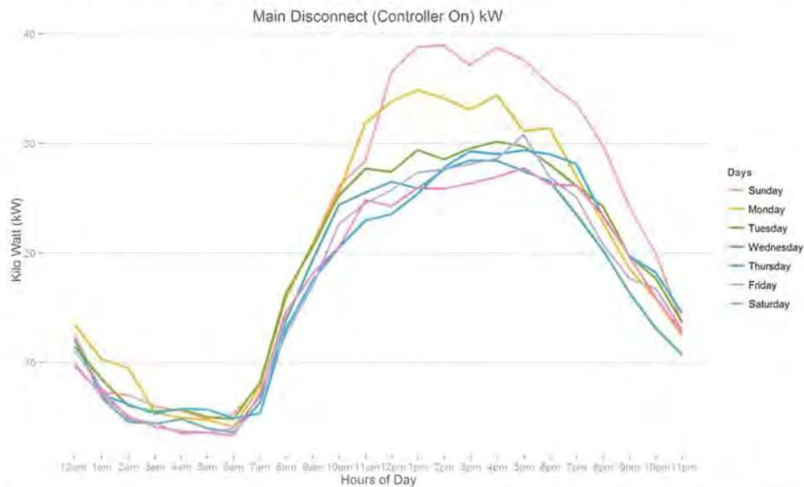
Figure 62: The figure above illustrates the average kWh draw of the main disconnect when the controller is ON for each hour of the day and each day of the week. This is helpful in understanding the operation of the unit throughout the days of the week. It is clear that as the temperature increases throughout the day, so will the kWh draw.
