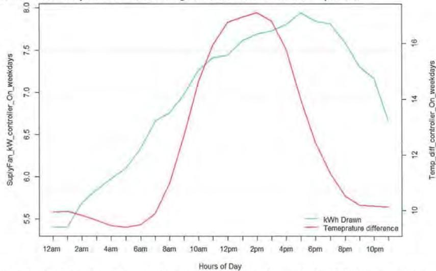
Figure 149: The figure above illustrates the relationship between the supply fan kWh draw and the indoor and outdoor temperature difference when the controller is ON for the weekday hours (Monday to Friday). As it can be seen, as the temperature difference between indoor and outdoor temperature raises so does the kW consumption of the main disconnect panel. This indicates a high correlation between kW and temperature.
