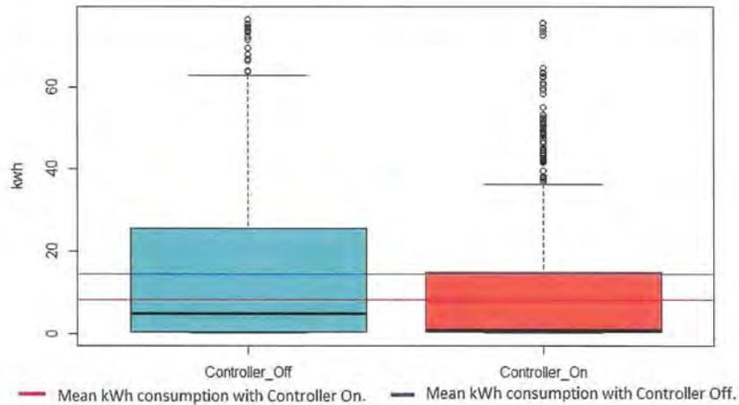
Figure 81: The Box Plot of the Compressor kWh and the Controller Status.
