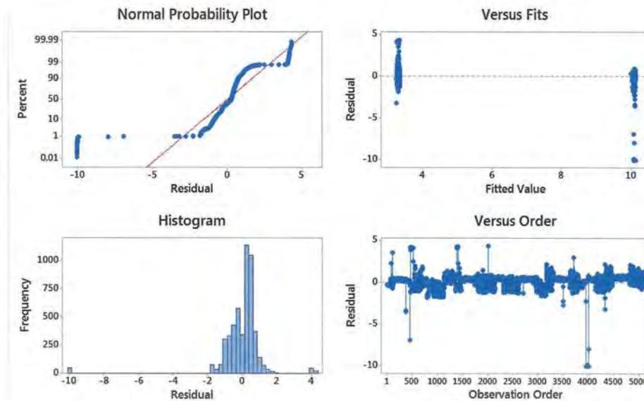
Figure 36: Residual Plots for Supply Fan kWh
