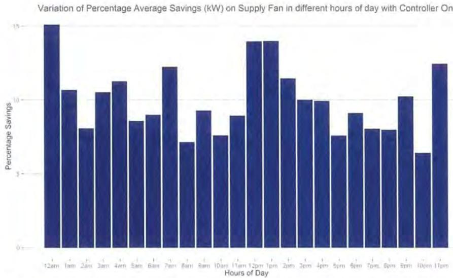
Figure 140: The figure above illustrates the average percent savings of the supply fan throughout the day. As it can be seen, savings are higher during the cooler parts of the day as the VFD is able to slow down the speed of the fan for longer periods of time.
