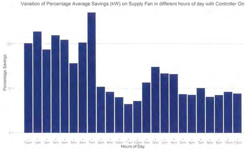
Figure 21: The figure above illustrates the average percent savings of the supply fan throughout the day. As it can be seen, savings are higher during the cooler parts of the day as the VFD is able to slow down the speed of the fan for longer periods of time.
