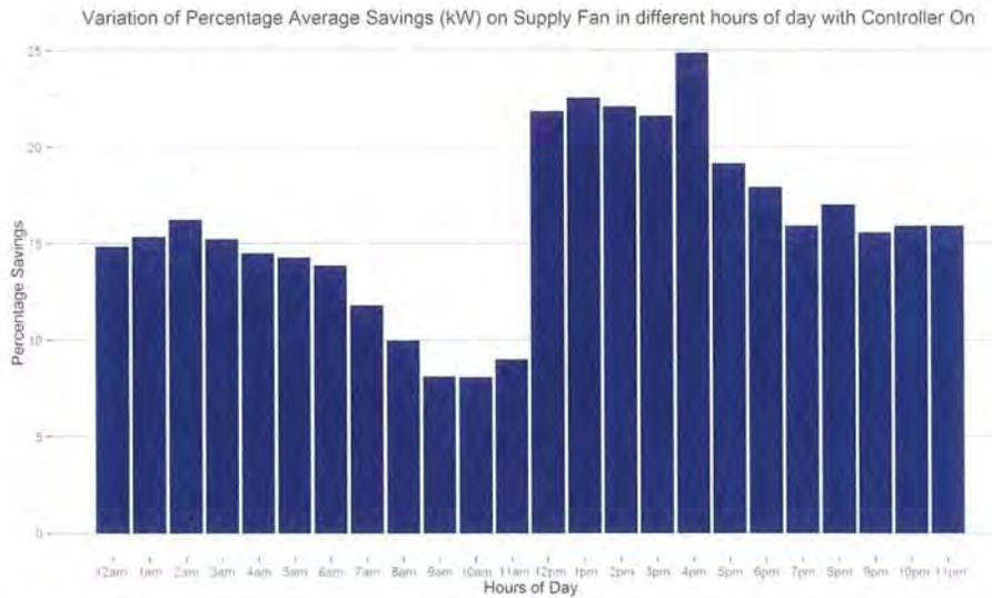
Figure 116: The figure above illustrates the average percent savings of the supply fan throughout the day. As it can be seen, savings are higher during the cooler parts of the day as the VFD is able to slow down the speed of the fan for longer periods of time.
