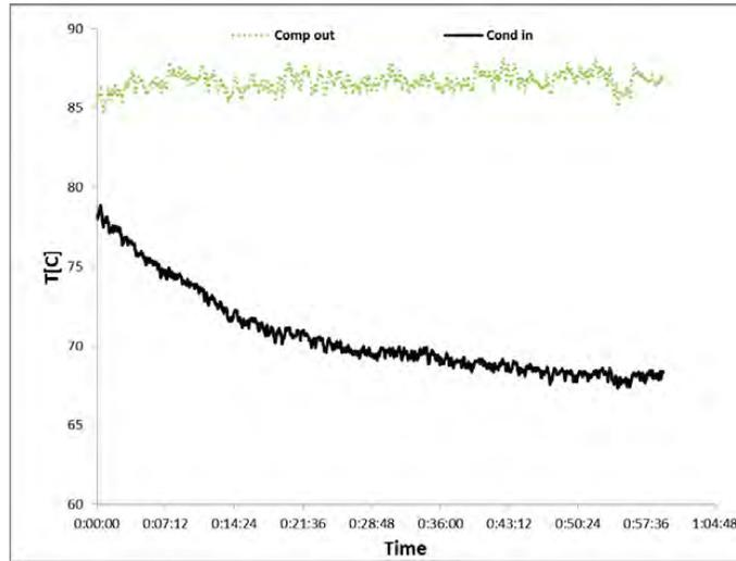
Figure 13: Solar test, refrigerant temperature profile between compressor outlet and condenser inlet (CASE I)
