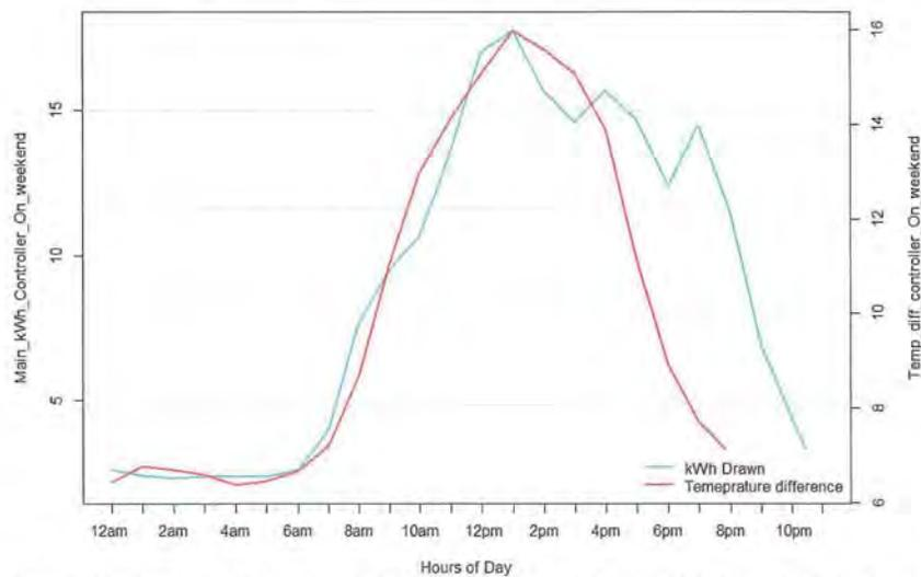
Figure 24: The figure above illustrates the relationship between the main disconnect kWh draw and the indoor and outdoor temperature difference when the controller is ON for the weekend hours (Saturday and Sunday). As it can be seen, as the temperature difference between indoor and outdoor temperature raises so does the kW consumption of the main disconnect panel. This indicates a high correlation between kW and temperature.
