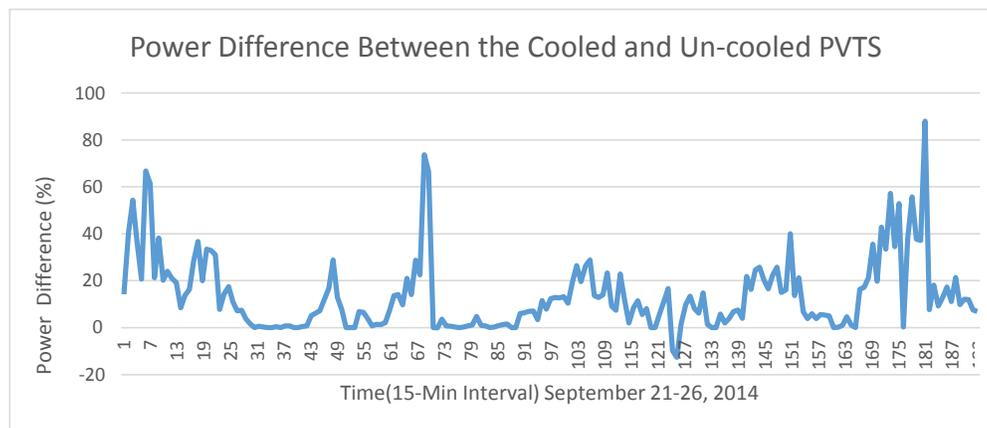
**Figure 1.2:** The difference between the power generated by the cooled and uncooled PVTs in the same time period for Figure 1.1.
