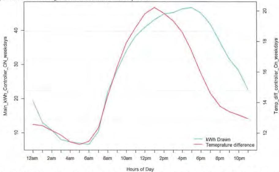
Figure 50: The figure above illustrates the relationship between the main disconnect kWh draw and the indoor and outdoor temperature difference when the controller is ON for the weekday hours (Monday to Friday). As it can be seen, as the temperature difference between indoor and outdoor temperature raises so does the kW consumption of the main disconnect panel. This indicates a high correlation between kW and temperature.
