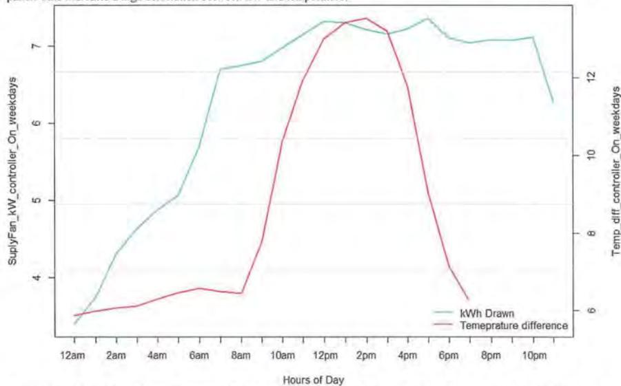
Figure 101: The figure above illustrates the relationship between the supply fan kWh draw and the indoor and outdoor temperature difference when the controller is ON for the weekday hours (Monday to Friday). As it can be seen, as the temperature difference between indoor and outdoor temperature raises so does the kW consumption of the main disconnect panel. This indicates a high correlation between kW and temperature.
