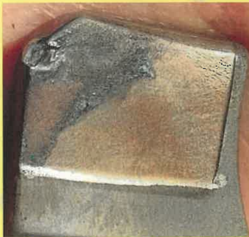
Figure 4 -- Photo of an L-0 blade Z-Lock from Period 5 Showing Contact Surface Wear
