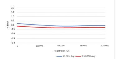
The accelerated life test of Intelis is stable and the open (250 CFH) and check (50 CFH) track tightly.
