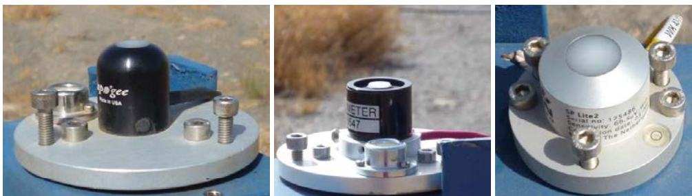
Figure 3-11. Selected photodiode sensors with different diffuser geometries. Photos from Stefan Wilbert, DLR
