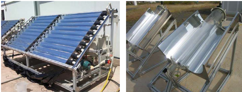
Figure 8-12. CPC photo-reactors installed at PSA for solar water disinfection applications: (left) CPC-SODIS, (right) FITOSOL-2. (Source: PSA, CIEMAT http://www.psa.es/en/instalaciones/aguas.php )
