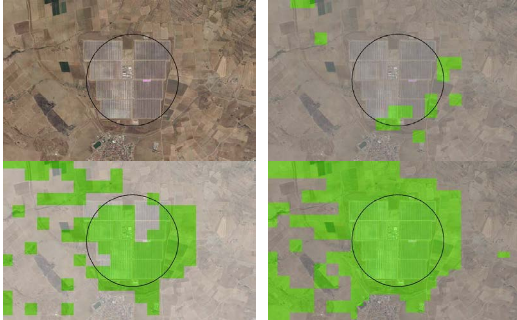
Figure 8-5. Buffer around the Orellana STE plant (Spain) and the suitable areas by the LRS1 (upper right), LRS2 (bottom left), and LRS3 (bottom right) methodologies with maximum slopes of 1%, 2%, and 3 %. Suitable zones are shown in green (Navarro et al. 2016)
