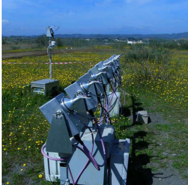
Figure 3-17. RSI calibration station at Plataforma Solar de Almería. Photo from Stefan Wilbert, DLR
