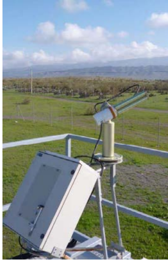
Figure 3-21. AERONET sun photometric station at the Plataforma Solar de Almería. Photo from DLR
