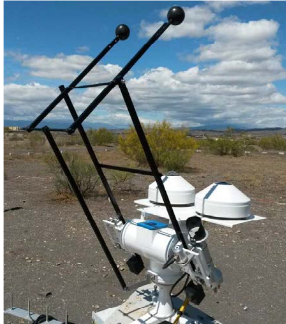
Figure 3-4. Pyrheliometer, a shaded pyranometer and a shaded pyrgeometer mounted on an automatic solar tracker. Photo from DLR
