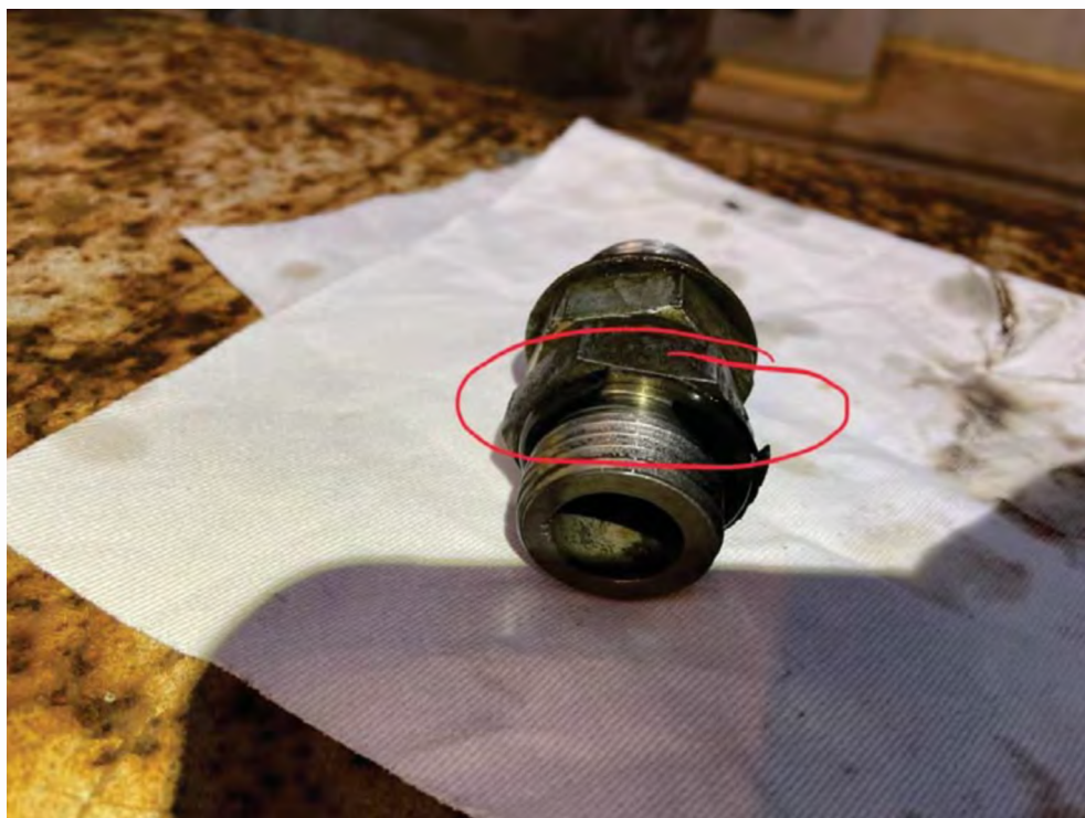
Figure 2 Original damaged o-ring
