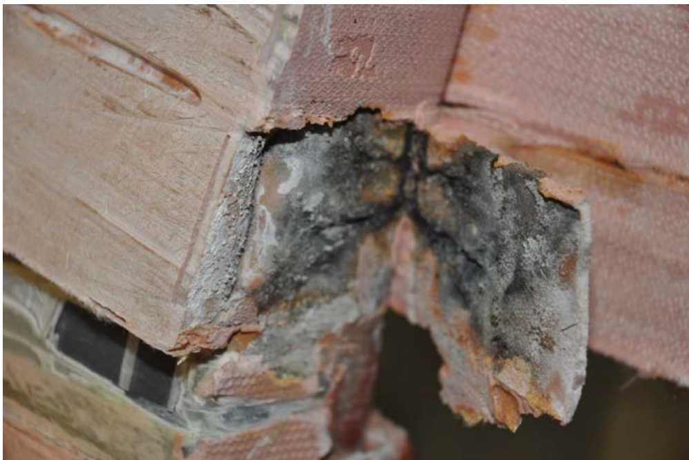
Figure 8. Spacer Banding Partially Removed, Showing the Assessed Fault Location
