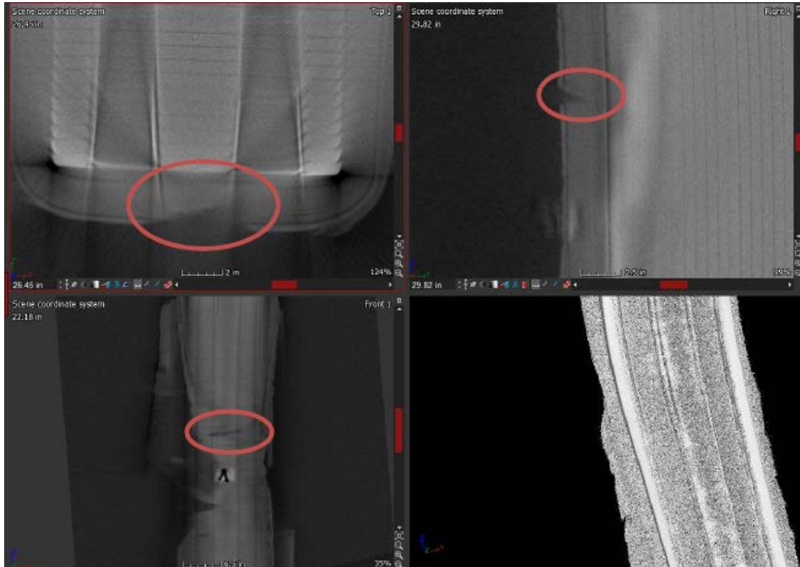
Figure 10. CT Image of the Assessed Fault Location
