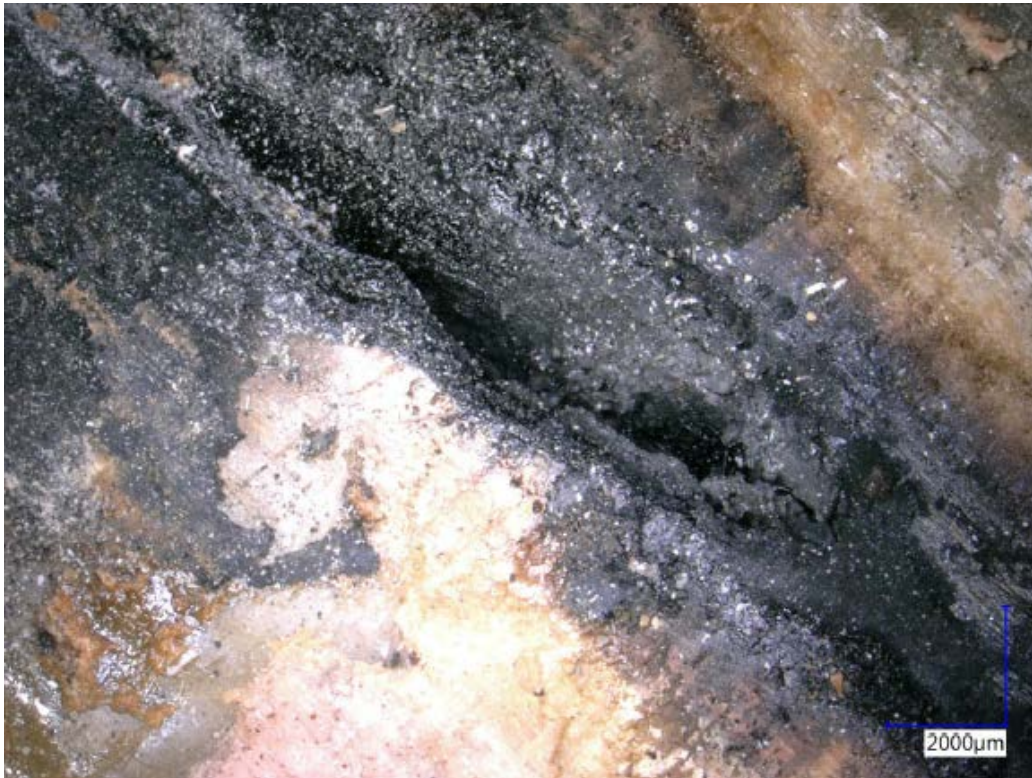
Figure 9. Assessed Fault Location, Microscope View
