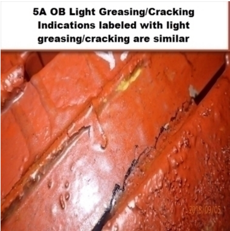
2.6 Turbine End Tuning Weight Inspection Very Light Greasing and Cracking
