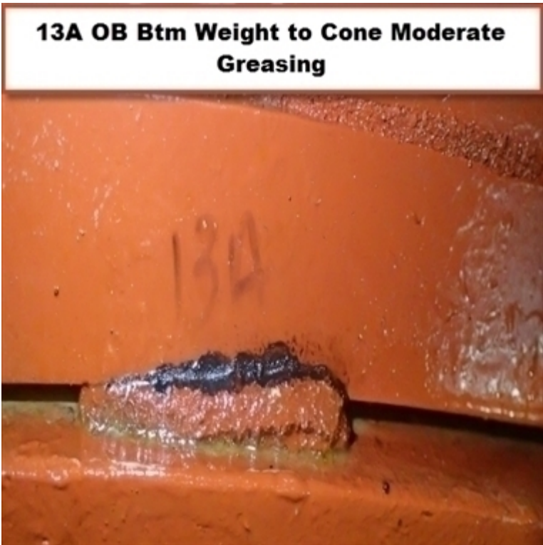
2.4 Turbine End Tuning Weight Inspection Weight to Cone Moderate Greasing
