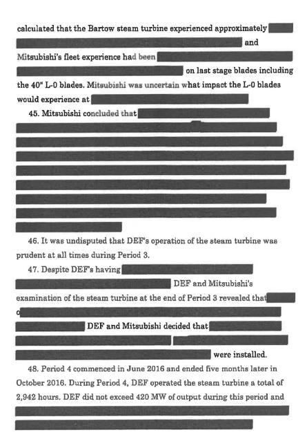
49. Just five months after the commencement of Period 4, DEF detected vibration changes in the LP turbine and stopped operation of the steam turbine to inspect the L-0 blades. During this inspection, DEF and Mitsubishi once again found several damaged L-0 blades. At the time of this blade damage, DEF was operating the steam turbine below 420 MW and observing the operating parameters established by Mitsubishi
