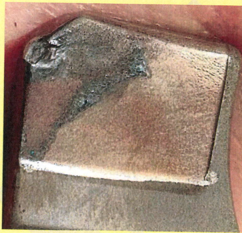
Figure 4 -- Photo of an L-O blade Z-Lock from Period 5 Showing Contact Surface Wear
