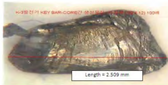
Particles from KoRi generator [lo carbon steel]
