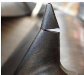
Failed stub #54 Blade.
