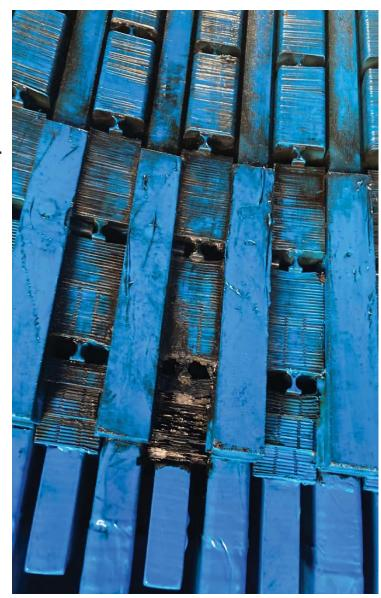
Stator Core Iron at 9 o'clock
