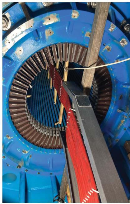
Damaged Ground Wall Insulation, Top Bar Slot 20
