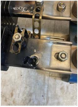
After discovering that the Generator Heaters were shorted, we went back to the drawings. We started to compare what was done in the field to the OEM GE drawing 108E7884. After reviewing the GE OEM Dwg and comparing it to the field de-term sheet we noticed that the 480V supply was parallel to all the heaters rather than in a series – parallel circuit causing them ALL to fail.
