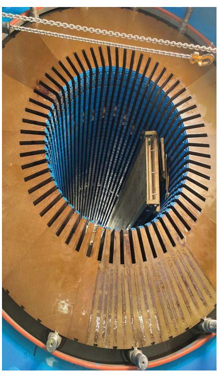
Broken Iron Lamination and Inside Spacer Block
