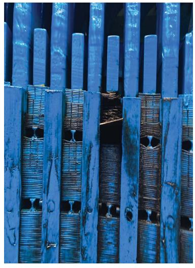
Stator Core at 1 o'clock, Greasing Removed
