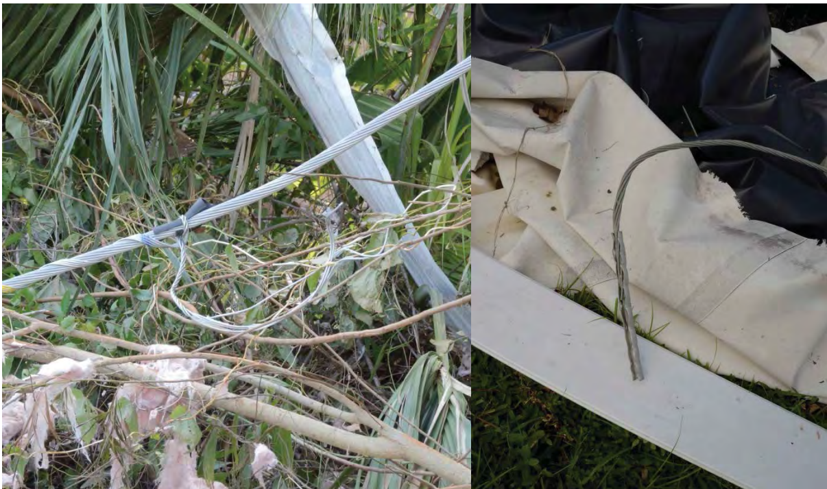
Insulator tie and failed splice. Below: ALS out of support and on ground
