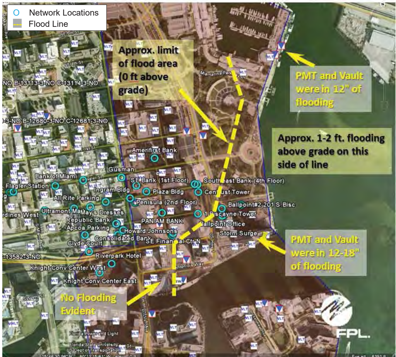
Exhibit 1: Flood intrusion into the Distribution Equipment in Miami
