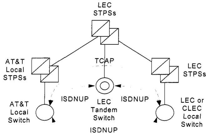
**Figure 4. Interswitch TCAP Signaling for SS7 Network Interconnection
