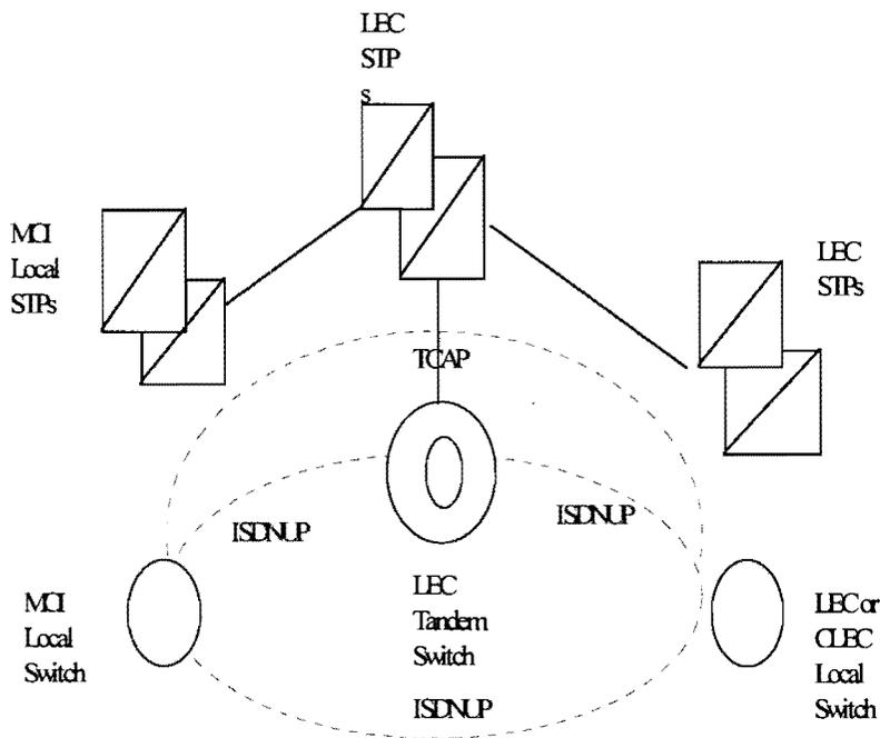
FIGURE 9. Interswitch TCAP Signaling for SS7 Network Interconnection
