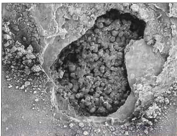
This pit (top), with the tubercle cap still in place, is typical of the Mission system in Texas. The scanning electron micrograph (bottom) shows the pitting structures underlying the tubercle caps.
