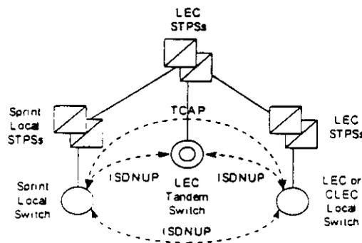
**Figure 10. Interswitch TCAP Signaling for SS7 Network Interconnection**
