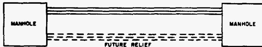
Figure 1a. Conduit Formation of Two to Four Vertical Rows and Duct Requirements Are Greater Than Racking Capacity of One Side of Manhole.
