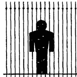
A person standing in a magnetic field (blue lines) showing induced current (white dashed lines).
