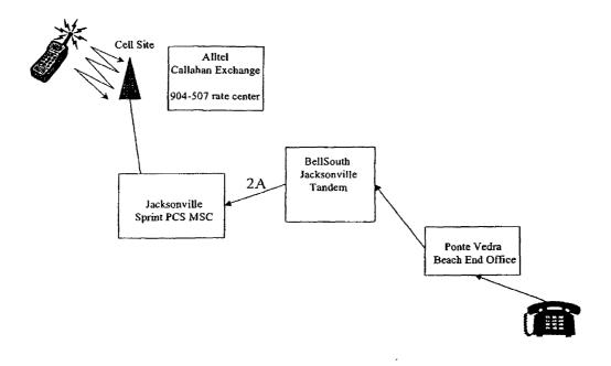
According to BellSouth's "new" and "revised" interconnection policy, because the Sprint 904-507 code is rated in the Callahan exchange, BellSouth's tandem switch should instead route the call to ALLTEL's end office switch in Callahan – even though no ALLTEL customer is involved
