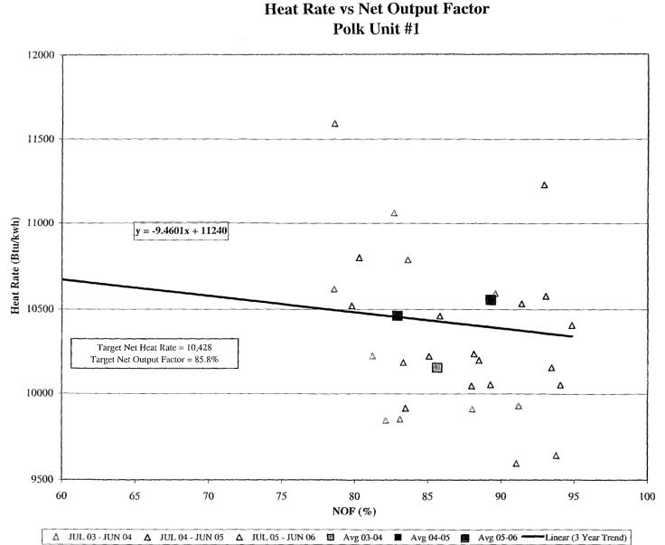
**Tampa Electric Company** Heat Rate vs Net Output Factor
