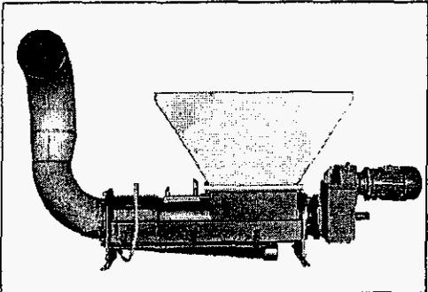
Left Below: Here you see a Model EWP 250/600 Washing Press with an inlet hopper and discharge pipe. The inlet hopper can be directly connected to a primary screening device such as a Mensch Crawler™ Bar Screen or Stair Screen, or can be fed by a conveyor. The discharge pipe can be fitted with a bagging assembly, or feed directly into a receiving container.
