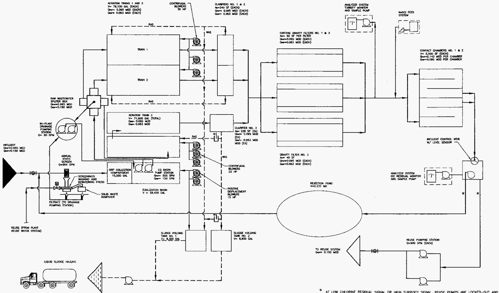
\* AT LOW CHLORINE RESIDUAL SIGNAL OR HIGH TURBIDITY SIGNAL, REUSE PUMPS ARE LOCKED-OUT AND TRANSFER PUMPS TO REJECT POND ARE ENERGIZED. NORMAL OPERATION IS MANUALLY RESET WHEN
