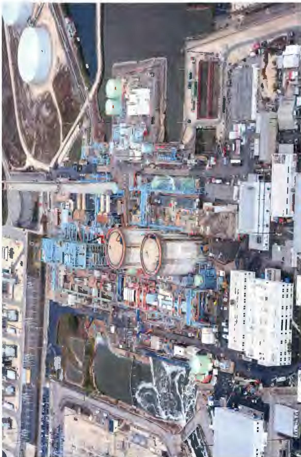
Turkey Point Units 3 and 4 use approximately 1,300,000 gallons per minute of cooling water which enters from the right and exits on the left side to support the generation of over 1,700 MWe which required the replacement of many major components.
