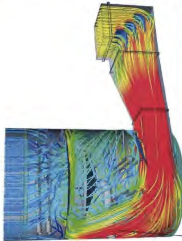
Tangential Inlet Forces High Velocity Gas Along Back Wall, Reducing the Minimum Gas Residence Time in the Quench Loop
