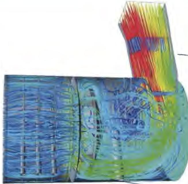
Significant Reduction in Maximum Velocity Along Back Wall
