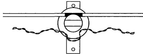
STEP 2: ALIGN THE EZ-WRAP SIDE TIE WITH THE CONDUCTOR. MAKE SURE THE TIE LOOP OF THE EZ-WRAP SIDE TIE IS FACING AWAY FROM THE CONDUCTOR AS SHOWN.
