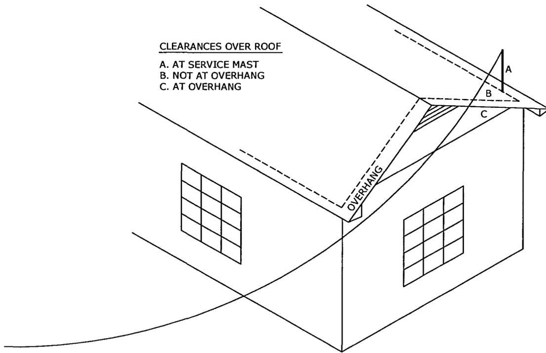
1. VERTICAL CLEARANCES OF NEW SERVICES TO BUILDINGS AT LOCATIONS A, B, AND C AS SHOWN ABOVE MUST MEET THE FOLLOWING MINIMUM CLEARANCES FOR THE HIGHEST VOLTAGE BETWEEN ANY TWO CONDUCTORS.
