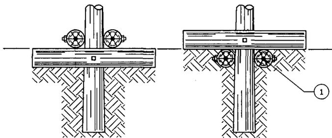
BOG SHOES SHOULD BE USED IN SOFT OR SWAMPY GROUND WHERE POLES MIGHT SETTLE EXCESSIVELY. SHOES ARE MADE OF 6' SECTIONS OF OLD CREOSOTED OR SIMILARLY TREATED WOOD POLES SECURELY FASTENED TO THE POLE AS SHOWN. POLE MUST BE GUYED AS SPECIFIED BY ENGINEER.
