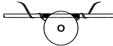
STEP 4: APPLY THE LEGS BY WRAPPING THEM AROUND THE CONDUCTOR. MAKE SURE TO SNAP THE LEG ENDS INTO PLACE TO COMPLETE THE APPLICATION. MAKE SURE THE TIE LOOP IS TIGHT ON THE INSULATOR NECK.
