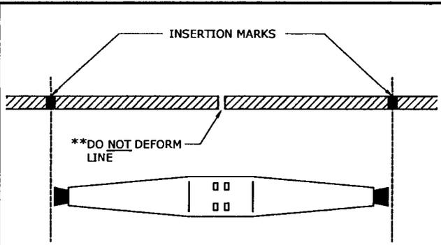
**\*\*WIRE BRUSH CONDUCTOR AND CONDUCTOR ENDS CLEAN, BRIGHT AND FREE FROM BURRS. SPLICE MUST ALSO BE CLEAN, FREE FROM DIRT AND JAWS FREE IN HOUSING. MEASURE AND MARK CONDUCTOR FOR INSERTION FROM KNURL TO END OF FUNNEL GUIDE. MARK WITH TAPE OR MARKER.**
