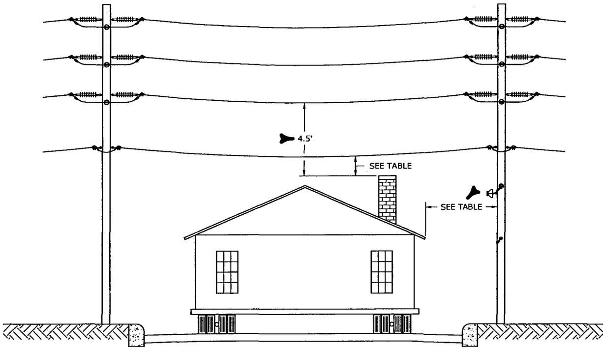
THE CLEARANCE OF A BUILDING BEING TRANSPORTED UNDER DISTRIBUTION LINES IS TREATED THE SAME AS A MOVING VEHICLE PER THE NESC UNIFORM SYSTEM OF CLEARANCES. THE VERTICAL CLEARANCE ABOVE GROUND CONSISTS OF A REFERENCE COMPONENT WHICH IN THIS CASE WOULD BE THE HEIGHT OF THE BUILDING ON THE TRANSPORT VEHICLE, PLUS A MECHANICAL AND ELECTRICAL COMPONENT AS FOLLOWS:
