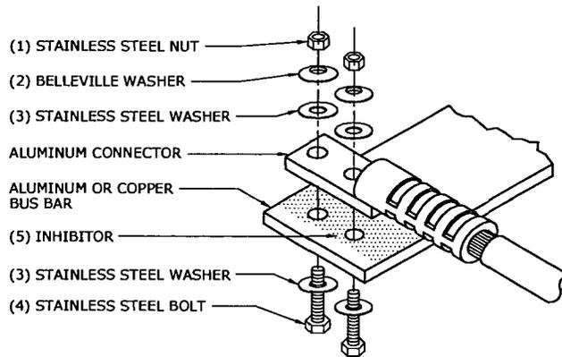
SWITCH CONNECTION DETAIL TORQUE TO 40 FT. LBS.
