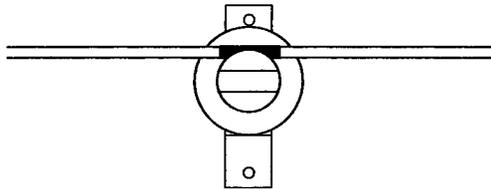
STEP 1: APPLY TIE PAD ON TO CONDUCTOR, SLIT FACING UP SO THAT CONDUCTOR DOES NOT COME INTO DIRECT CONTACT WITH THE INSULATOR.
