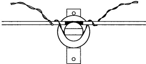
STEP 3: PLACE THE EZ-WRAP SIDE TIE IN POSITION AND START WRAPPING THE LEGS. NOTICE ONE LEG GOES OVER THE CONDUCTOR WHILE THE OTHER GOES UNDER THE CONDUCTOR.
