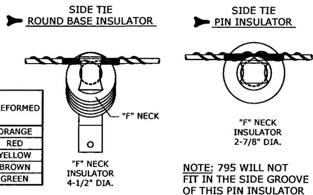
NOTE: 795 WILL NOT FIT IN THE SIDE GROOVE OF THIS PIN INSULATOR
