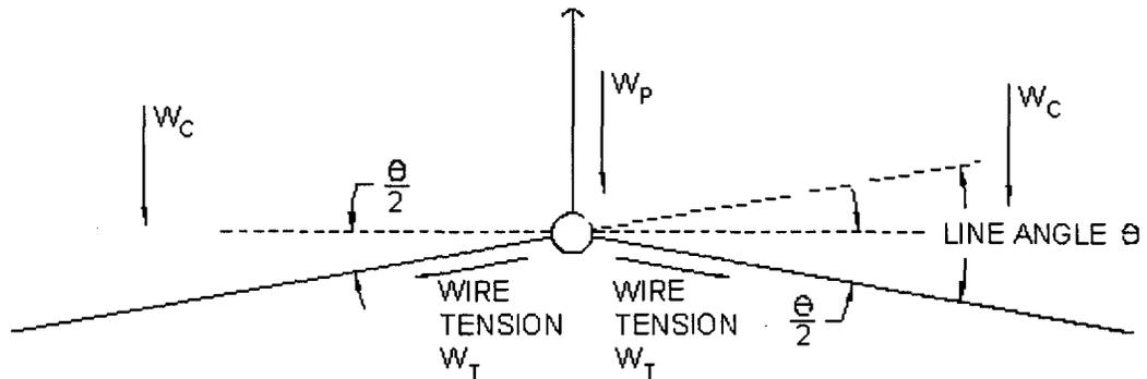
$$W_T = \text{WIRE TENSION FORCE} = 2 \times \text{TENSION PER CONDUCTOR} \times \sin \frac{\theta}{2}$$
