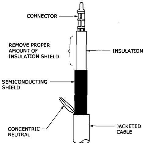
CAREFULLY REMOVE THE PROPER AMOUNT OF INSULATION SHIELD USING A SEMICON STRIPPER. STRIP LENGTHS CAN VARY BY ELBOW. USE THE INSTRUCTION SHEET THAT CAME WITH THE ELBOW. DO NOT NICK OR SCORE INSULATION.
