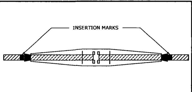
**INSERT CONDUCTORS TO FULL DEPTH: PUSH SLOWLY AND DO NOT TWIST. NEXT, PULL CONDUCTORS TO MAKE SURE JAWS FIRMLY GRIP. CHECK INITIAL GRIP WITH MOMENTARY PULL ON CONDUCTOR PRIOR TO APPLYING LINE TENSION.**
