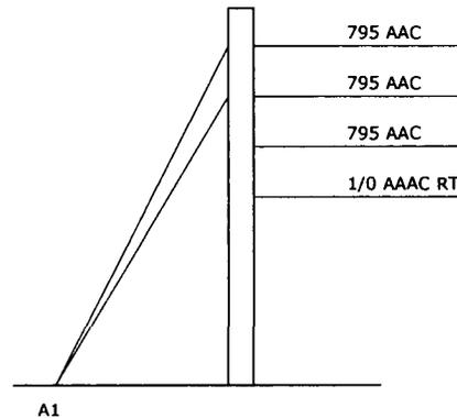
THE REQUIRED ANCHOR (A1) TO SUPPORT BOTH GUY WIRES IN CLASS 5 SOIL IS 2 HELIX ANCHOR, WHICH IS
