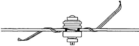
STEP 3: APPLY THE LEGS BY WRAPPING THEM AROUND THE CONDUCTOR. MAKE SURE TO SNAP THE LEG ENDS INTO PLACE TO COMPLETE THE APPLICATION. MAKE SURE THE TIE LOOP IS TIGHT ON THE INSULATOR NECK.
