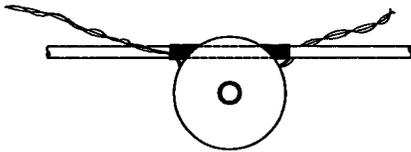
STEP 3: PLACE THE LOOP TIGHTLY UP AGAINST THE INSULATOR'S GROOVE AND POSITION THE TIE LEGS, AS SHOWN, SO THEY CAN BE APPLIED TO THE CONDUCTOR.
