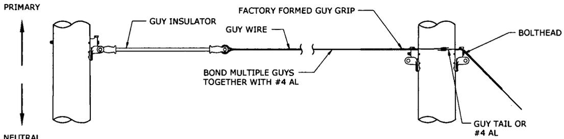
▶ IF A SPAN GUY IS RAN TO THE PRIMARY POLE NEUTRAL POSITION, IT SHOULD BE BONDED TO SYSTEM NEUTRAL.
