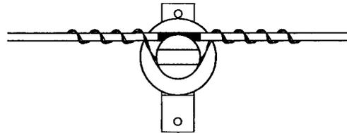
STEP 4: WRAP BOTH LEGS COMPLETELY, SNAPPING THE ENDS IN PLACE WITH THUMB PRESSURE. MAKE SURE THE TIE LOOP IS TIGHT ON INSULATOR NECK AND UNDER INSULATOR HEAD.
