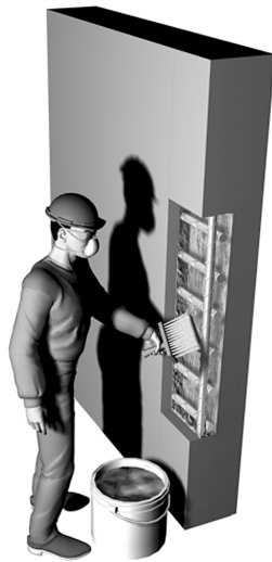
Fig. 6—Treatment of exposed reinforcement.
