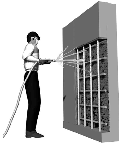
Fig. 3—Presaturate prepared surface with water.
