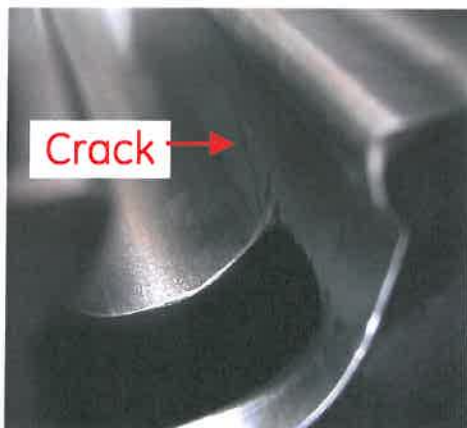
Figure 2: Example of Turbine Wheel Crack
