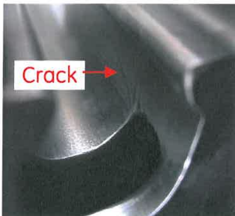
Figure 2: Example of Turbine Wheel Crack
