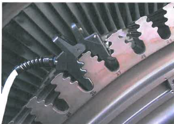
Figure 5: Eddy Current Inspection
