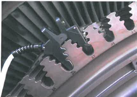
Figure 5: Eddy Current Inspection
