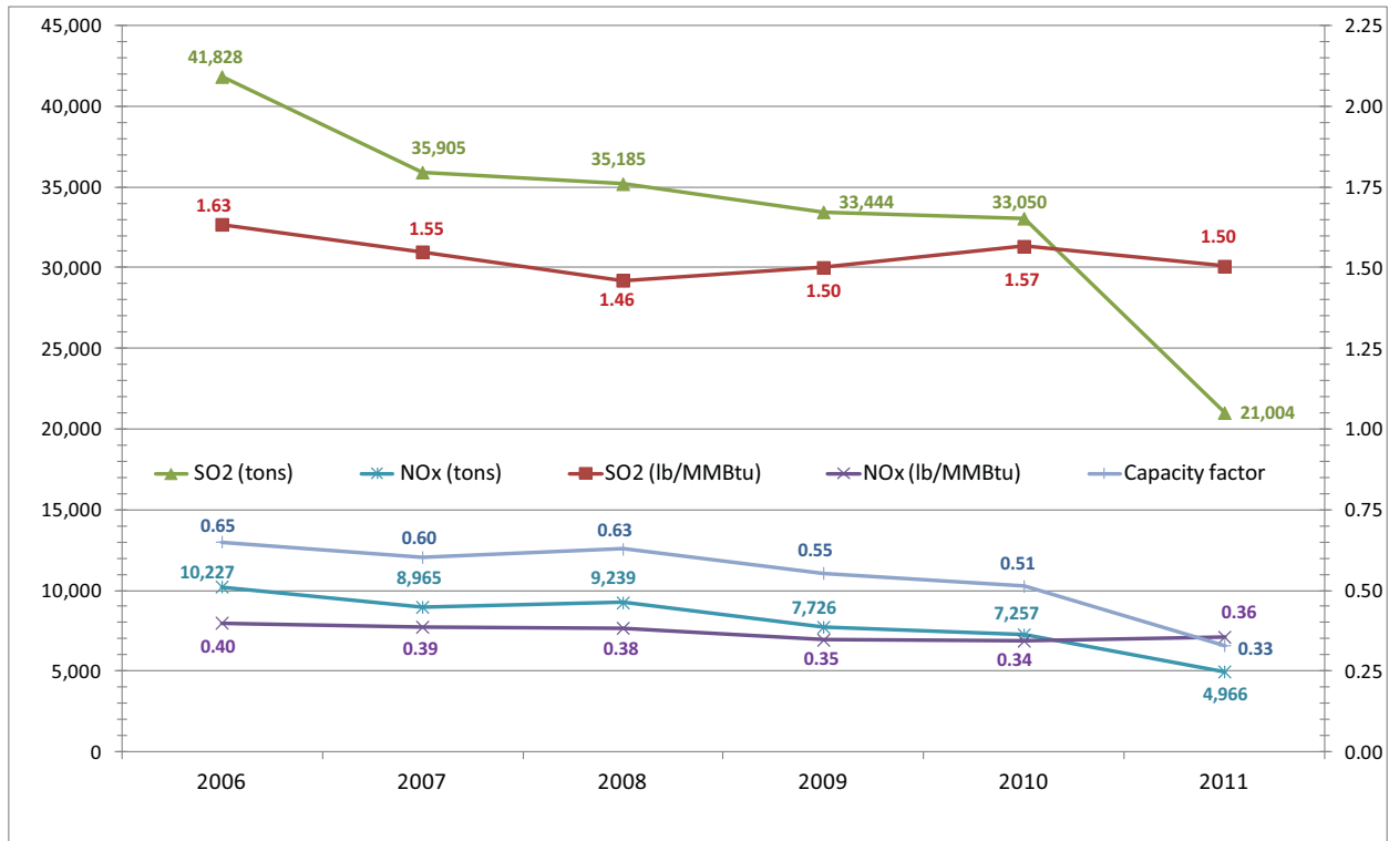
Figure 5. Combined Units 1 and 2 NO x , SO 2 Emissions and Gross Generation Capacity Factors
