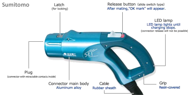
Figure 24 - Sumitomo CHAdeMO Connector
