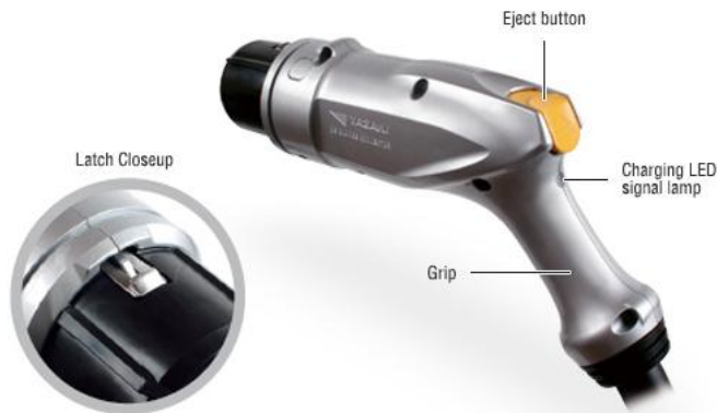
Figure 27 – Yazaki Gen 2 CHAdeMO Connector
