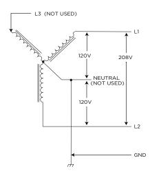
CAUTION: The unused leg (L3 in the illustration) must remain open. Do not connect to a neutral bar, or to ground.
