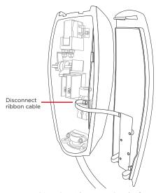
CAUTION: When removing the front cover, do not damage the ribbon cable. Disconnect the ribbon cable before fully releasing the front cover.
