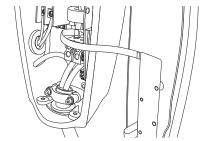
3 Hang the front cover over the hinge located at the top of the connector. Do not secure the front cover yet.
