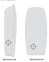
NOTE: Use the back knock-out when mounting to a pedestal or when running wires from behind a wall.
