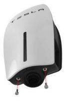
Release the front cover by pulling it towards you far enough to disconnect the ribbon cable. Disconnect the ribbon cable from inside the main enclosure to fully release the front cover.
