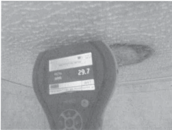
Photo 17. Elevated moisture levels around a water and possible fungal stained area in the ceiling of the women's restroom
