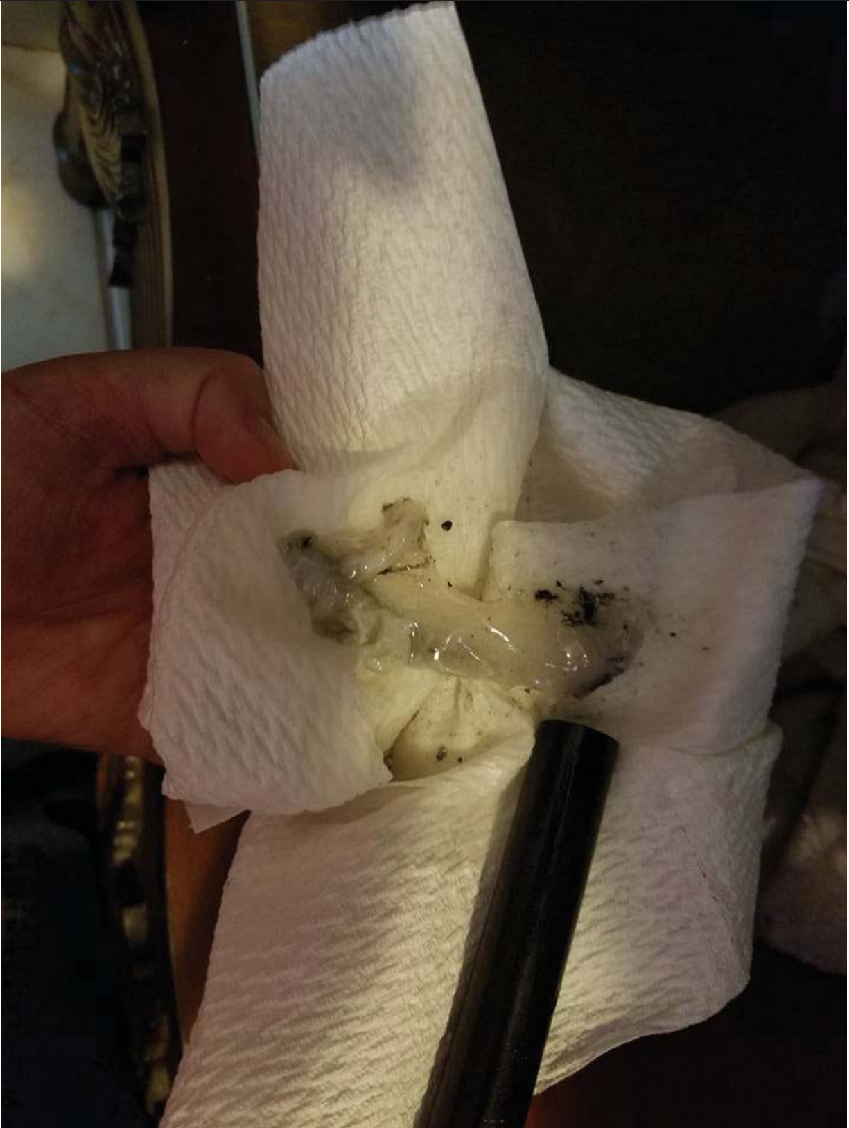
Photo 6 - Algae buildup in water line and drain.
