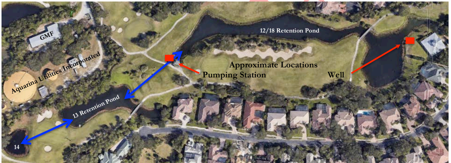
Figure-1 shows the installation showing the Pumping Station, Well and Pond interconnections. The Irrigation System tie-in is due left of the Pumping Station near the trees by AUI. Admin Building is at upper right.
