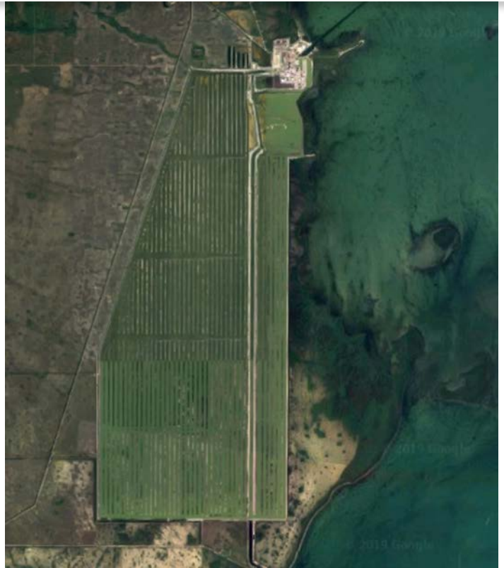
A 2019 Google Earth image of the cooling canals at Turkey Point that are used to cool two nuclear reactors and a gas-powered plant and also hold wastewater from the plant site.
