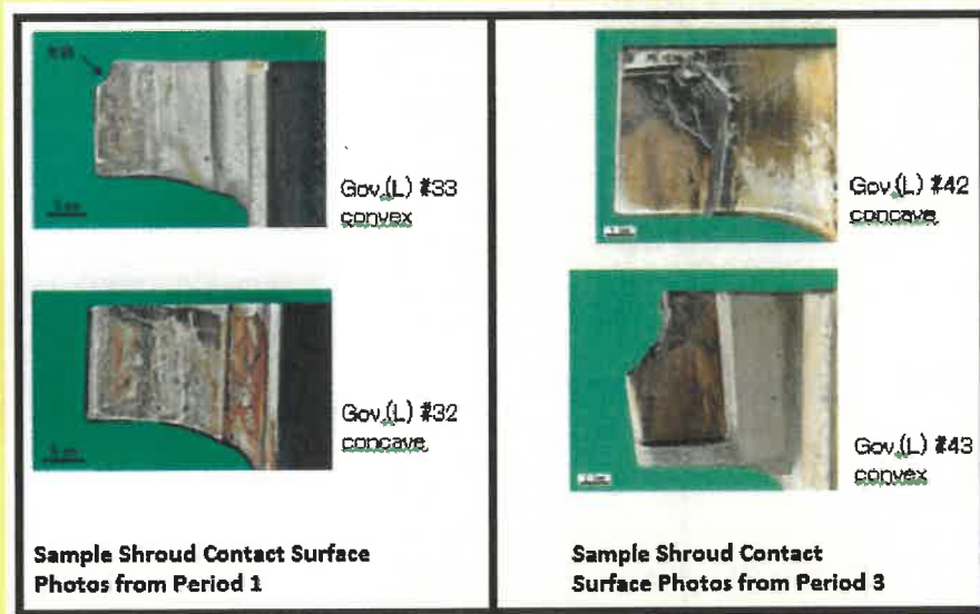
Figure 1 -- Comparative Photos of Shroud Contact Surface Wear for Periods 1 and 3
