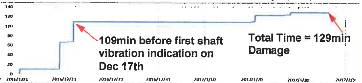
Period 5 – D Bypass Accumulated Time – Stub Damage (Gen)
