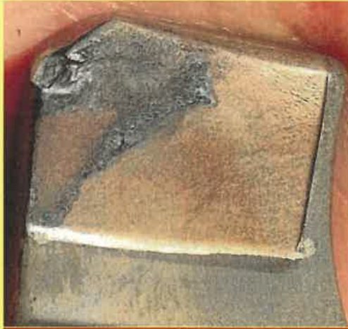
Figure XX: Photo of Z-notch from Period 5 showing wear of contact surface
