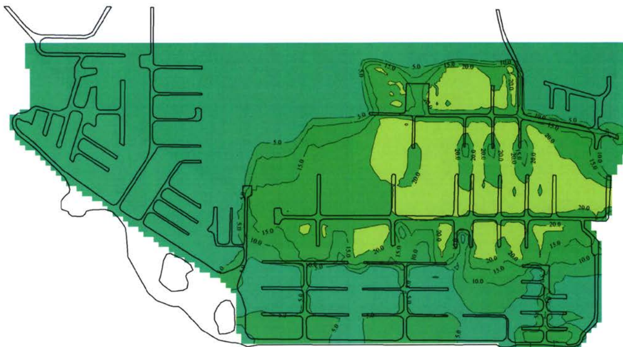
Fig. 8 Nitrate plume concentrations (mg/L) at nearly 40 years of elapsed simulation time prior to sewer conversion
