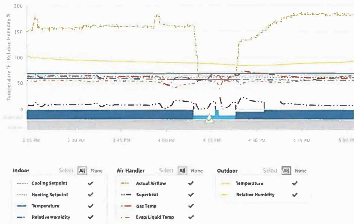
Figure 3-1 Operational status of a variable capacity heat pump from the manufacturer diagnostics portal. Note the 15-minute DR event triggered at 4:08PM.
