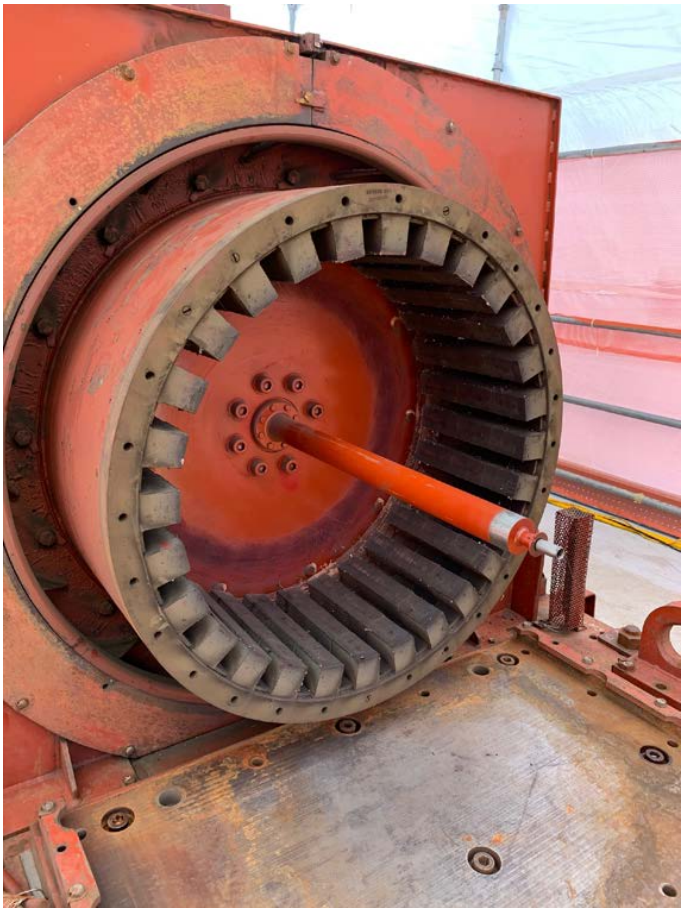
Fig. 8 PMG Pole Support w/ Magnets
