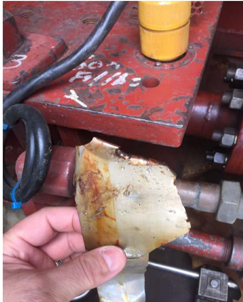
Fig. 12 Liberated Shim Stock Found in AC Exciter Section
