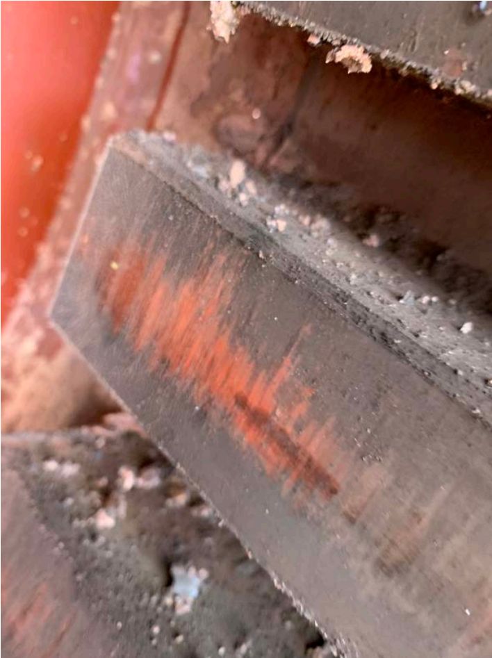
Fig. 9 PMG Magnet Rub
