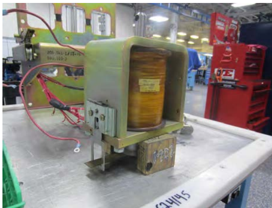
Closing Solenoid Assembly
