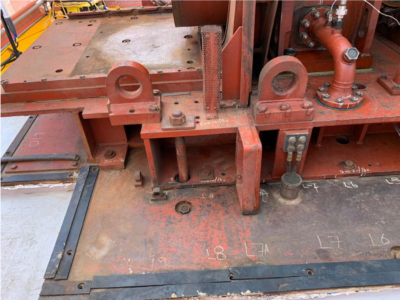
Fig. 13 Exciter Base to Housing Seal / Gasket Arrangement
