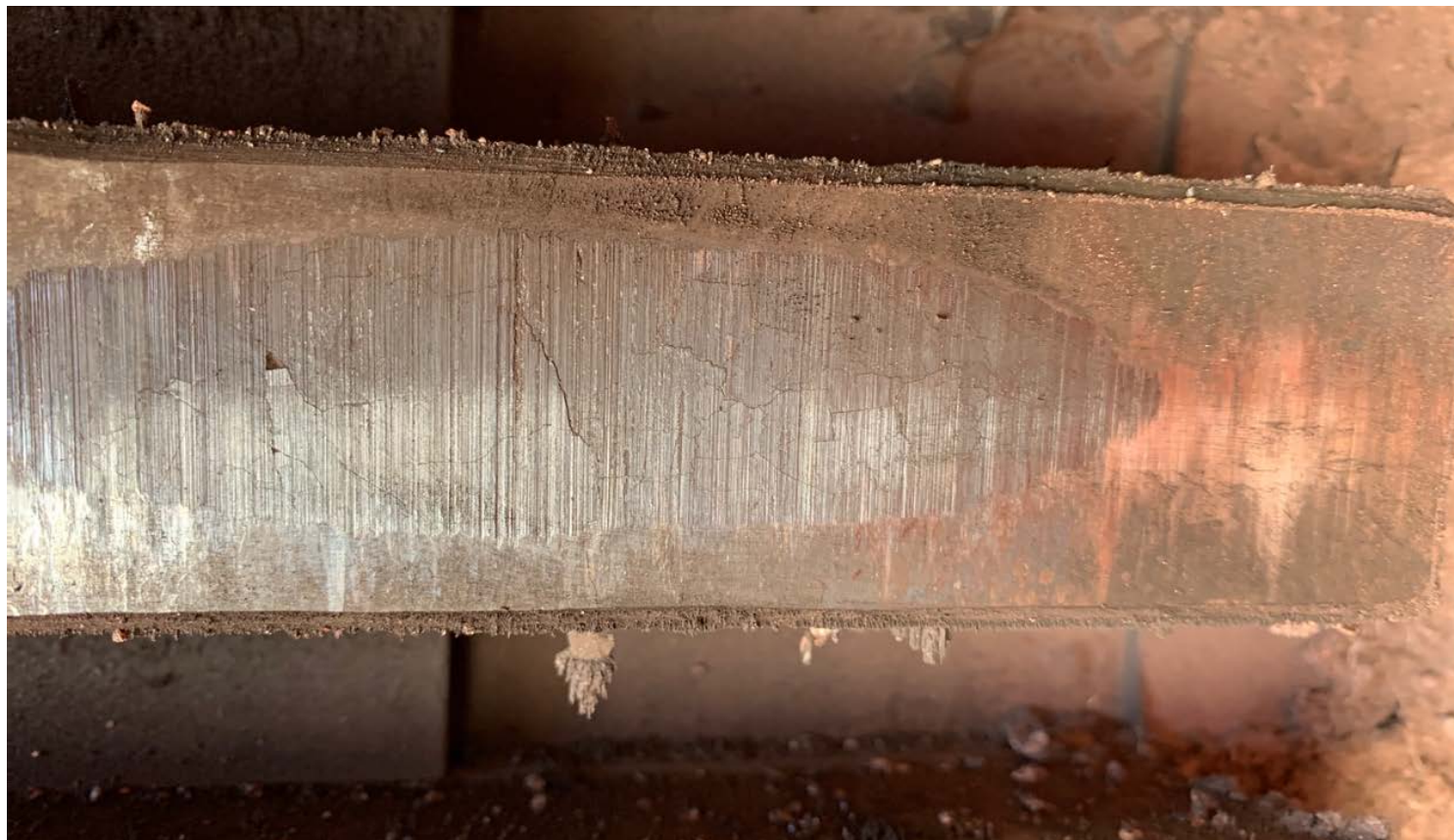
Fig. 10 PMG Magnet Cracking
