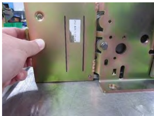
Operating Mechanism Inspection Hole
