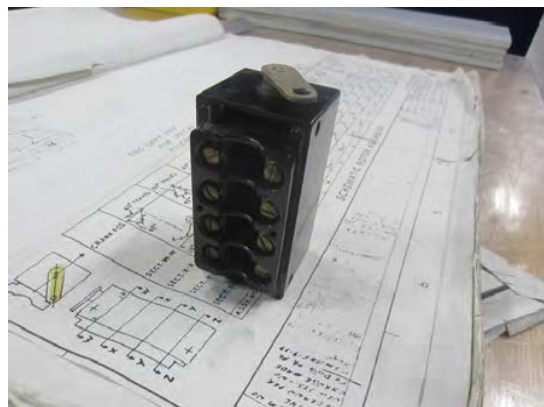
Switch Contact Verification
