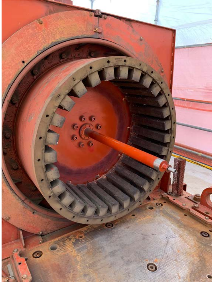
Fig. 8 PMG Pole Support w/ Magnets
