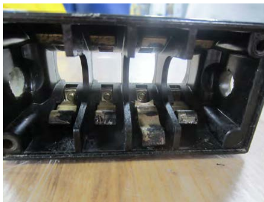
Right-Side Switch Stationary Contacts
