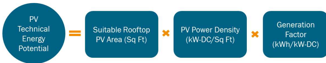
Equation 3: Core Equation for Solar DSRE Technical Energy Potential
