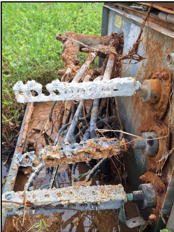
Figure 1: Underground construction with severe corrosion and electrolysis due to storm surge during Hurricane Helene
