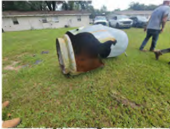
Tank failure and damage to site caused by explosion - Oakcrest Villas system
